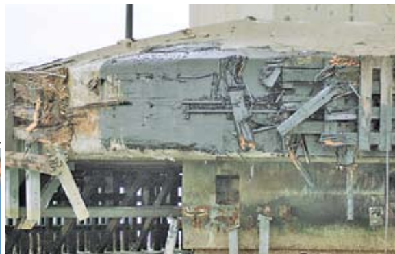
Spread, the 'Cosco Busan' displays her wounds. Above, the Bay Bridge's concrete abutment acted like a giant can opener on the ship. Note the oily 'arterial spray' from the accident.
