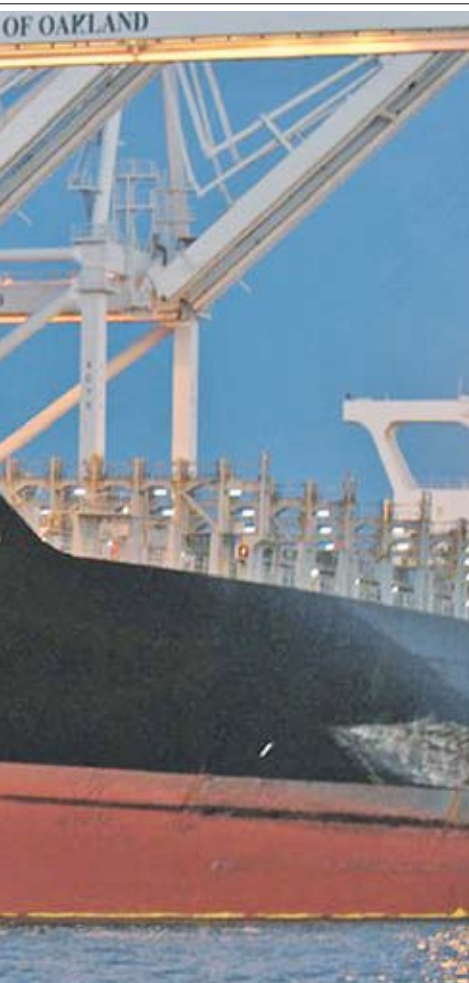
Spread, the 'Cosco Busan' displays her wounds. Above, the Bay Bridge's concrete abutment acted like a giant can opener on the ship. Note the oily 'arterial spray' from the accident.
