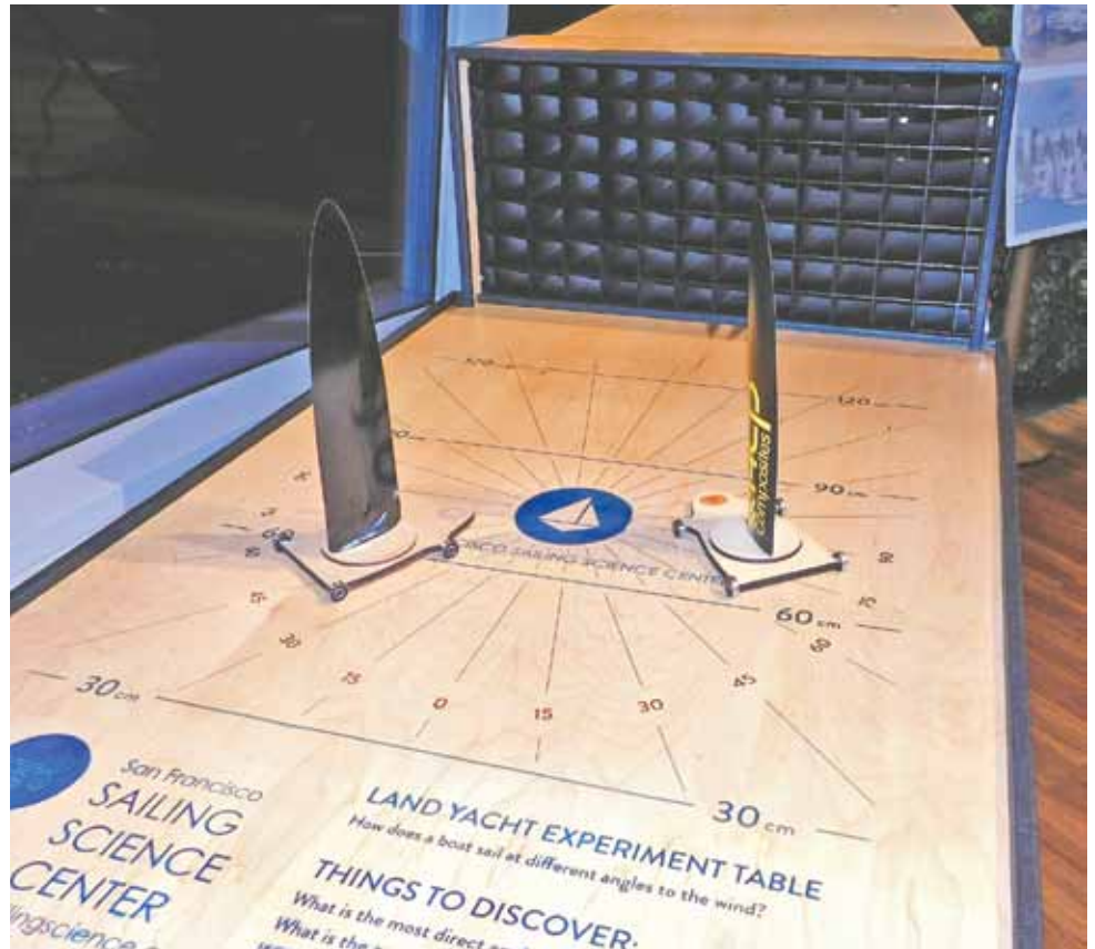
The Land Yacht Experiment Table. Perfect for skeptics who need to be convinced that yes, a sailboat really can sail into the wind. Adjusted carefully, these models can point within 30 degrees of the true wind direction.
