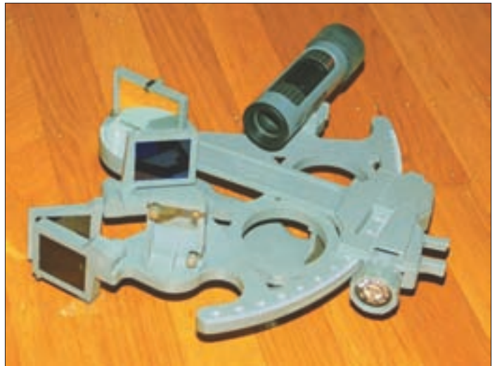
The upgraded Mark 25. The full-field beam converger mirror is replaced with the more conventional split mirror.
