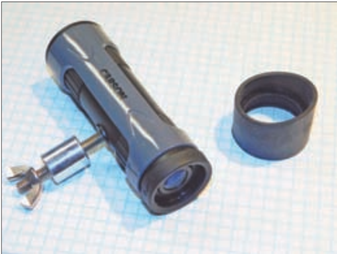
You'll need a few inches of \frac{1}{4} " x 20 threaded rod, a \frac{1}{4} " wing nut and a spacer or large fender washer.
