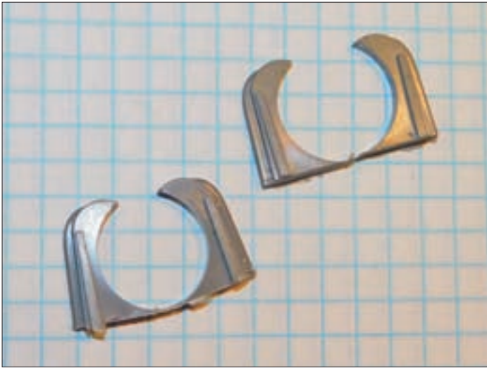
Cut off the clips that hold the standard plastic telescope.
