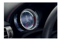
TEXT BY SHOGO HAGIWARA PHOTOGRAPHY BY GREG WHITE Inspired by the design of the Lexus LFA digital gauge, the Lexus IS's F SPORT meter is formed of an eight-inch thin film transistor liquid-crystal display (TFT-LCD), framed by a ring-shaped element mounted on the screen. well put together." This measures about 120 millimeters in diameter and sits at the center of the monitor, with the digital elements of the gauges
