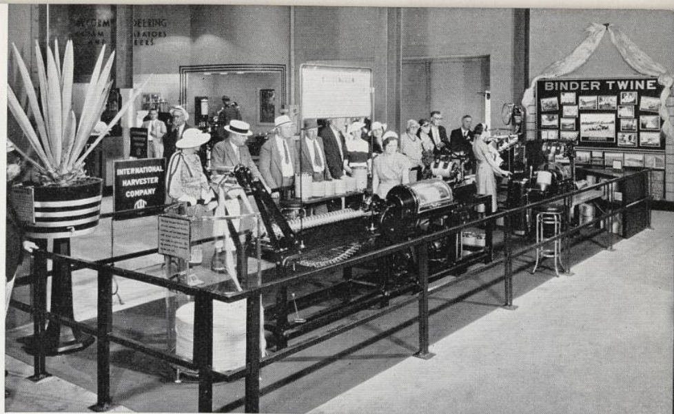
Spinning and halling McCormick-Deering Binder Twine, as demonstrated at A Century of Progress. The spinner, baller, covering machine, and testing machine are attended by regular employees of McCormick Twine Mill in Chicago. Binding mechanism of a modern grain binder at the far end of the exhibit shows how the knot is tied. Seventeen colored transparency pictures on the wall show the process of binder twine manufacture from the young sisal plants on the International Harvester sisal plantation in Cuba to the finished product. Colored photographs of the six International Harvester twine mills are shown below the transparencies. Pillars of twine balls and samples of the fiber are at each side of the pictures.
