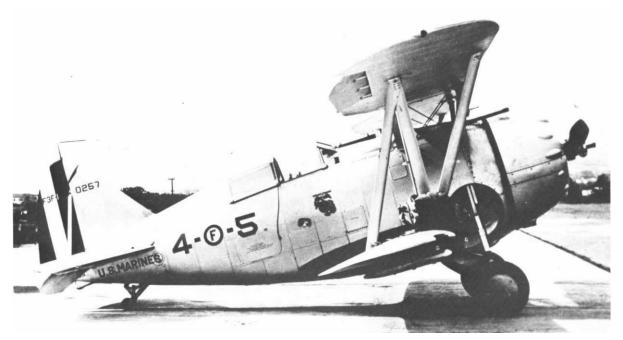
An F3F-1 of VF-4M. This was the first Marine fighter with retractable landing gear. (Photo from Museums Branch Activities, Quantico).
