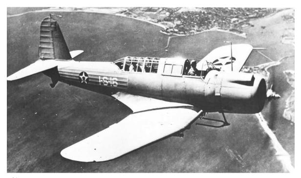
SB2U-3 in flight. This aircraft was classed as a scout bomber and could take off from carriers or be launched from a ship's catapult. (Marine Corps Photo 306304).
