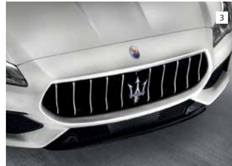
3 - Chromed front grille, front sport bumpers with Black Piano finishing, blue inserts on Trident.
