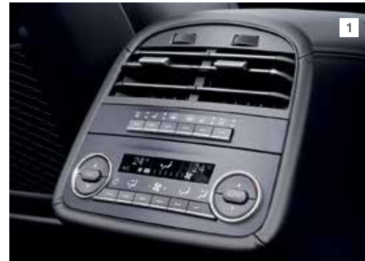
1 - Four zone air conditioning.
