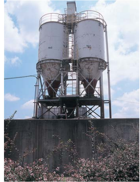
Humidifying system for using casting sand in cement manufacture.
