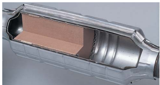
Internal structure of the new three-way catalyst
