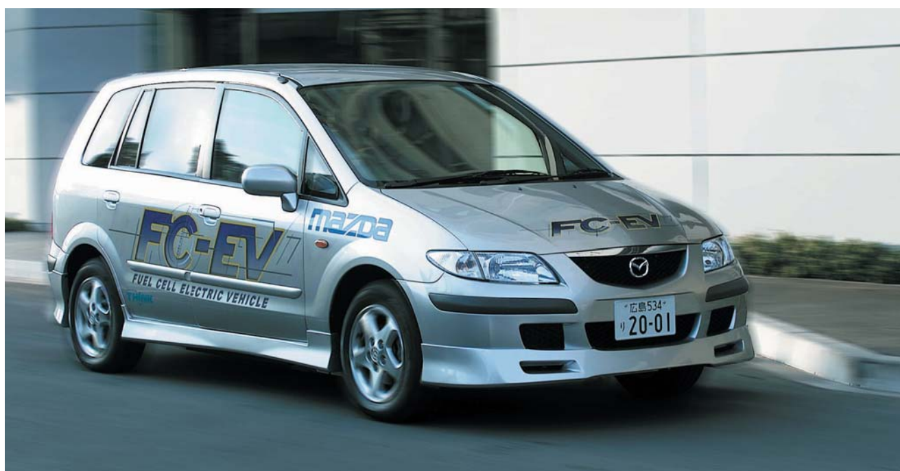
Premacy FC-EV (methanol-reforming fuel cell powered vehicle)
