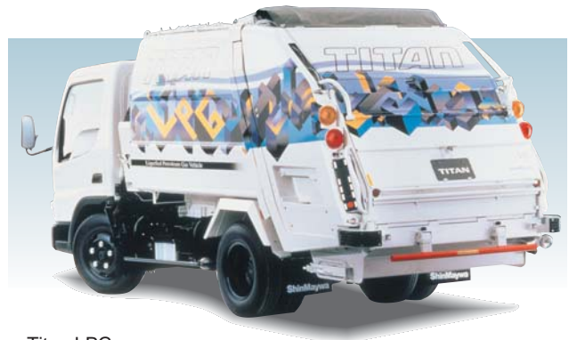
Titan LPG Refuse collection vehicle fitted with odor eliminating equipment
