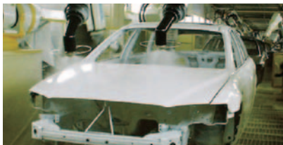
Three-Layer Wet Paint System
