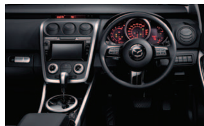
Adhesive-free instrument panel achieved through integrated construction of components and covering
