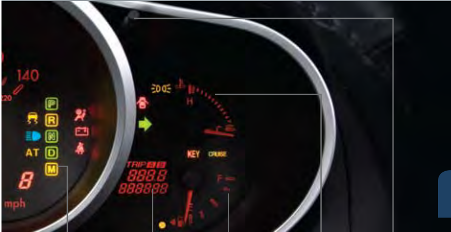
GEAR INDICATOR ODOMETER/ TRIP METER FUEL GAUGE ENGINE COOLANT TEMPERATURE GAUGE ODOMETER/TRIP METER SELECTOR
