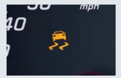
LOAD-ADAPTIVE ELECTRONIC STABILITY **PROGRAM (ESP®)**<sup>8</sup> This dynamic handling system actively intervenes to help keep the van firmly under control and safe by automatically braking individual wheels, and reducing engine power to help stabilize the vehicle if wheelspin, understeer, or oversteer is detected.
