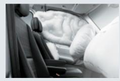
DRIVER AND PASSENGER AIRBAGS<sup>9</sup> The driver and passenger front, thorax, and window airbags<sup>9</sup> help protect you and your passengers in the event of a collision. Sprinter airbags shown are from Model Year 2014.
