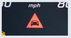
ACTIVE BRAKE ASSIST<sup>1</sup> This advanced system senses the likelihood of a collision with a vehicle ahead and sends both a visual and audible warning, and autonomous braking can be initiated.
