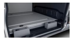
Pallet bracing and tie-downs help when hauling cargo with unusual sizes and shapes<sup>25</sup>
