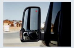
BLIND SPOT ASSIST<sup>3</sup> has Rear Cross-Traffic Alert<sup>4</sup>, which employs automatic braking to avoid a collision with traffic crossing the vehicle's path (e.g., vehicles or pedestrians) when reversing.
