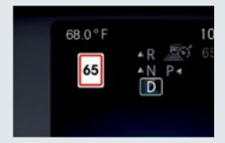
**TRAFFIC SIGN ASSIST<sup>30</sup>** uses a camera to give drivers additional help with identifying speed restriction signs, No Passing zones, and No Entry signs.
