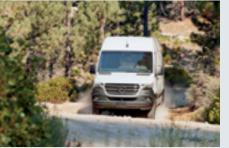
HILL-START ASSIST briefly stops the vehicle from rolling backward or forward, giving you an extra level of safety and confidence when making a hill start. Hill-Start Assist maintains brake pressure for approximately two seconds, so you can remove your foot from the brake pedal without rolling.
