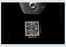
With **RESCUE ASSIST**,<sup>™</sup> first responders to an accident can scan a QR code in a Mercedes-Benz Van to quickly see where batteries, airbags, and other structural elements are located in order to safely perform the rescue.
