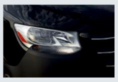
HIGHBEAM ASSIST<sup>SM</sup> adjusts the highand low-beam headlamps automatically, allowing for continuous adaptation to the prevailing traffic situation. The system helps ensure better and earlier recognition of the course of the road.
