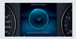
ATTENTION ASSIST®<sup>2</sup> helps prevent drowsy driving by monitoring your driving patterns and providing an early warning in case fatigue is detected.
