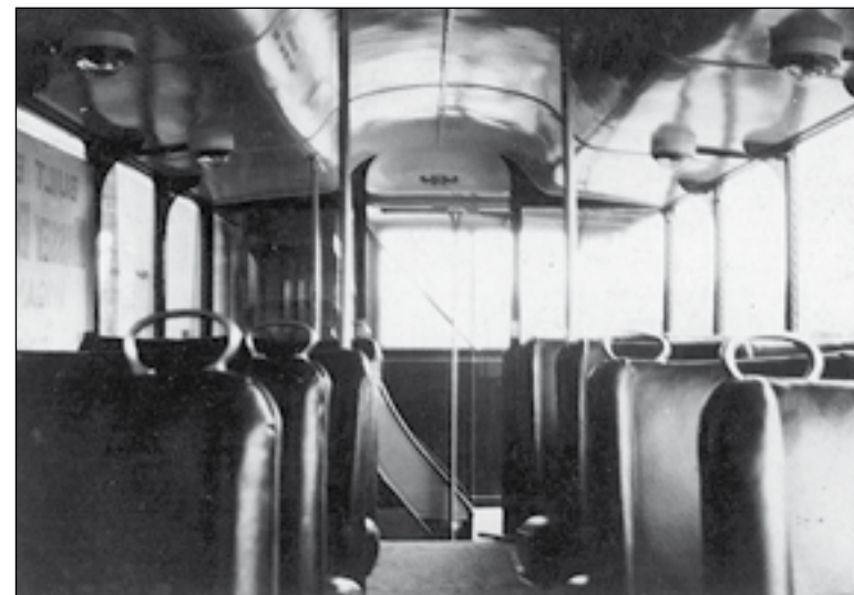
Left: The patented Leyland Motors side gangway layout, designed by GJ Rackham, which reduced the height of the lowbridge Titan TDI to 12ft 10in and revolutionised the double-decker market. Competitors were obliged to use alternative layouts, as above with Cumberland's Guy, or, later, pay Leyland a royalty for use of the design. (STA)
