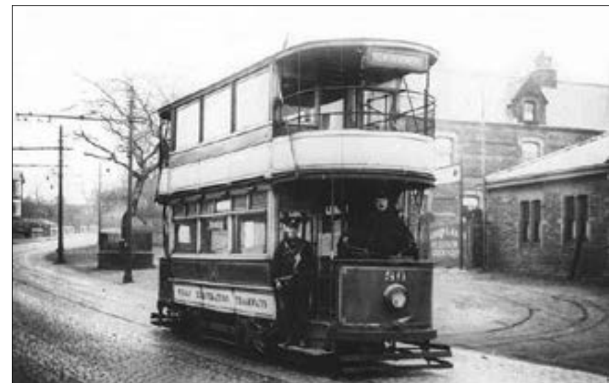
Wigan Corporation 62-seat tram No. 90 at the Abbey Lakes terminus shortly before the abandonment of the tramway system in 1931 which brought more Leyland Titans – but now with Massey bodies – into the fleet. Massey also built the bodies on these trams which, as described in the text, were then fitted to English Electric equipment. Note the method of securing the top deck cover to the canopy bend above the conductor's head.
