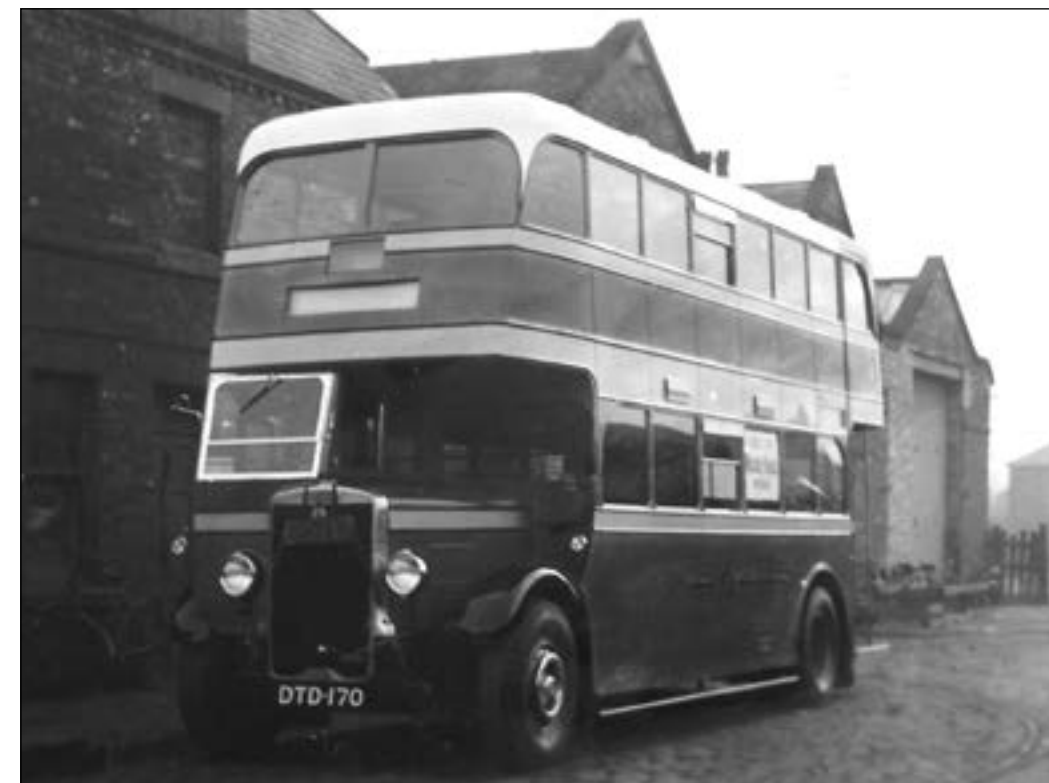
Showing its rear entrance body to good effect is this Leyland Tiger TS8c which was one of two with Massey bodies supplied to Bolton Corporation in the late summer of 1938. There were two more similar vehicles supplied at the same time but with dual-purpose bodies by Park Royal. (STA)
