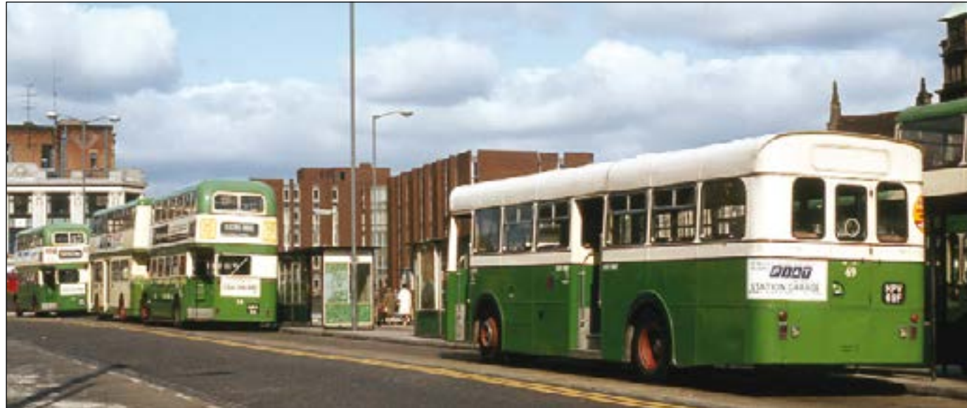
This shows the rear nearside of Ipswich Corporation AEC Reliance No. 69 showing the unusual dual door layout with centre exit, which these buses introduced to the town, and are still evident on several buses remaining from the 1990s. The doors were not necessarily popular with maintenance staff but this door layout was perpetuated on all full sized buses, saloons and double-deckers purchased until the mid 1990s. The bus appears to be on layover with two East Lancs Regents, and a Roe Atlantean sometime in 1980. (OP)
