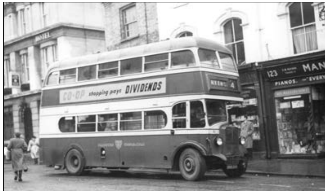
Burnley, Colne and Nelson's No. 152, (HG 6013), a Leyland Titan TD5c dating from December 1937, was seen standing in a light covering of snow at their Nelson depot shortly after delivery and showing the body styling before the introduction of the curved front to the upper deck. The logo, incorporating the coats of arms of the three authorities, was one of the most distinctive of the municipal embellishments carried by any public service vehicle. (JL)
