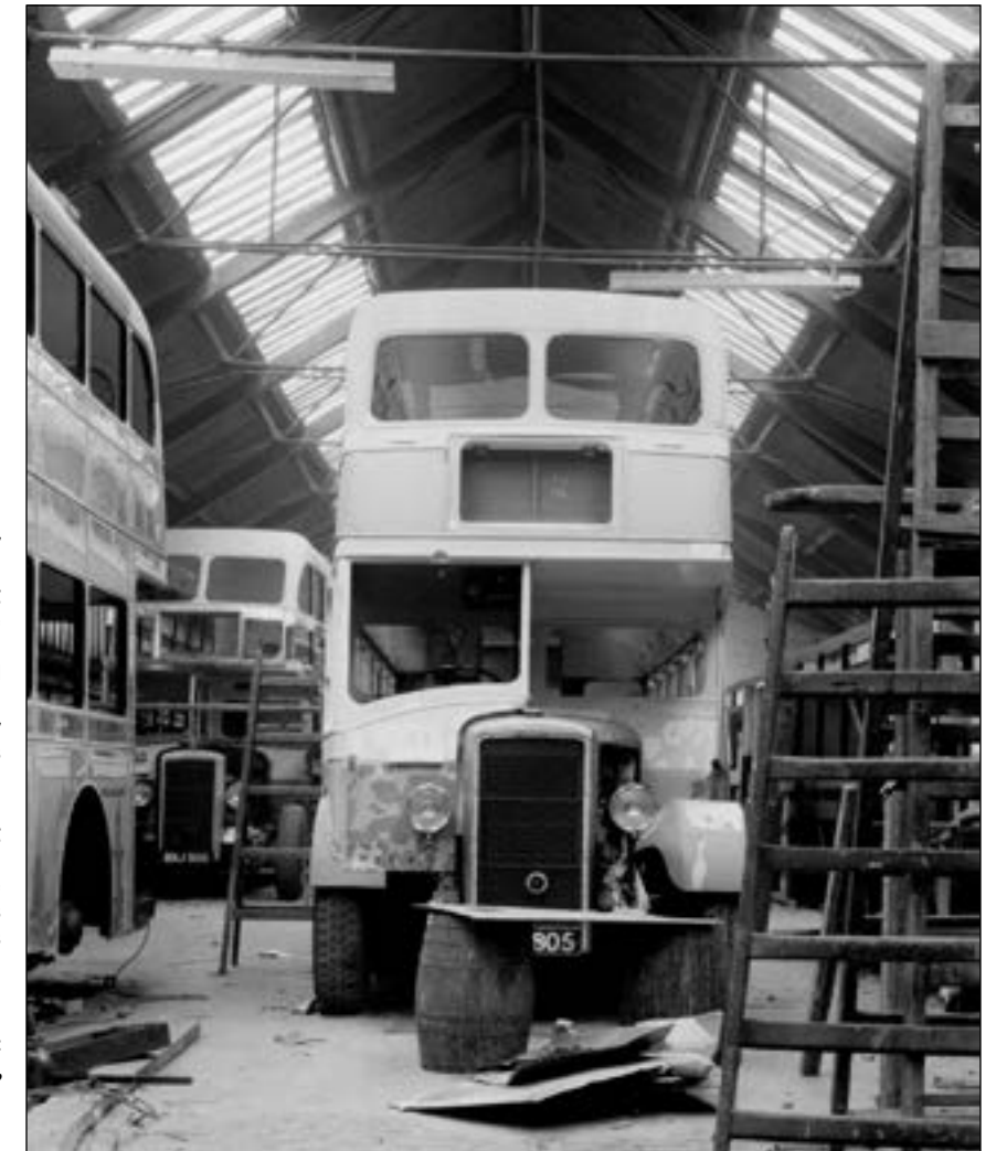
Southend Corporation's wartime lowbridge Daimler CWA6's were worked hard, and six were rebodied by Massey in 1952. This is No. 231, BHJ 805, nearing completion in the Massey bodyshop. This was one of a batch of six to be rebodied (sister vehicle 806 is visible behind) and this particular vehicle had clocked up 691,596 miles when finally withdrawn in 1965, a testimony to the rugged wartime Daimler chassis. Note that Southend have had the radiators chromium plated to enhance the appearance, in keeping with the rest of its very smart fleet.
