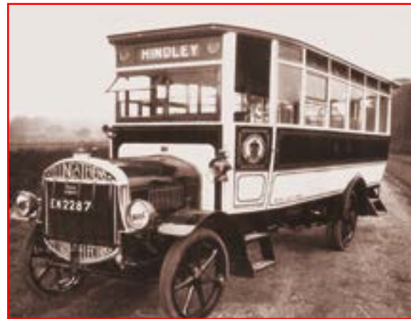
Wigan Corporation's Tilling-Stevens petrol-electric chassis were fitted with dual-doorway bodies as seen here, but had short lives as noted in the text. The half-open rear was quite common at the time, being favoured by several bodybuilders. Note the high floor, requiring steps for access, due to the straight-framed chassis – a normal feature until cranked chassis were introduced later in the 1920s.
