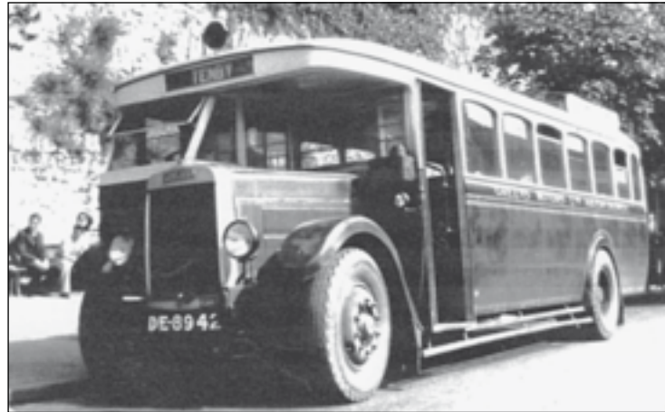
This Leyland Lion LT5, (DE 8942), with 31-seat Leyland-style body, complete with arched windows, entered service in July 1932 with Greens Motors Ltd of Haverfordwest and is seen parked in Tenby in the late 'thirties. Although the chassis specification had been upgraded the old-fashioned frontal arrangement with short radiator made the vehicle seem quite dated. Note the roof-mounted luggage carrier and marker light above the indicator.
