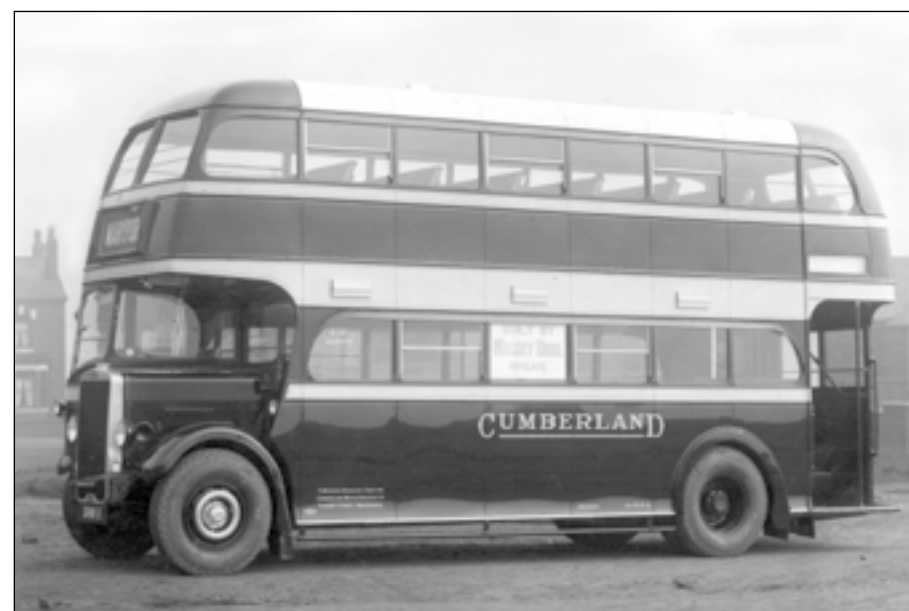
These photographs show the evolving Massey body curvature. The top image shows Cumberland Motor Services No. 135 (DAO 50) a lowbridge Leyland Titan TD5 one of a batch of five such vehicles delivered in 1938 with a restrained but not unpleasing appearance.
