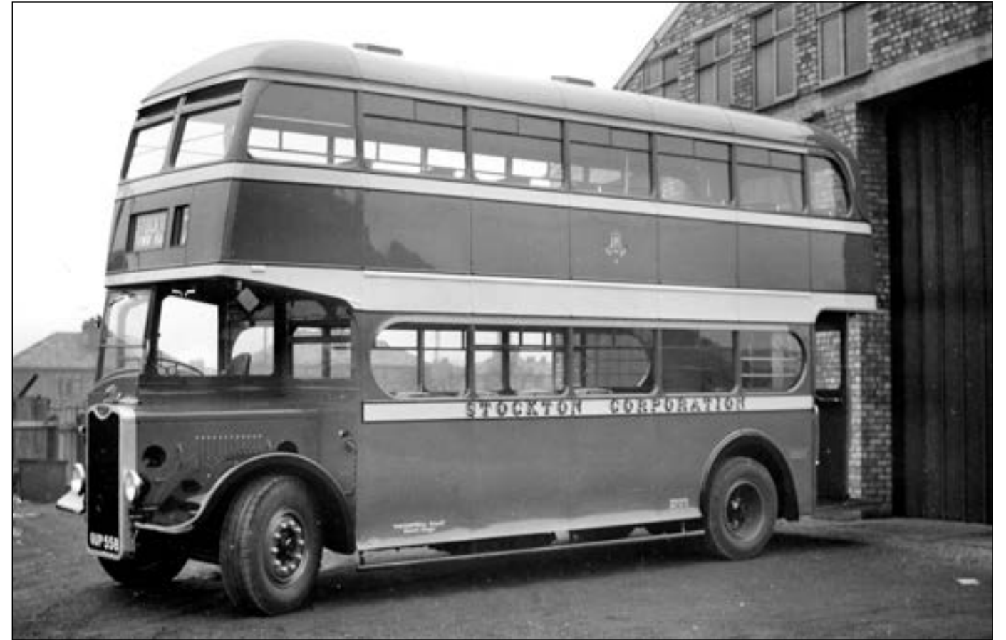
Stockton Corporation placed orders for Massey bodies on four different chassis makes during the immediate post-war period. This particular vehicle was one of eight supplied on Guy Arab chassis (two on Mk II and six on Mk III). Number 10, (GUP 558), a Mk III model, awaits departure from Enfield Street to the north east on a dull February day in 1947. The Massey body transfer is just visible.
