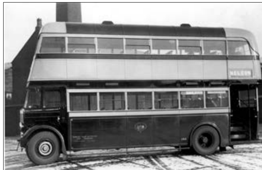
Burnley, Colne and Nelson's No. 152, (HG 6013), a Leyland Titan TD5c dating from December 1937, was seen standing in a light covering of snow at their Nelson depot shortly after delivery and showing the body styling before the introduction of the curved front to the upper deck. The logo, incorporating the coats of arms of the three authorities, was one of the most distinctive of the municipal embellishments carried by any public service vehicle. (JL)
