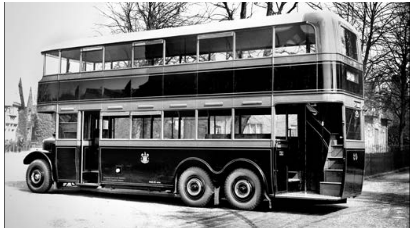
Warrington Corporation purchased two 30ft long AEC Renown chassis which were intended for London Transport. Massey Brothers supplied the 65-seat dual entrance/exit bodywork and No. 39 (ED 5880) is shown in the Warrington livery of Munich Lake (Maroon) and Citron (Yellow) at the corner of the A56, opposite the Walton Arms, in April 1930. The two vehicles remained in service until 1937, and whilst the design looks strange, even dangerous perhaps, it was no more so than the hundreds of tramcars then in use throughout the country with their equally restrictive layout as seen on page 30. Nevertheless, the front staircases were fairly soon removed, possibly following an inspection under the new 1931 Road Traffic Act. This was Massey's first order from Warrington; the operator took six Titan TD1s in 1931 but never patronised the Pemberton factory again. Had the body design been a step too far, closing the door on any future prospects? (STA)
