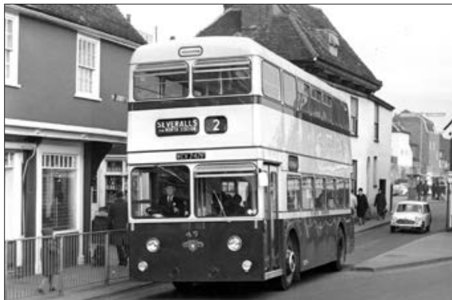
Number 47 in the Colchester fleet makes its way down St John's Street on the number 2 service from Ipswich Road to Severalls. It was one of ten Atlantean PDR1/1 models delivered to the operator in 1967/8. The box-line structure is a far cry from Massey's earlier well-rounded and much-loved designs.
