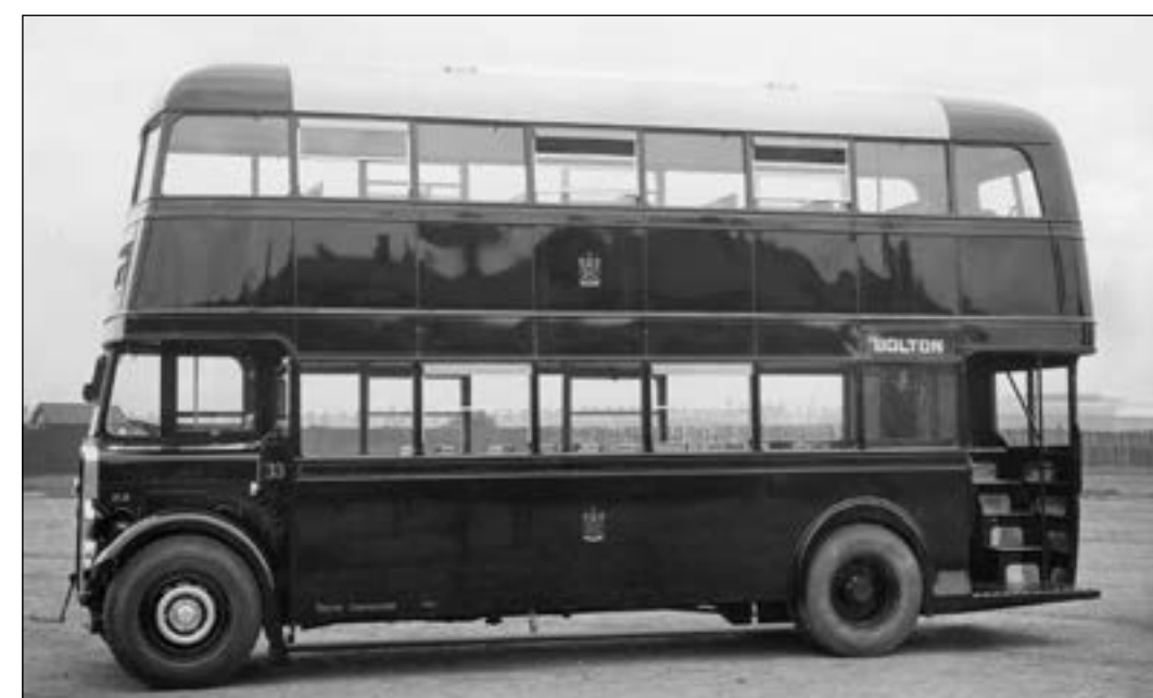
This almost broadside view clearly shows the sharp lines of the front upper-deck, combined with the more rounded rear. Bolton number 33 was also a TD4c with torque-converter transmission, this being popular with many operators replacing trams and making the transition easier from driving trams to driving buses. The deep housing on the front bulkhead (carrying the fleet number) is the combined Autovac and header tank for the fluid for the converter.
