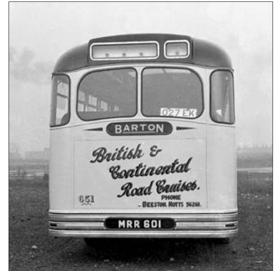
Barton Transport No. 651 was one of a number of rebuilds undertaken by this independent during the post-war period, and in this instance designated BTS1. The chassis on this vehicle was previously a Leyland PS1 from 1948 (No. 541) with a Duple body but it was rebuilt in 1951 with a new 30ft chassis frame and sent to Massey Bros. for a new dual-purpose body which was photographed in October 1951 prior to delivery. It was withdrawn in 1966 and sold to a church youth club. In June 1972 it became a mobile caravan, but in 1973 was back in service with Gosport Buses of Glasgow and was last seen in Ayr in 1979. Pictured below is the rear of 651 also taken when new at Pemberton. Despite the extent of the reconstruction it retained its original registration number throughout its life.
