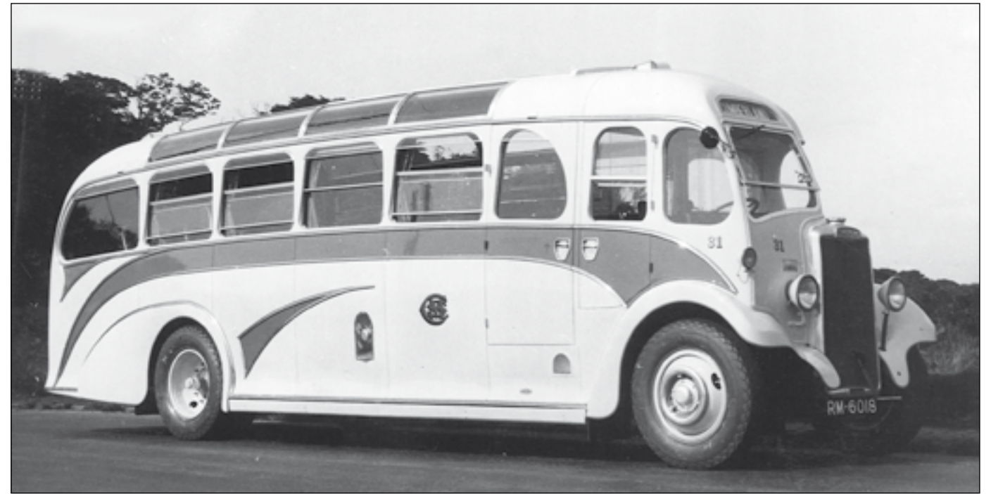
Cumberland No. 31 may have needed a Cov-Rad radiator conversion, and spats to cover the projecting dumb irons of its 1929 built chassis, but no one could fault the interior body appointments. Two-and-one deep leather-trimmed moquette seats with arm rests, radio speakers and a clock, glass cantrails for better visibility in the glorious Lake District, curtains to the deep half-drop windows and a discrete measure of chromium trim put this in a top quality league. Note the Massey Bros. gilt transfer on the bulkhead above the chrome fire extinguisher.
