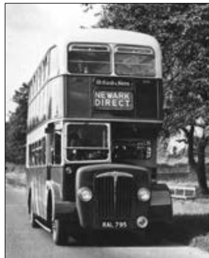
Numbered DD10 in the fleet of W Gash & Sons of Newark, Nottinghamshire, was this Daimler CVG6, seen before delivery in July 1954 and then soon afterwards in service. The Gash fleet, in two shades of green, was always well turned out and the rear platform doors and Daimler nearside mudguard arrangement help to produce an extremely handsome vehicle. (HSP left and below both)
