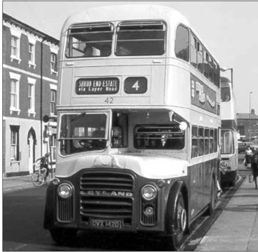
Colchester Corporation's number 42, one of a batch of six Leyland Titan PD2A/30s dating from 1966 and thus contemporary with the Maidstone Atlantean on the previous page. An unidentified example of Colchester's own Atlanteans is seen behind.
