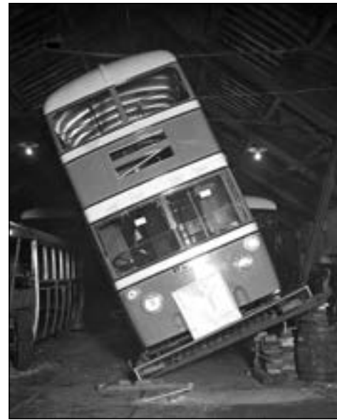
The Leyland Lowloader being tilt-tested at Massey's and then towed out of the Enfield Street works on its way to Leyland for checking out and official photographs, one of which is shown opposite.
