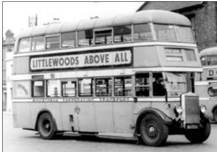
Birkenhead Corporation No. 219 was the first of a batch of 40 Leyland Titans delivered in 1937; this bus was the sole TD4c and the remainder were TD5c models. The seating for 54 was finished in blue leather which became standard Birkenhead practice from this point on. Three of the vehicles became air raid casualties but were rebodied/ repaired by Masseys in 1942. (HSPC)
