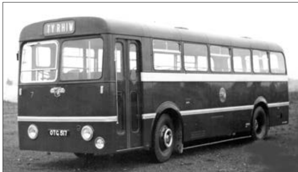
Caerphilly UDC purchased two Leyland Royal Tiger PSU1/13s in 1954, and shown here is No. 7 before delivery. Note the flat driver's windscreen compared to the Royal Tiger of Barrow Corporation in the adjacent illustration.
