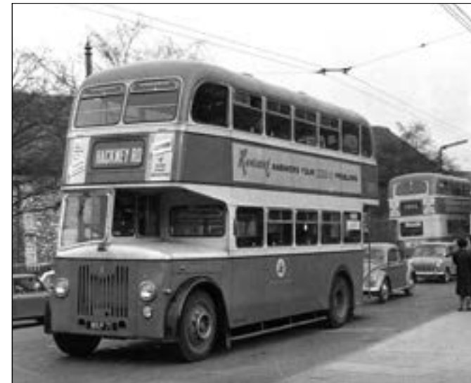
Below, left and right: Massey Brothers became firm favourites with Maidstone Corporation after the initial deliveries in 1956. These two photographs show number 1 (WKP 71) which was the first in a batch of six Leyland Titan PD2/20s noteworthy for having the revised front which did away with the traditional radiator, as also seen on the Yarmouth and Southend vehicles on this page.
