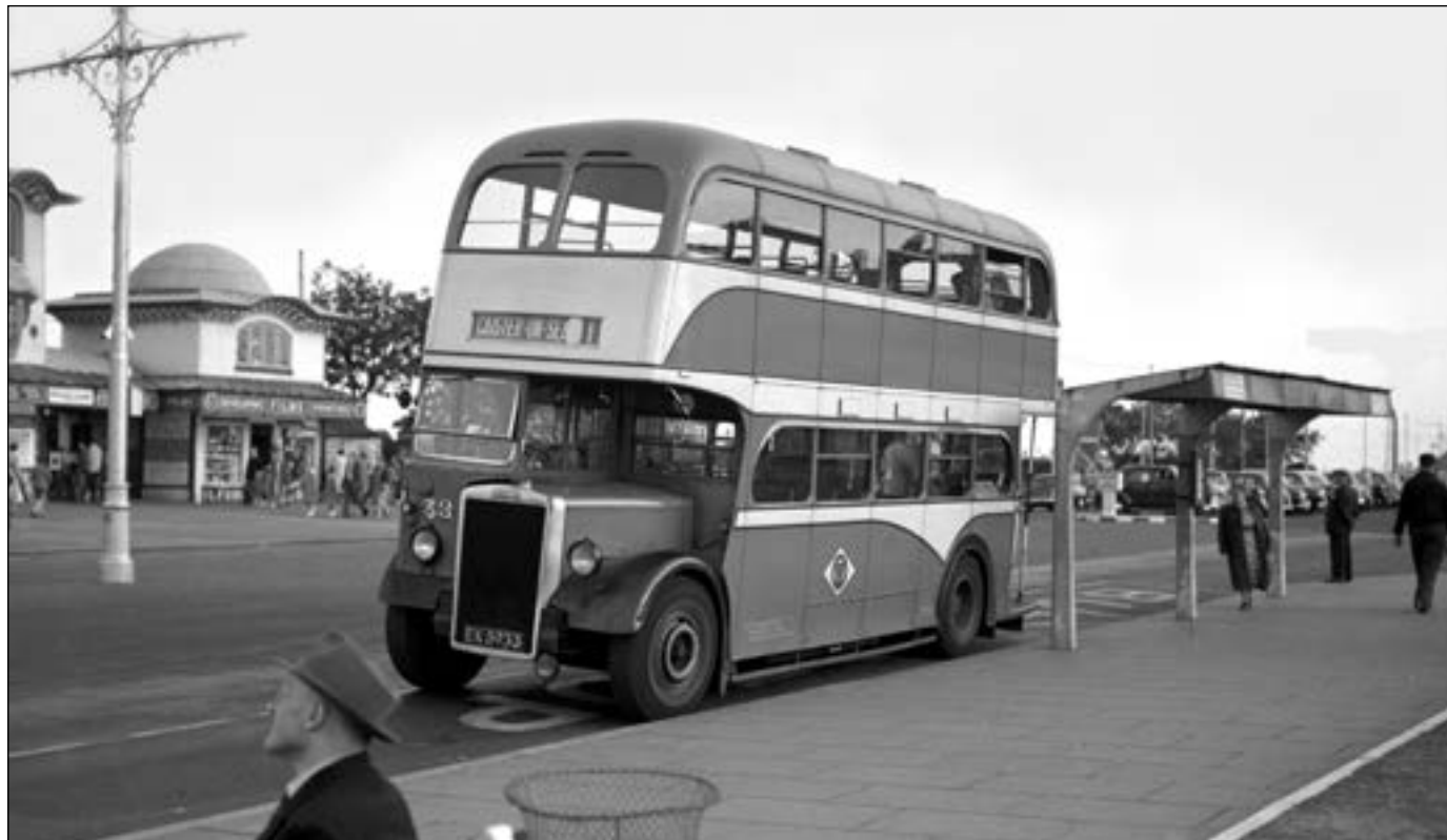
Showing its well proportioned body and D-shaped windows to good effect was Chester Corporation's No. 60 (HFM 170), one of three Daimler CVA6 types, here passing the town centre's famous Rows on route 25 in the early 'fifties. Andrews Liver Salts graced the sides of many buses in those days and every decent sized town boasted a branch of the Maypole combine.
