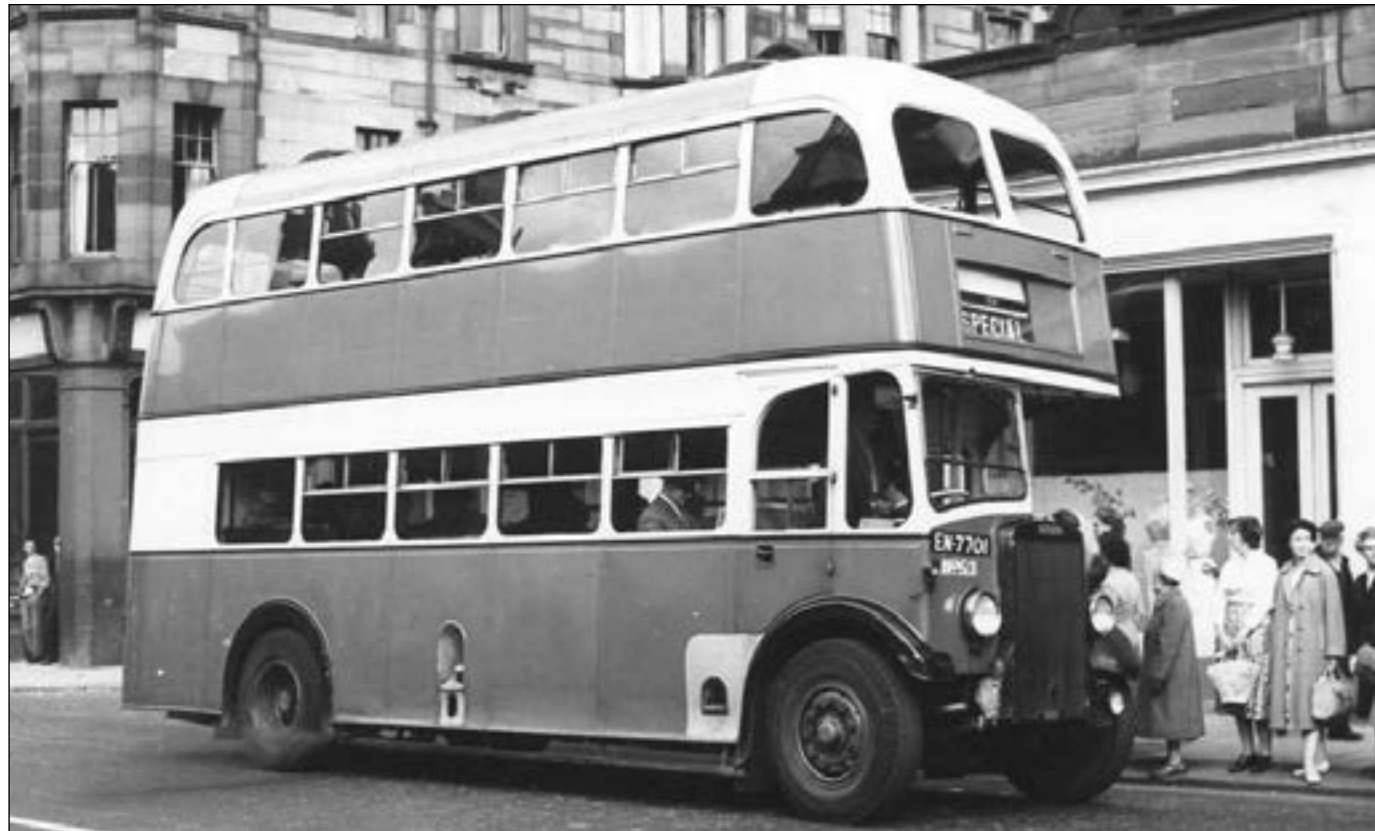
Complete with trade plates is Bury Corporation No. 73, one of four 1938 TS8c chassis rebuilt to TD5 designation and this time with double-deck bodies. It is standing at the pit-head complex of Summersales Colliery. The original four Tigers had been supplied with Burlingham single-deck bodywork but Bury were unable to sell them in this form and in late 1951 decided to have them rebodied. They were all withdrawn in 1958 and passed to Tiger (dealer) of Salsburgh who sold three of them to Paton Brothers of Renfrew and the other to Dunoon Motor Services. Number 53 in the Paton fleet was spotted a few years later at an unidentified location.
