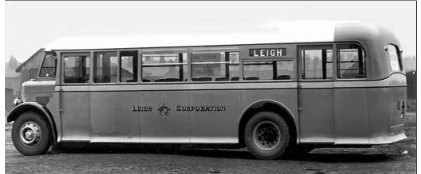
Leigh Corporation number 65, right, shows the final pre-war design of single-deck service bus bodies. Similar vehicles but with rear entrances were produced for Cumberland Motor Services. The radiator confirms Massey's records that this is indeed a Titan double-deck chassis, and without autovac. Is it by now diesel-engined? The maker's view in the yard of one from an earlier batch shows a dual-doorway layout. The third photograph shows No. 65 again, this time waiting at Lower Mosley Street bus station in Manchester, doubtless on hire to one of the combine operators who then used this long-distance coach station where the Bridgewater Hall now stands. (HSPC lower two)
