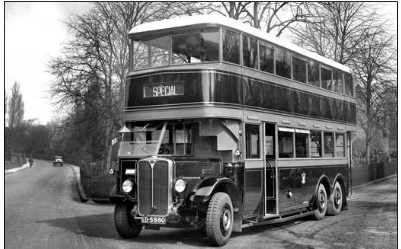
Warrington Corporation purchased two 30ft long AEC Renown chassis which were intended for London Transport. Massey Brothers supplied the 65-seat dual entrance/exit bodywork and No. 39 (ED 5880) is shown in the Warrington livery of Munich Lake (Maroon) and Citron (Yellow) at the corner of the A56, opposite the Walton Arms, in April 1930. The two vehicles remained in service until 1937, and whilst the design looks strange, even dangerous perhaps, it was no more so than the hundreds of tramcars then in use throughout the country with their equally restrictive layout as seen on page 30. Nevertheless, the front staircases were fairly soon removed, possibly following an inspection under the new 1931 Road Traffic Act. This was Massey's first order from Warrington; the operator took six Titan TD1s in 1931 but never patronised the Pemberton factory again. Had the body design been a step too far, closing the door on any future prospects? (STA)
