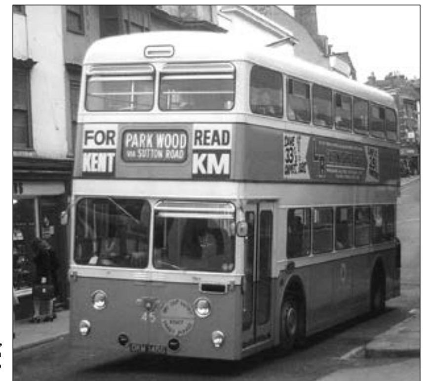
Maidstone Corporation Leyland Atlantean number 45, OKM 145G, clearly demonstrates the great difference in body styling adopted when rear engined chassis came to be dealt with.
