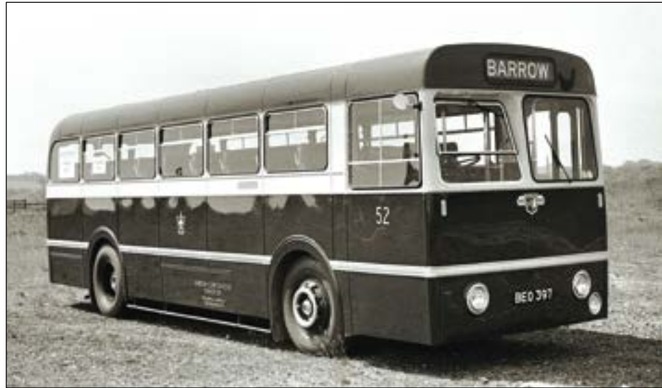
Barrow Corporation had not ordered any new single-deckers since 1933, when, in the early 'fifties, several were purchased, one of which was this Leyland Royal Tiger PSU1/13, number 52 (BEO 397) with dual-purpose seating for 43 passengers, used mainly for private hire. The vehicle was used in an advertisement for 'brighter windows' as seen on the previous page.
