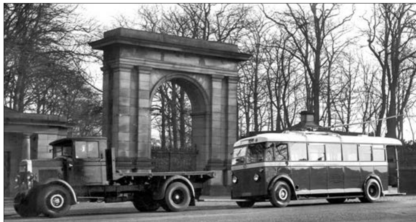
Posed outside the main gates of Wigan's Haigh Hall in December 1936 having been towed from Massey's factory by the Leyland truck which would deliver it to Tees-Side is Leyland TB3 trolleybus No. 10, one of a batch of five, remaining in service until 1945 when they were bought by Southend Corporation for £250 each. The 'Scottish' style rear entrance is noteworthy. As is the continuation of the six-bay construction in contrast to the five-bay design of the St Helens models above. (STA both)
