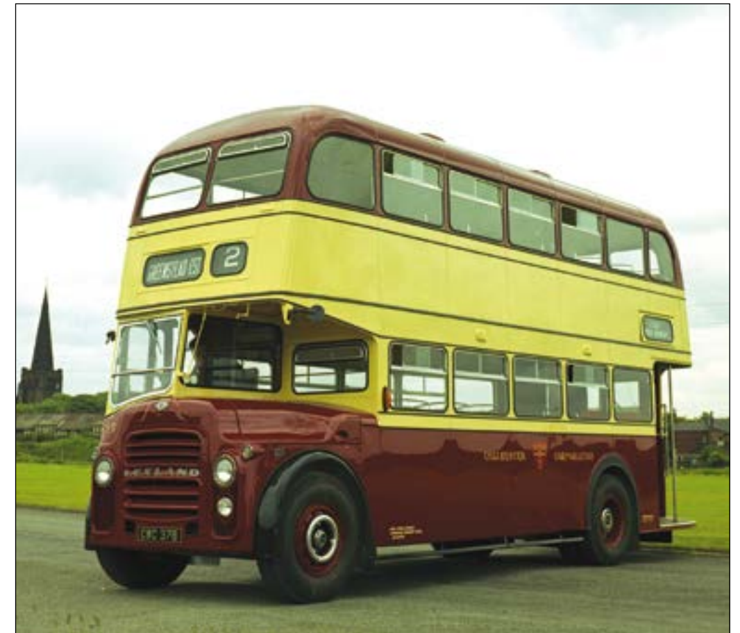
Colchester Corporation's No. 37 was one of three Leyland Titans designated PD2A/30Spl denoting that it was 7ft 6in wide. The equivalent 8ft 0in wide standard version (PD2/31) had by then been discontinued. It is shown before delivery in 1964.
