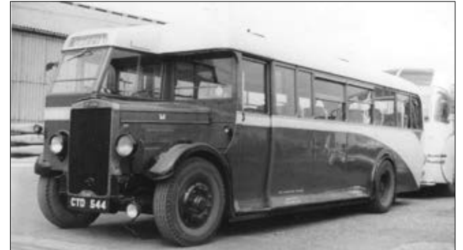
Leigh Corporation number 65, right, shows the final pre-war design of single-deck service bus bodies. Similar vehicles but with rear entrances were produced for Cumberland Motor Services. The radiator confirms Massey's records that this is indeed a Titan double-deck chassis, and without autovac. Is it by now diesel-engined? The maker's view in the yard of one from an earlier batch shows a dual-doorway layout. The third photograph shows No. 65 again, this time waiting at Lower Mosley Street bus station in Manchester, doubtless on hire to one of the combine operators who then used this long-distance coach station where the Bridgewater Hall now stands. (HSPC lower two)
