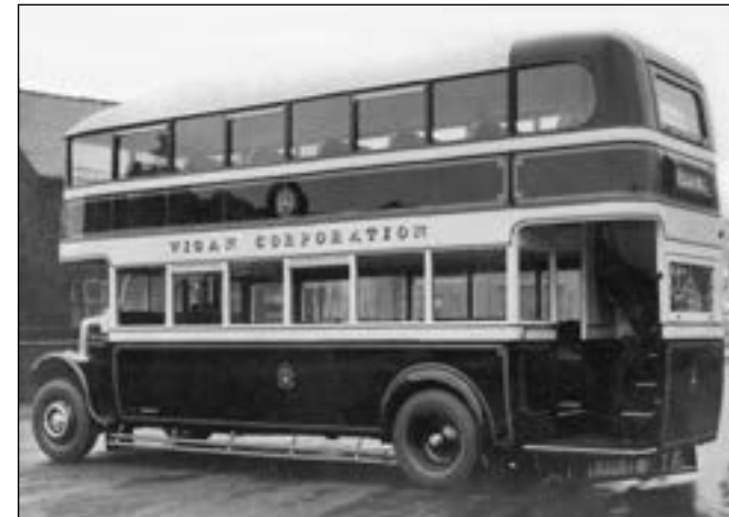
Wigan Corporation No. 74, one of ten Leyland Titan TD1s with 48-seat Massey-built lowbridge body to the Leyland design, which was delivered in 1931.
