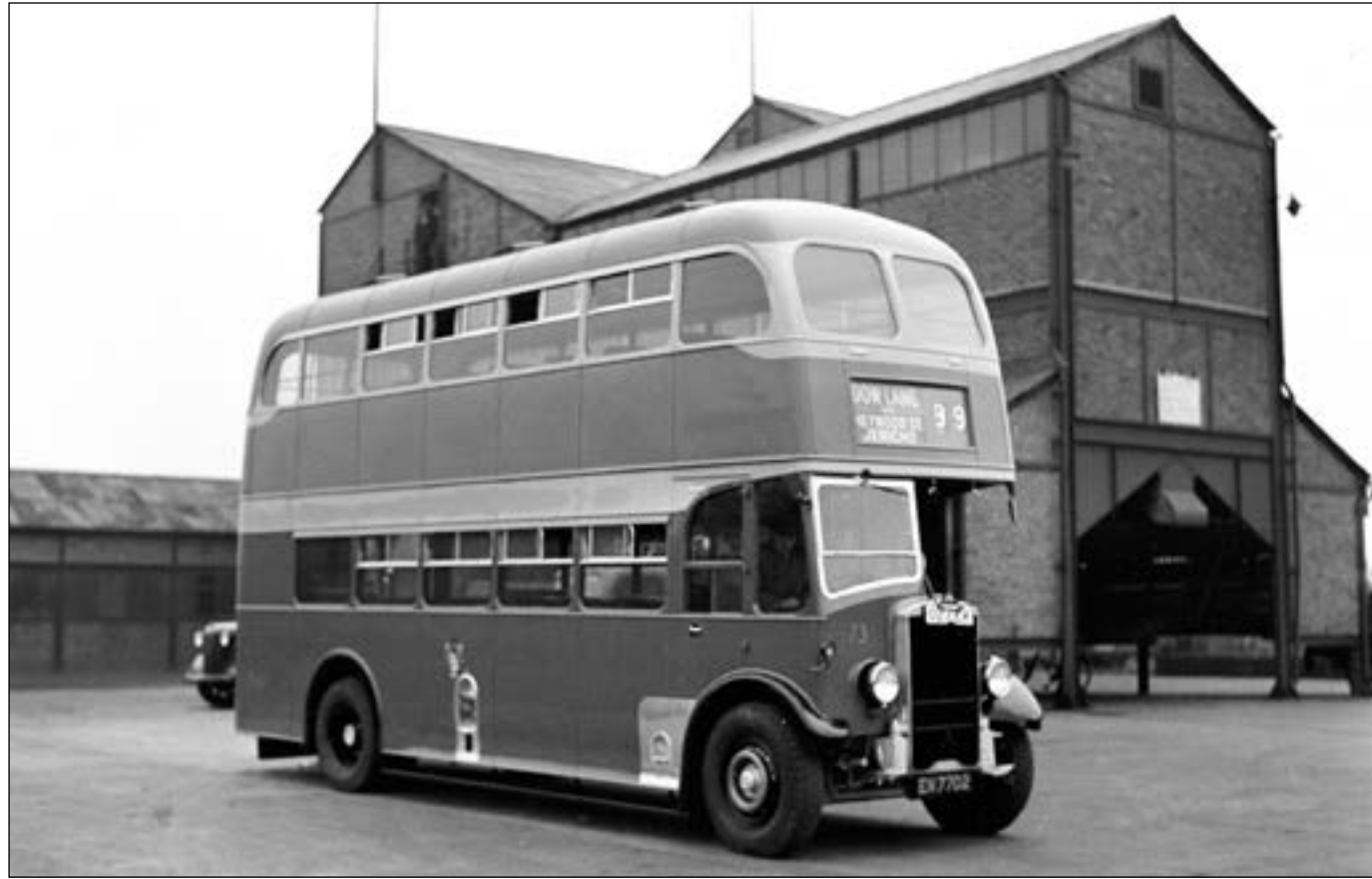
Complete with trade plates is Bury Corporation No. 73, one of four 1938 TS8c chassis rebuilt to TD5 designation and this time with double-deck bodies. It is standing at the pit-head complex of Summersales Colliery. The original four Tigers had been supplied with Burlingham single-deck bodywork but Bury were unable to sell them in this form and in late 1951 decided to have them rebodied. They were all withdrawn in 1958 and passed to Tiger (dealer) of Salsburgh who sold three of them to Paton Brothers of Renfrew and the other to Dunoon Motor Services. Number 53 in the Paton fleet was spotted a few years later at an unidentified location.
