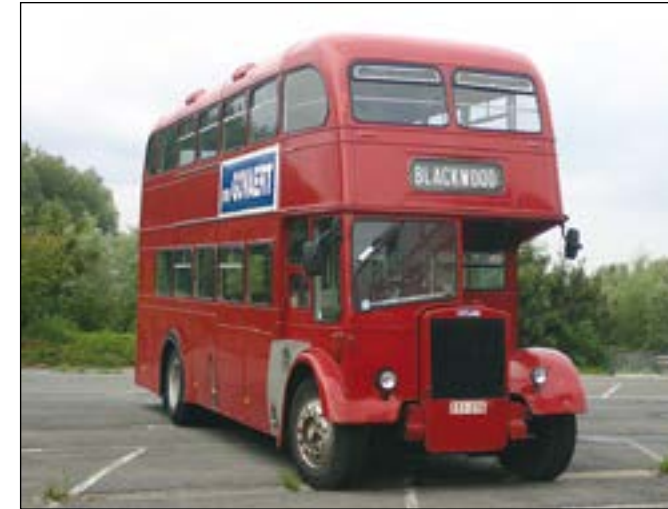
West Monmouth No. 13 (UWO 688) was originally a Leyland Titan PD2/41 'special' with Willowbrook single-deck body built for the Bargoed Hill route in 1959 but was rebuilt in 1966 (when the route changed) with this Massey Bros. lowbridge double-deck body. It was spotted in Wetteren, Belgium in August 2004.
