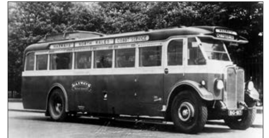
As detailed in the text above, Maxways ordered six AEC Regals with 32-seat rear entrance bodywork for their North Wales coastal service. Here we see BG 617 posing for the camera prior to delivery in June 1932. (STA)
