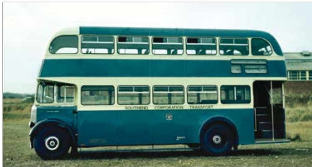
Southend Corporation's number 298 was a Leyland Titan PD2/12 with 55-seat lowbridge bodywork. It was one of a batch of twelve supplied in 1955/6 and is seen before delivery.
