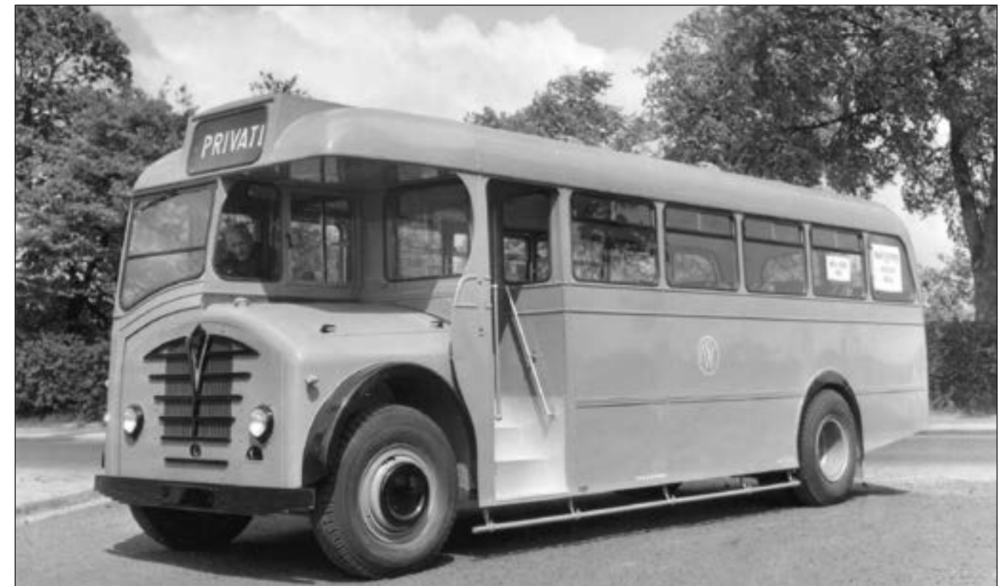
During 1953/4 Masseys also built two 31-seat bus bodies on Foden PVSC6 chassis for the Wankie Colliery in southern Rhodesia – now Zimbabwe – one of which is seen prior to delivery at Foden's works and described in the article above. The item will be seen to record a bonus paid to the drivers – a spring bonus – which resulted in an 80% reduction in broken springs. In between dodging potholes and avoiding snakes, their drivers appeared to have a fairly normal sort of occupation for bus and lorry drivers. (PT)
