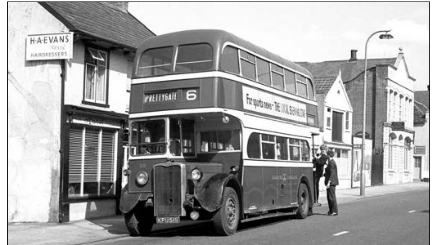
Massey Brothers only ever bodied one Crossley after WWII, this bus becoming a firm favourite with many enthusiasts. It was numbered 55 in the Colchester fleet and dates from November 1948. The long droopy wings spoil the appearance of an otherwise pleasing design. It is seen here on the number 6 service in the early 1960s. (LM)
