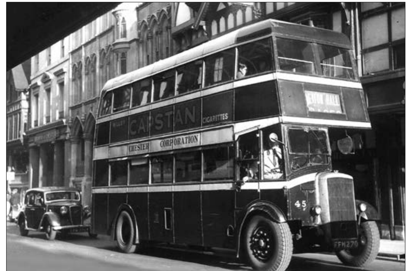
Chester had need for more vehicles to serve the Sealand American airbase which provided a home for many of the US bombers used during the conflict. Here one of its Daimlers, No. 45 (FFM 270) is seen after the war in the city's shopping area. This was a CWG5, easily recognised by the vertical slats of the radiator.
