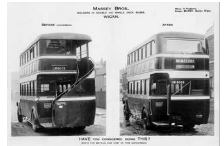
The original Leyland Titan TDI models featured this open staircase arrangement which, within a matter of months, had been superseded by the enclosed version seen on the right. Massey Bros. had been building the enclosed version for Wigan to Leyland's design and quickly realised that there was a market for converting the earlier models – which clearly had many more years life left in them – into the by-then more commonly used enclosed version. By chance a Bolton vehicle was converted back to open staircase format when it was saved for preservation, and can be seen in the LVVS museum at Lincoln. (STA)
