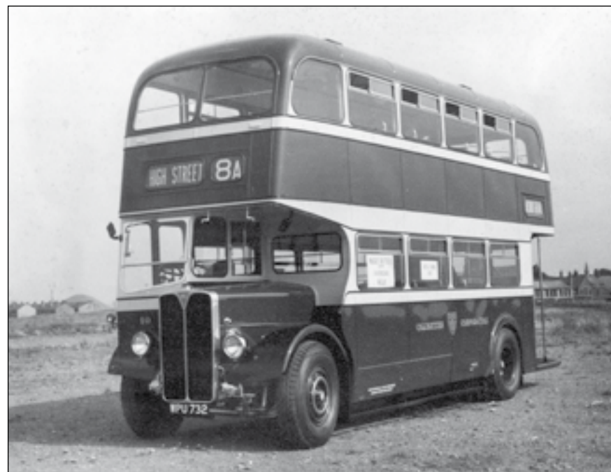
One of three stylish AEC Regent IIIs supplied to Colchester Corporation in 1953. This is number 10 (WPU 732) shown before delivery. All gave invaluable service before being withdrawn in October 1971. Comparison of this vehicle and the Heyfordian Daimler above clearly show the increase in width to 8ft of the Colchester vehicle's bodywork.
