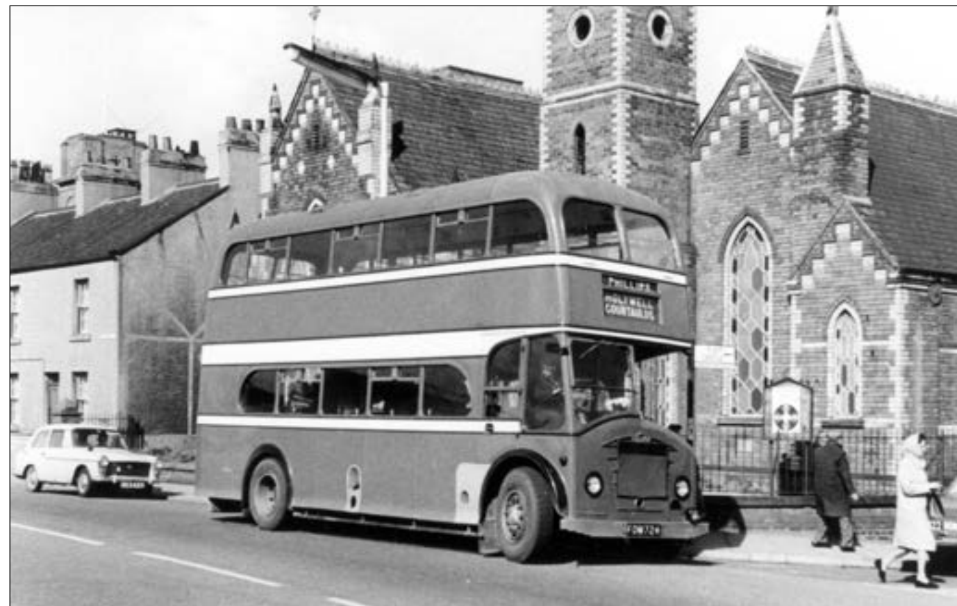
Below: A splendid shot of Phillips of Hollywell's Foden PVD6 (FDM 724) as it wends its way through its hometown near to the Dee estuary in north east Wales en route to the local Courtaulds factory in March 1967. The Foden bonnet blended very well with the Massey body curves.
