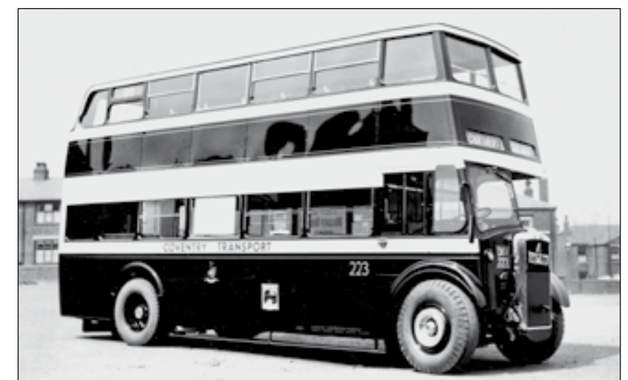
Whilst this is very clearly not a Massey design, records show that this Daimler COA6, No. 233 (DKV 233) is indeed a Massey built vehicle. It was assembled in 1939 from metal sections, as were the other vehicles in the batch for Coventry, but the rest were either Brush or Metro-Cammell products and this example from Wigan was supplied for comparison. It was priced at £890 as against £1,021 for the Birmingham product, but maybe Massey had seriously underestimated the true cost of production. Whatever the actual situation the outcome was clear – Coventry did not pursue the idea and Massey's next metal-framed bus would be for Birkenhead in 1950 as shown on page 86.
