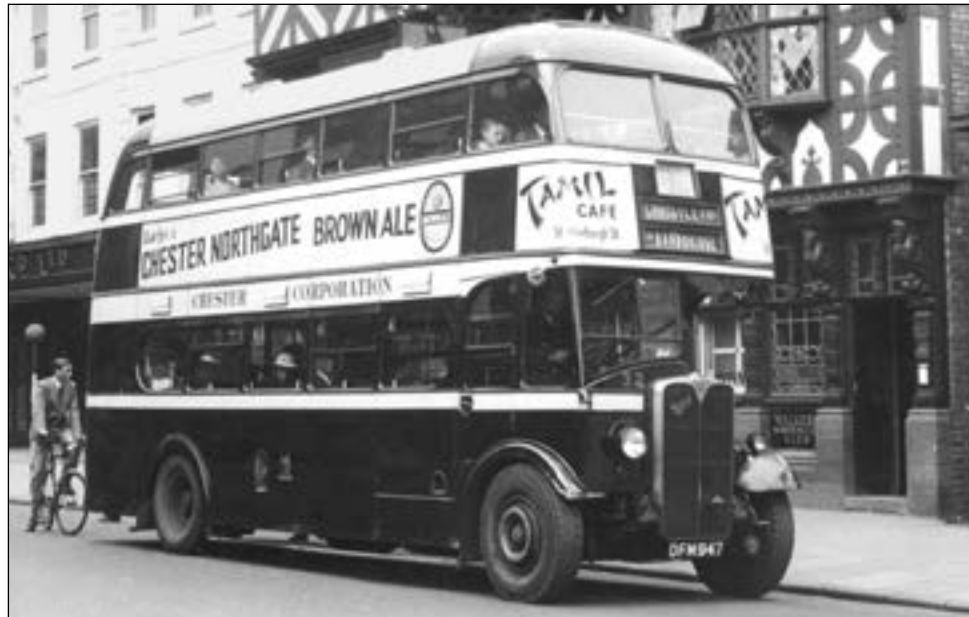
Chester No. 32 delivered in 1939 shows the curved frontal profile introduced around this time. It is mounted on an AEC Regent II chassis. By the time the next Chester vehicles, including No. 39 also on AEC Regent II chassis, were delivered in June 1940 the frontal profile had changed yet again with increased curvature to the front and heavier corner pillars, a design that was to be used with little modification for some years in the post-war period – see page 61. (HSPC)
