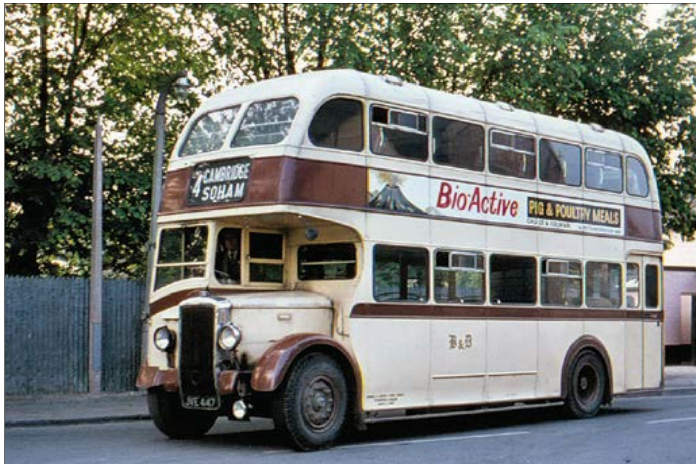
Burwell & District lowbridge Daimler CVD6 (JVE 447), complete with platform doors, supplied in June 1951 and shown here on a local service in 1965. Note the front rake applied to lowbridge buses by Massey Bros. in the late 'forties/early 'fifties period.; note also the not uncommon knocked backed lower radiator shell where the vehicle has 'grounded'. This bus gave 19 years service before being withdrawn in May 1970 and lay derelict until being scrapped in 1990. (GL)
