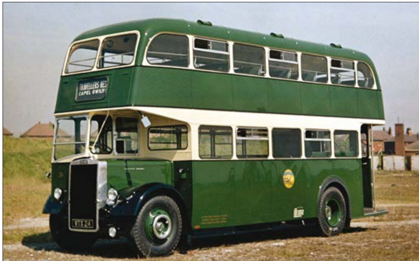
Photographed around the same time in July 1957 was Caerphilly UDC's No. 24, a Leyland Titan PD2/40 with 55-seat lowbridge body.
