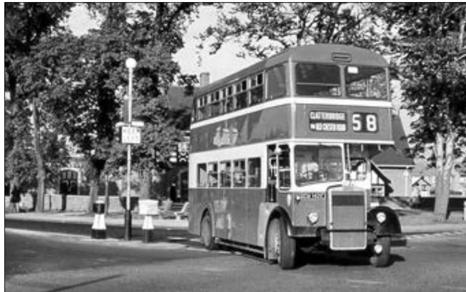
Birkenhead Corporation No. 142 is seen at Spital Cross roads, Bebington, in the early 'seventies. This was one of the second batch with the newer style of bodywork, the familiar curved front and roof profile giving way to a more upright frontal appearance.
