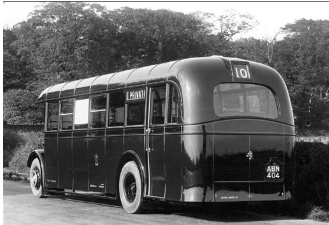
Showing its rear entrance body to good effect is this Leyland Tiger TS8c which was one of two with Massey bodies supplied to Bolton Corporation in the late summer of 1938. There were two more similar vehicles supplied at the same time but with dual-purpose bodies by Park Royal. (STA)
