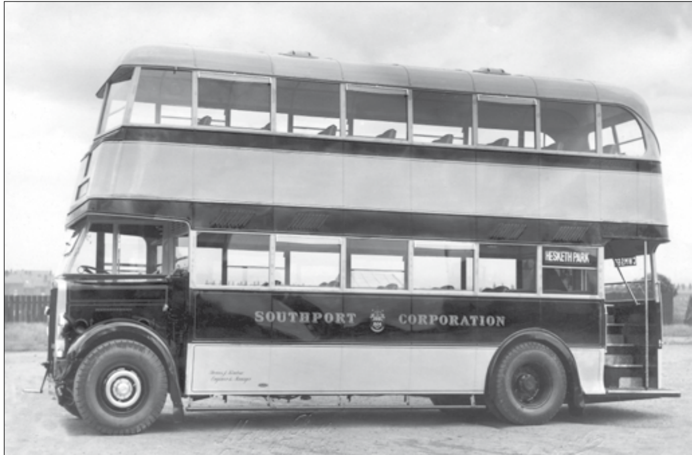
Southport Corporation No. 53, a Leyland Titan TD5c, was one of a batch of five delivered with clearly recognisable English Electric-designed bodywork in 1937. This must either have been an order placed with Massey to be built to EE design, or, possibly, sub-contracted from the Preston firm as it became increasingly busy with military orders. As Southport is only a few miles from Wigan it is perhaps surprising that Massey Bros. only ever received this one order from the seaside undertaking.
