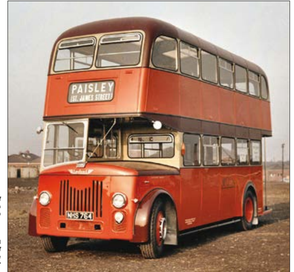
Showing the prominent colour scheme of McGill of Barrhead is this Leyland Titan PD2/30 (NHS 764) completed in March 1959.
