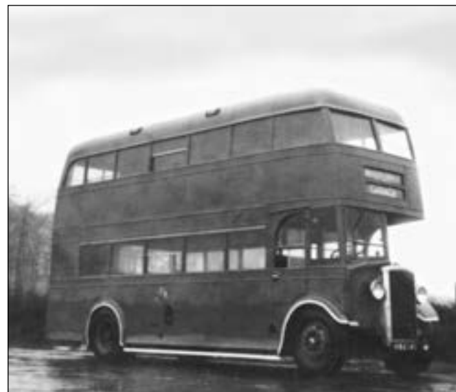
Posing for the camera prior to delivery, below, on a bleak day in April 1942 is Sheffield Corporation's No. A461 (HWA 141) an 'unfrozen' Daimler COG6, in full wartime livery, and believed to have been the only such example from the Daimler output. The body will be seen to be of the same design as that fitted to the four Regents, as seen left.
