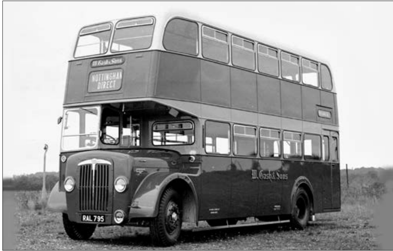
Numbered DD10 in the fleet of W Gash & Sons of Newark, Nottinghamshire, was this Daimler CVG6, seen before delivery in July 1954 and then soon afterwards in service. The Gash fleet, in two shades of green, was always well turned out and the rear platform doors and Daimler nearside mudguard arrangement help to produce an extremely handsome vehicle. (HSP left and below both)
