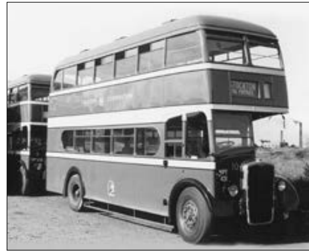
Massey-bodied Bristols were something of a rarity. Below is Stockton-on-Tees No. 10, a Bristol K6G built in 1947. Note the change in angle of the front panel, spoiling the line and giving the front of the body an awkward and old-fashioned appearance. (RLK)
