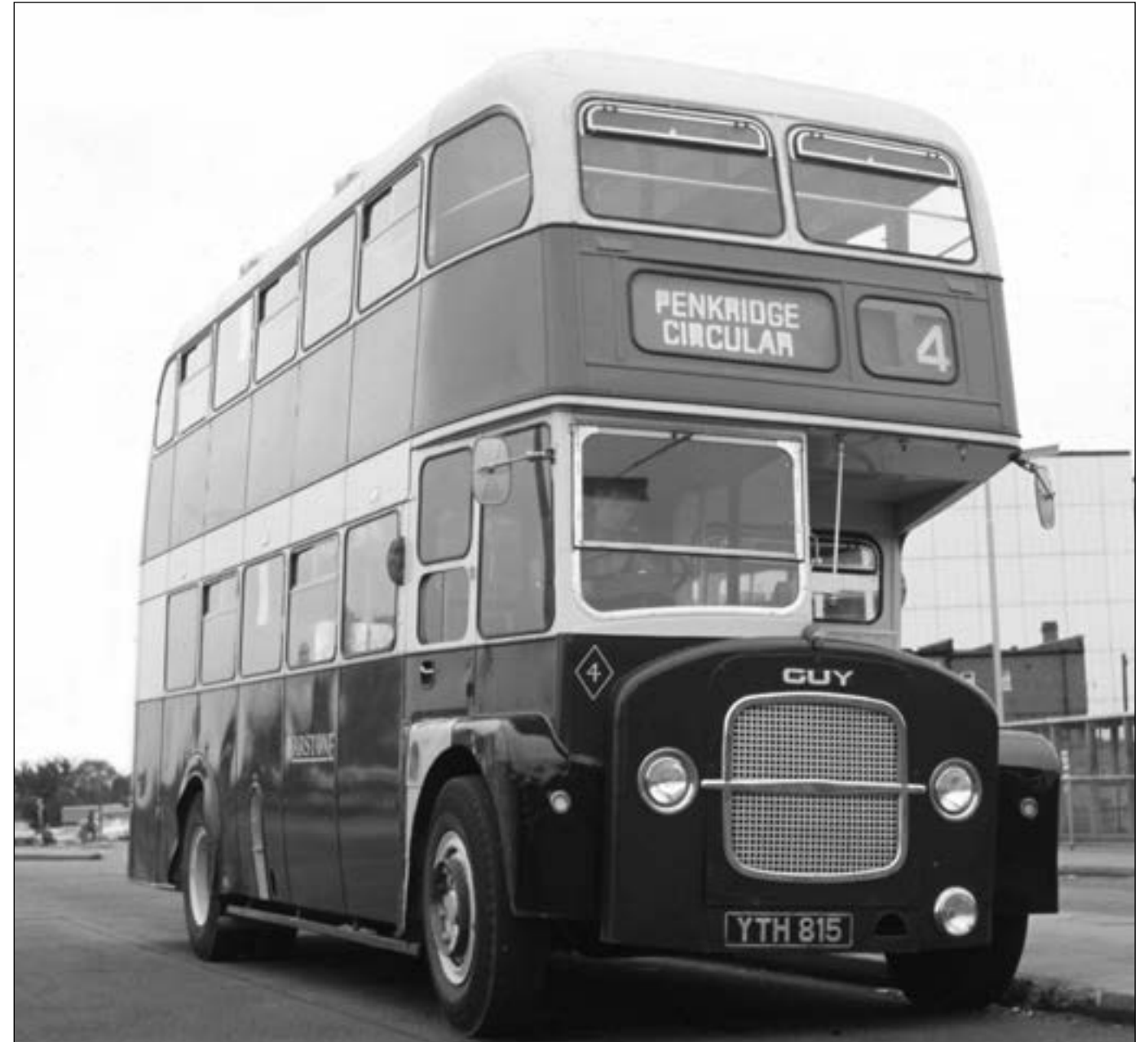
Rees & Williams were based in Tycroes, a village near Ammanford in south Wales. They took several Massey-bodied buses over a period of some 14 years and the vehicle pictured (YTH 815) was the last one purchased. It is a Guy Arab IV with lowbridge body fitted with platform doors and the distinctive if perhaps not very attractive 'Johannesburg' front. It is seen in the lower view resting between journeys on the Company's busy service 16, Llandilo to Ammanford, whilst in the larger view above it is now in the service of Warstones, in Staffordshire. (DC)
