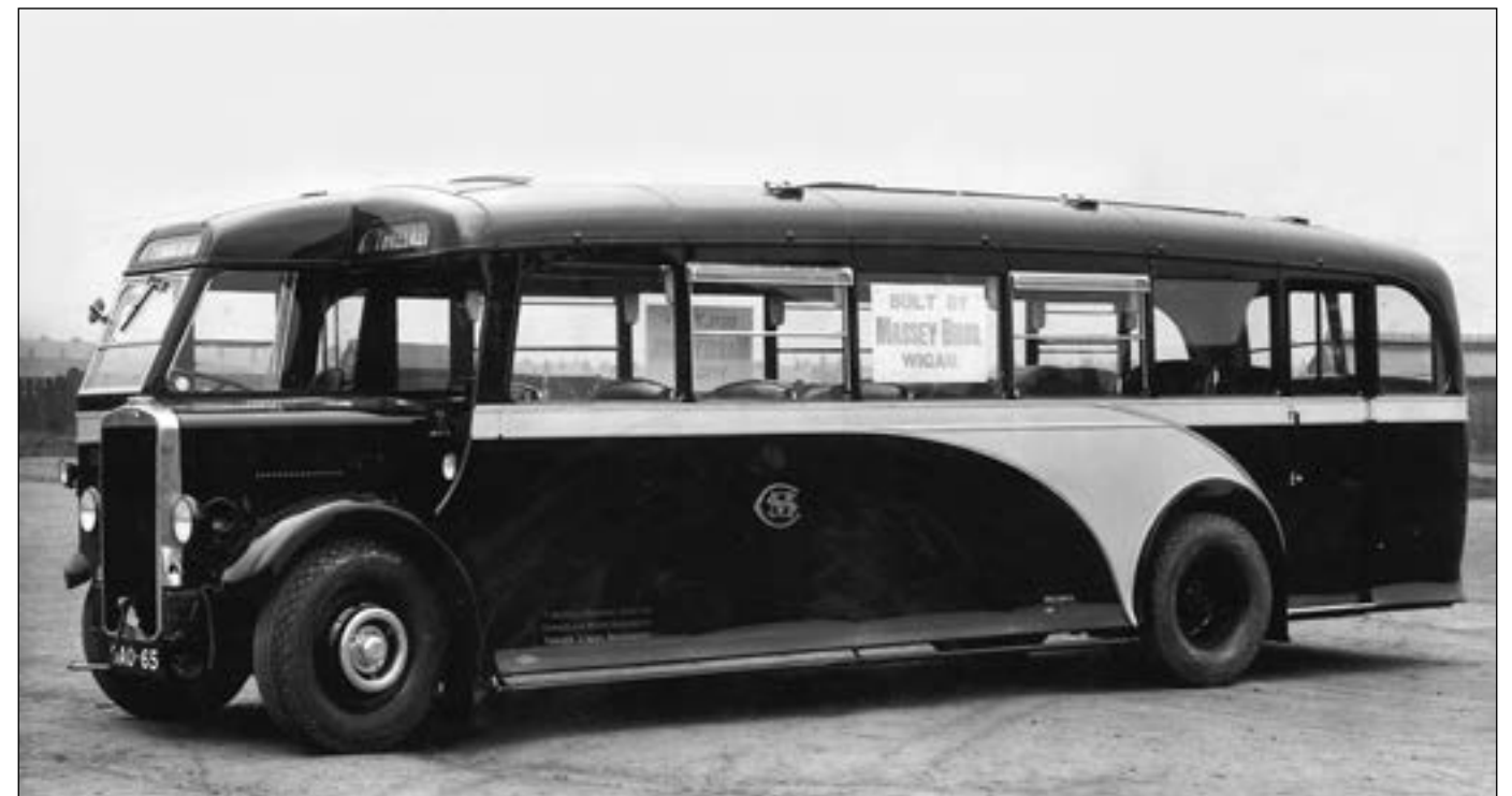
In 1938 Cumberland Motor Services took delivery of five Leyland Tiger TS8 half-canopy single-deckers with moquette covered seats that had higher than the usual standard backs giving extra comfort on longer routes. Number 139 is shown outside the Enfield Street coachworks prior to delivery, with outswept panels again in evidence. Sister vehicle No. 142 lasted in service until 1959 and was being used as a static site office in Methley near Leeds as late as the end of 1960.
