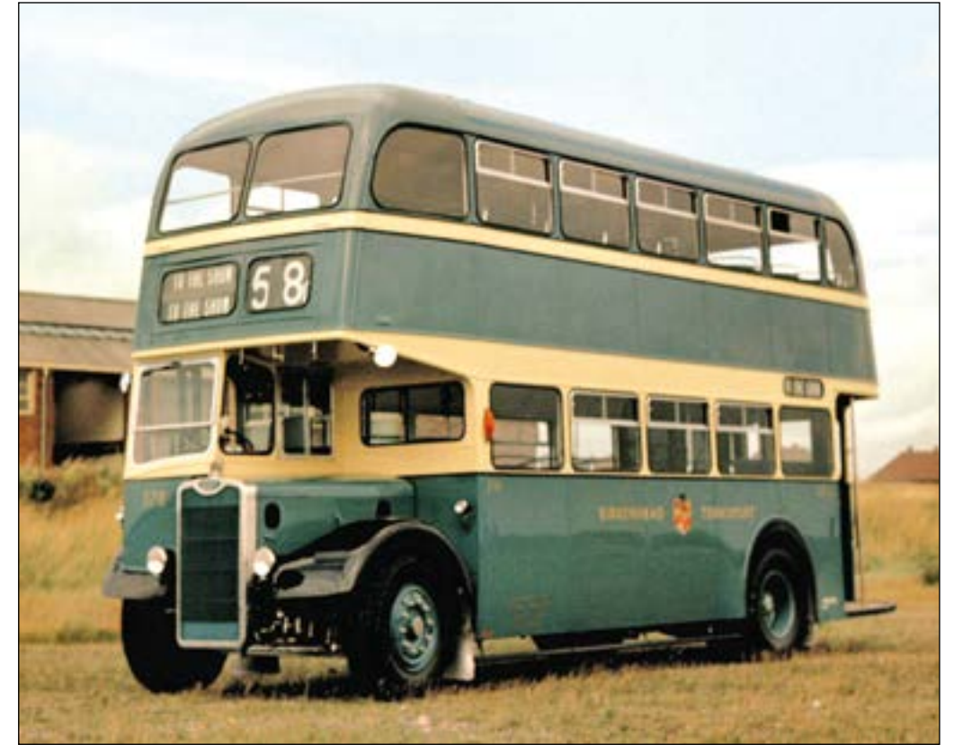
Birkenhead Corporation's intake for 1956 was 15 Guy Arab IVs, five with East Lancs bodywork, the remaining ten by Massey including No. 378 shown here prior to being exhibited at the Commercial Motor Show and having different interior finishes from the others. These were also the first vehicles in the fleet to be fitted with flashing direction indicators.
