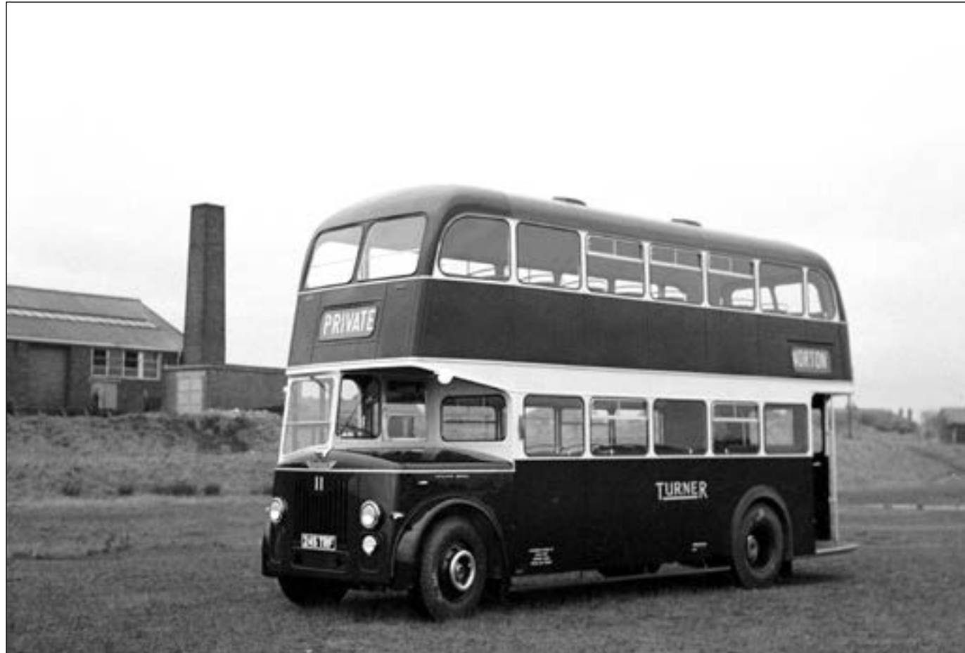
Turners of Brown Edge, a village between Leek and Stoke-on-Trent, took delivery of this Leyland PD2/30 in December 1957 with open rear platform bodywork and numbered it 11 in the fleet. When number 12 arrived in June 1959 it was a Titan PD3/1 and featured a forward entrance with sliding door, as seen below. After sale by Turners it saw further service in the north east with three further owners and was finally scrapped in 1979.
