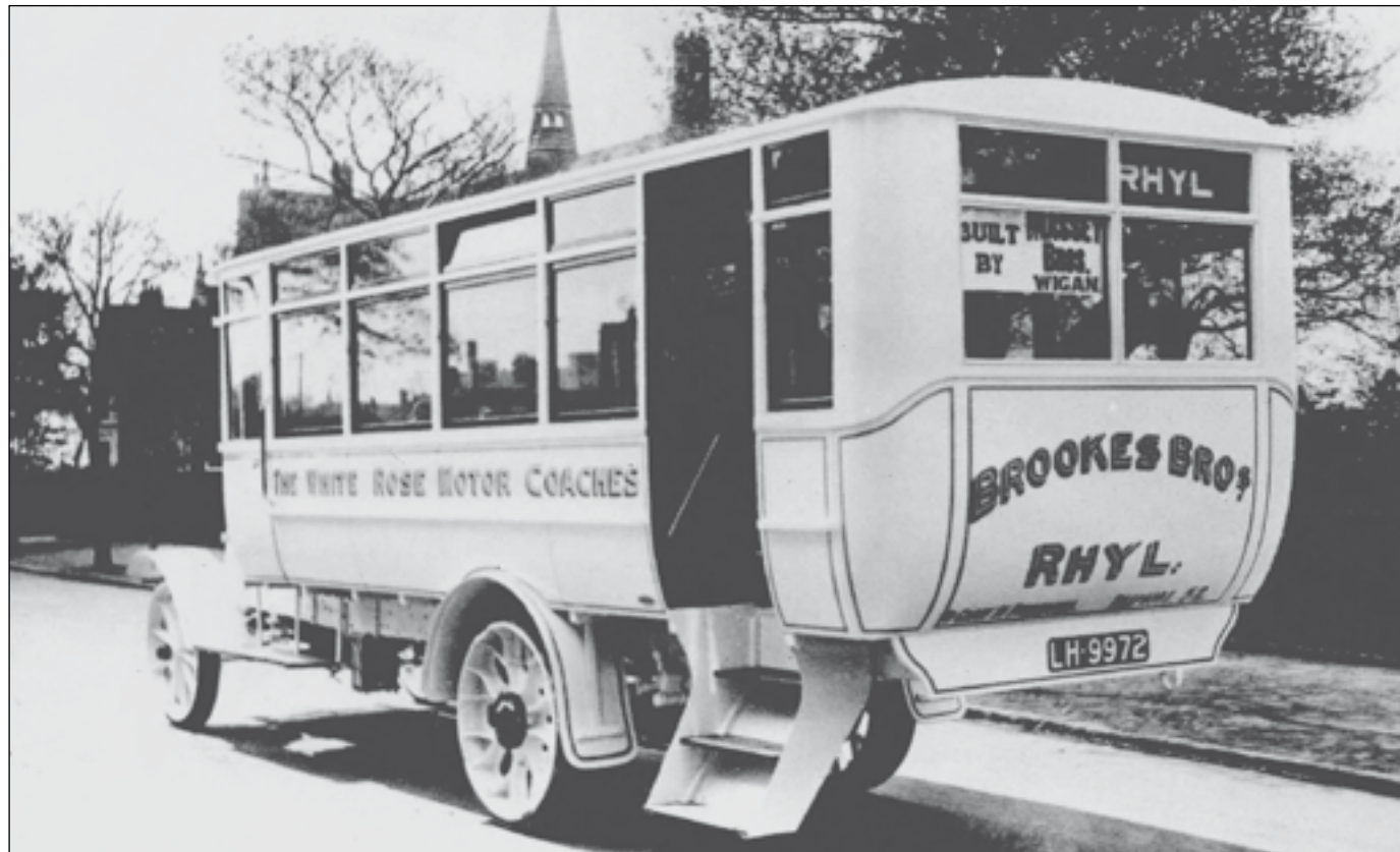
This Daimler B-type started life in London before being purchased by Royal Blue in Llandudno, North Wales, and fitted with a charabanc body as seen here in Rhyl. The robust, if somewhat rudimentary, chassis, was capable of more than seasonal summer excursion work, of course, and like many others purchased in the early post-war years was soon rebuilt as a saloon bus. This example was rebodied with a Massey 32-seat body as seen below in May 1922 for new owners Brookes Brothers based in Rhyl. Trading as White Rose Motors the firm grew to an impressive size and became a considerable thorn in the side of the Crosville Motor Company until the takeover after the LMSR investment in Crosville. The company had considerable charisma and one of its mid-twenties Leyland-bodied Leyland SG-types has been lovingly restored by Mike Sutcliffe, the Leyland specialist, ensuring this splendid livery and much-loved operator will not be forgotten. (STA upper)
