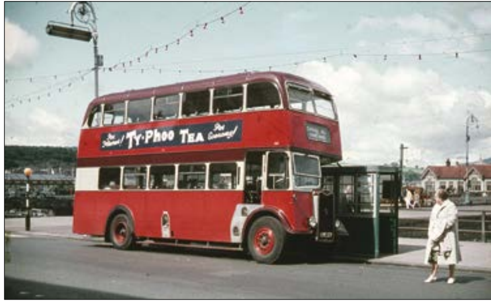
Looking smart in its owner's livery, Rothesay Motor Services, is this Guy Arab II which was one of four wartime chassis re-bodied with 58-seat highbridge bodywork. The original bodies had been Park Royal wartime utility models. (IGMS)
