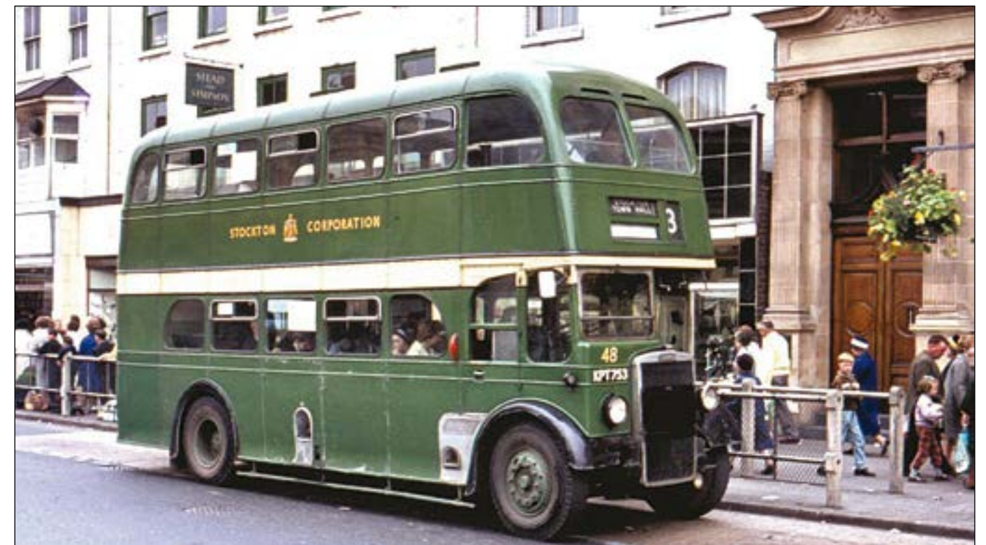
Stockton Corporation placed orders for a total of 43 Massey-bodied double-deckers in the immediate post-war period. Number 48 was one of a batch of 25 Leyland Titan PD2/3s with typical body for that period and delivered in the final three months of 1949. It was photographed in Stockton High Street in September 1963. (GL)
