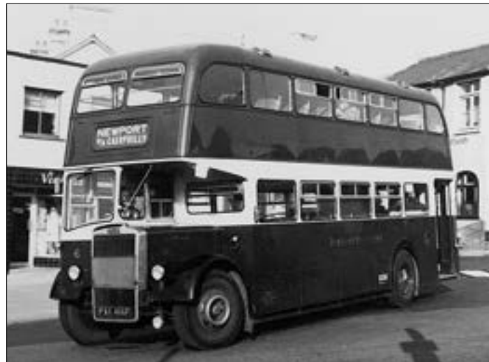
Massey Bros. had the distinction of building the very last lowbridge (side gangwayed) double-decker, and it is seen here. (RM)
