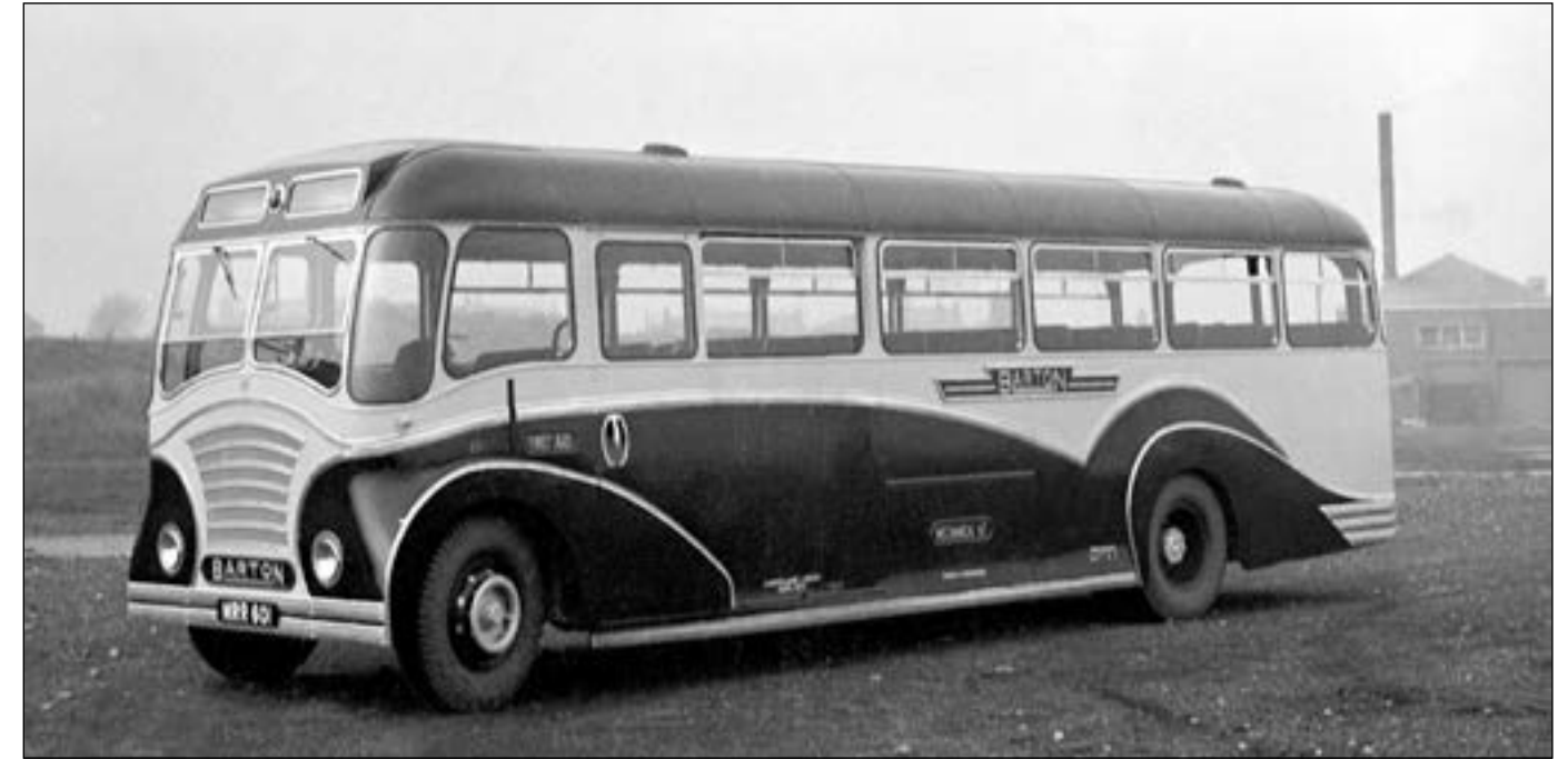
Barton Transport No. 651 was one of a number of rebuilds undertaken by this independent during the post-war period, and in this instance designated BTS1. The chassis on this vehicle was previously a Leyland PS1 from 1948 (No. 541) with a Duple body but it was rebuilt in 1951 with a new 30ft chassis frame and sent to Massey Bros. for a new dual-purpose body which was photographed in October 1951 prior to delivery. It was withdrawn in 1966 and sold to a church youth club. In June 1972 it became a mobile caravan, but in 1973 was back in service with Gosport Buses of Glasgow and was last seen in Ayr in 1979. Pictured below is the rear of 651 also taken when new at Pemberton. Despite the extent of the reconstruction it retained its original registration number throughout its life.
