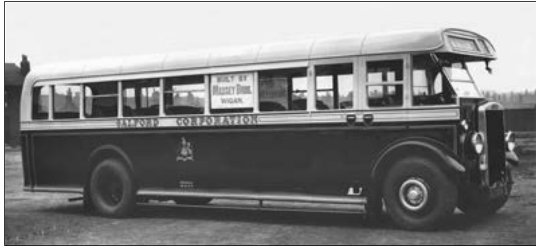
Salford No. 6, RJ 7004, was one of three Leyland Tiger TS7s built in 1937. All were withdrawn in 1950 when the operator's need for single-deckers was being reduced, and were sold for further use, but they were the last Massey vehicles delivered to the operator, Metro-Cammell and Leyland metal-framed bodies being preferred.
