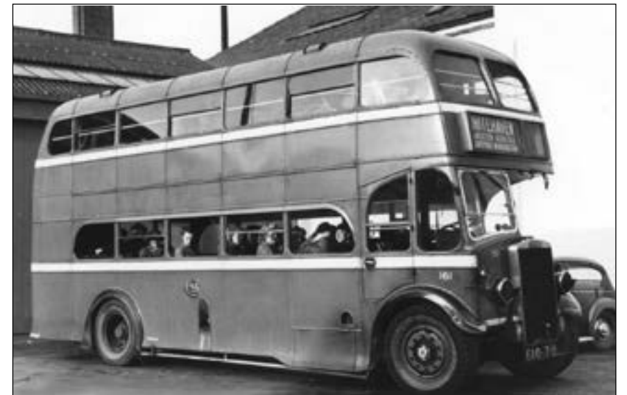
Cumberland Motor Services No. 161, EAO 701, was one of five Leyland Titan TD7s supplied in 1941 with Massey bodies. They were built entirely to peacetime standards and were delivered in the traditional red and cream livery. By the time this photograph was taken in Carlisle Bus Station, as it was about to depart to Whitehaven, it had been repainted by the operator in wartime grey and white livery. Note the masked headlamps, and the white painted stripes at front and rear to aid visibility by others in the blackout. (SLP)
