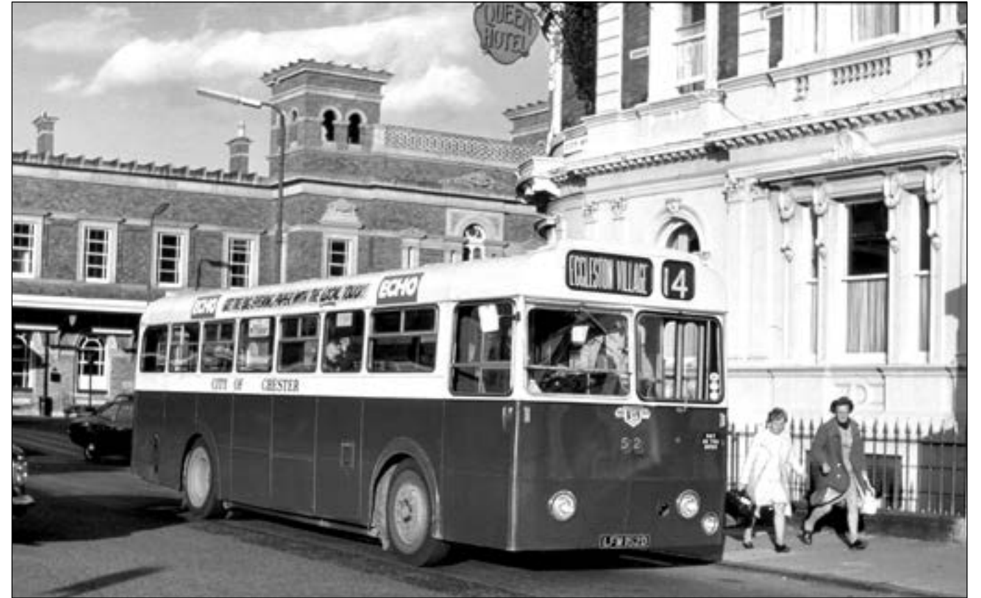
One of the three Chester Corporation dual-entrance Leyland Tiger Cub PSUC1/1s seen here on 30 July 1977. Number 52 dates from 1966 and clearly shows the large destination displays favoured by this operator. Notice also the flap for the 'Pay as You Enter' sign, open in this instance but closed when a conductor was being carried.
