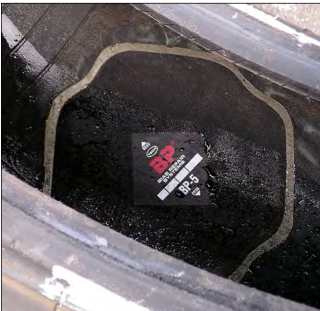
Improper Repair, Bias Ply Patch In a Radial Tire, Note Also the Misalignment
