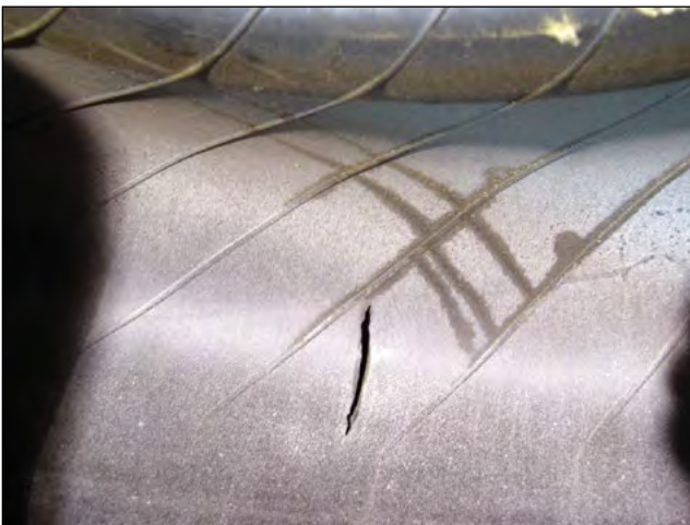
EFFECT: Inner Liner Split CAUSE: Sidewall Impact
