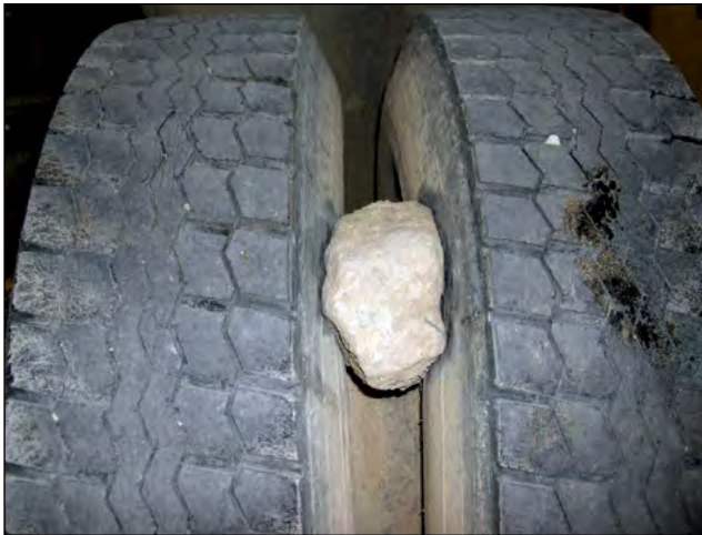
EFFECT: Sidewall Damage CAUSE: Object Wedged Between Dual Assembly
