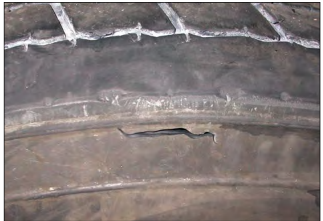
Sidewall Rupture Shock
