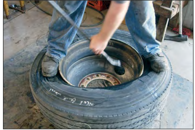
8 Mount second bead using same method.
