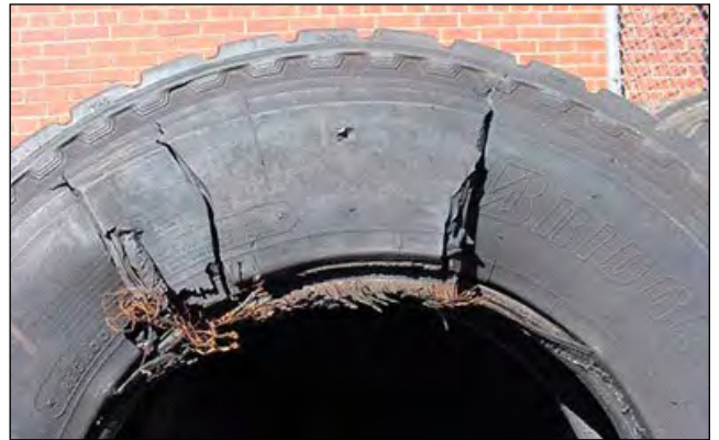
3rd Stage – Partial Unwrapping of the Casing Ply
