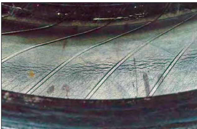
Potential Zipper Rupture
