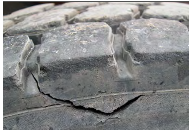
Sidewall Area Damage
