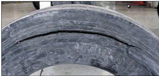
Circumferential Rupture of Casing Ply or "Zipper Rupture"
