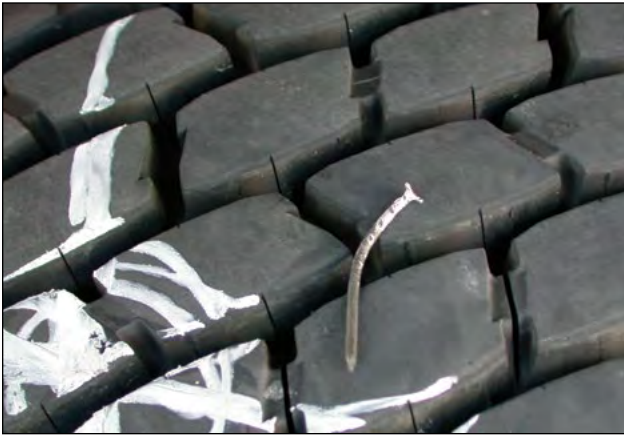
Inspect for Penetrating Objects
