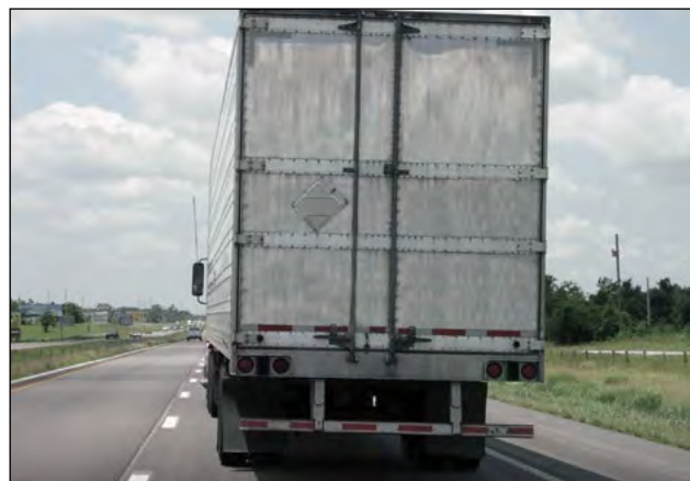
A misaligned (dog-tracking) trailer may also be the cause of steer tire wear.
