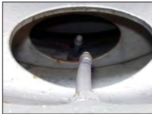
Incorrect Dual Wheel Placement
