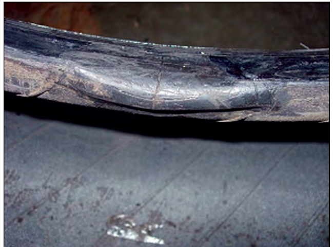
Bad Bead Repair
