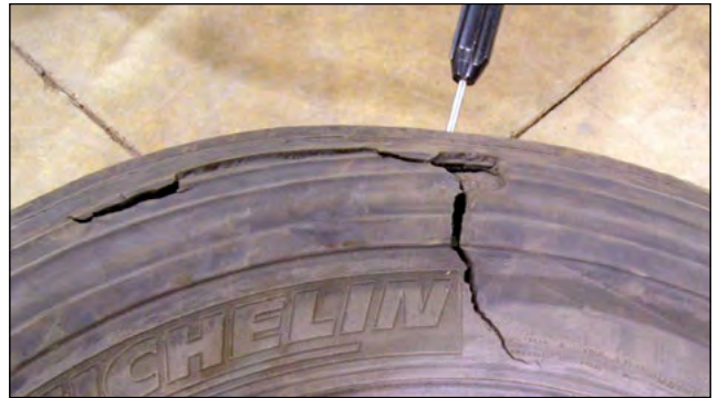
EFFECT: Crown/Sidewall Injury Resulting in Tire Pressure Loss CAUSE: Nail Hole Bolt/Debris Penetrating the Liner
