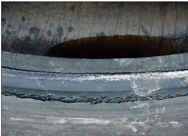
2nd Stage – Bead Splitting from Heat
