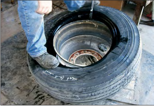
7 If necessary, continue to work the first bead on with proper tubeless tire tools like T45A tire iron.
