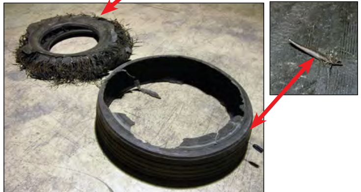
EFFECT: Run-flat CAUSE: Crown Perforation/Penetration
