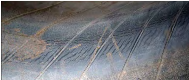
EFFECT: Inner Liner Marbling - Creasing CAUSE: Underinflation
