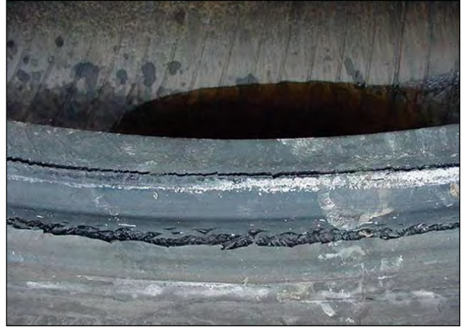
2nd Stage – Bead Splitting From Heat
