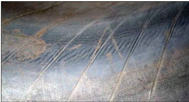
EFFECT: Inner Liner Marbling - Creasing CAUSE: Underinflation
