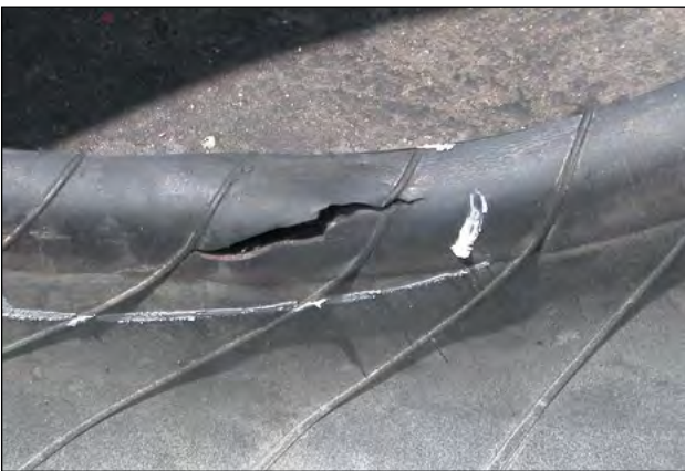
Bead Damage Caused by Mounting/Dismounting
