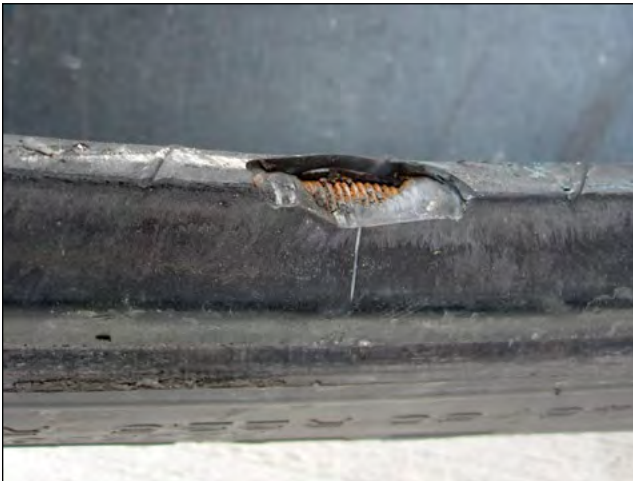
EFFECT: Bead Tearing From Mounting/Demounting CAUSE: Insufficient Lubrication, Improper Tools
