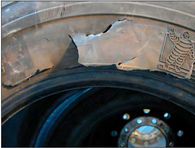
EFFECT: External Rubber Damage CAUSE: Severe Impact
