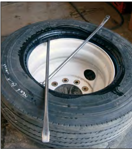
7 Completely unseat the first bead.
