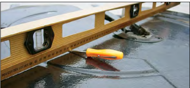
Distortion of the 5th Wheel
