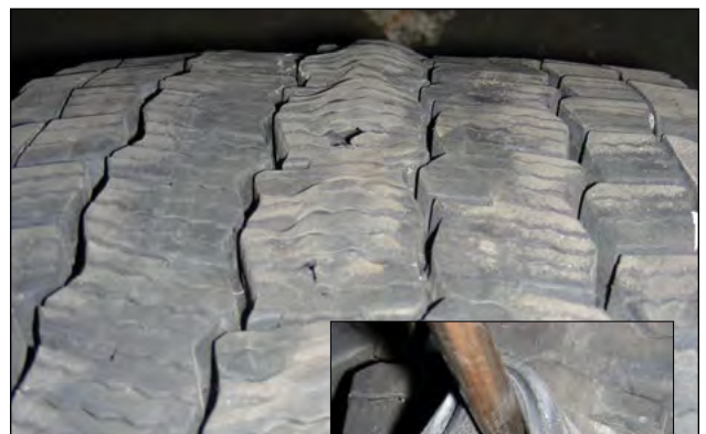
EFFECT: Internal Deterioration of the Tread Rubber
