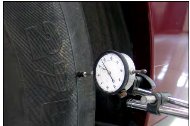
Measuring Lateral Runout on Outside Shoulder
