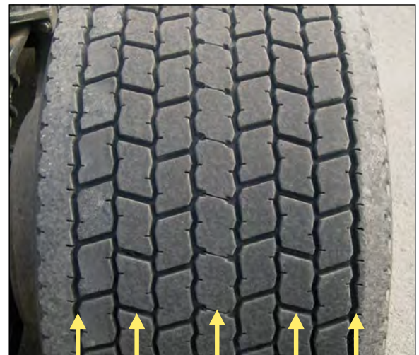
Inset: Notice appearance of shoulder-scrub on side of tread-blocks inner/outer shoulders.
