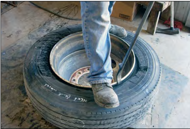
9 Use the proper tool like T45A tire iron, not the duck bill hammer.
