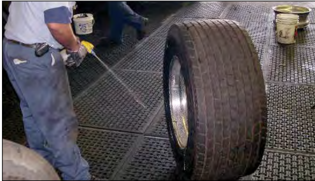
Lubricating Beads for Dismount
