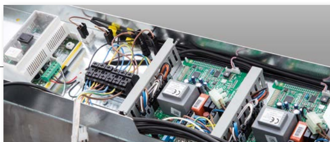
Assembly of the electronic PCBs for the management of the thermal elements and BCM 2.0
