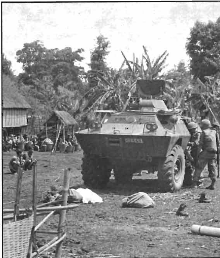
V-100 COMMANDOS WERE USED IN VIETNAM FOR POLICE AND CONVOY ESCORT DUTIES.
