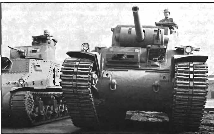
The M6 Heavy tank, at right, seen in comparison with the M3 Medium. Although a production tank, the M6 - at 60 tons - was thought to be too heavy for fighting in Europe and was never in combat.
