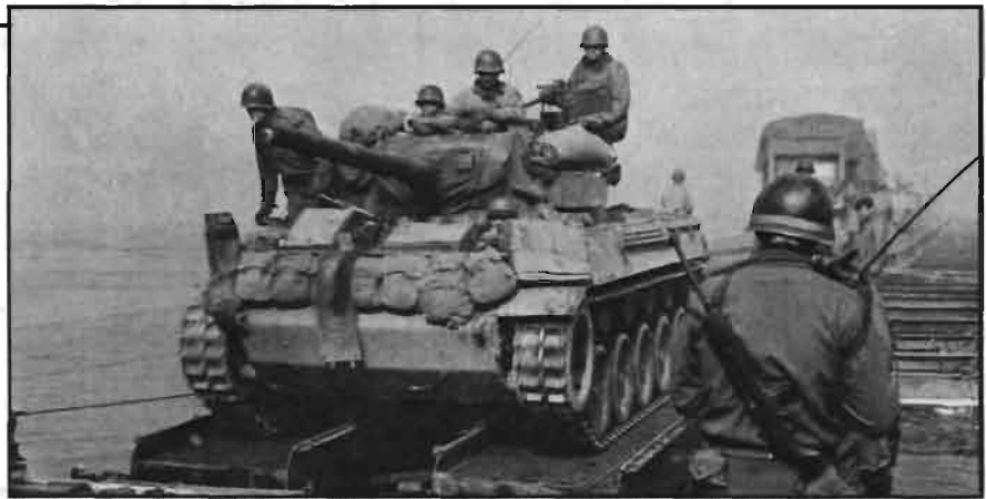
The M18 "Hellcat" Tank Destroyer, its suspension based on research done in the 1930s, was the first U.S. production vehicle to use torsion bar suspension. This one is seen crossing the Moselle River in 1945.
