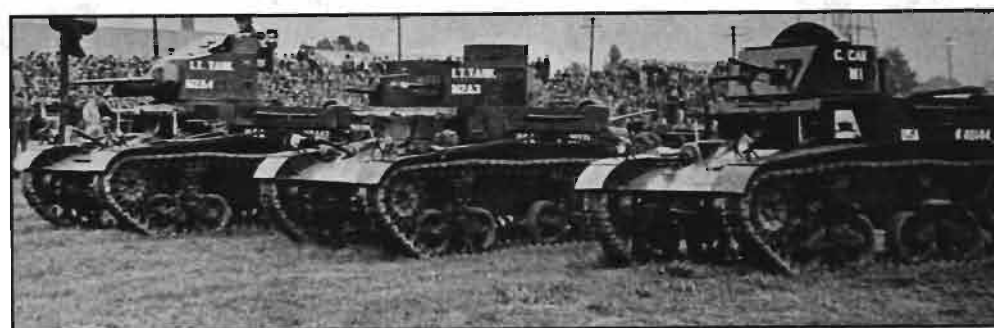
Three light tank designs at Aberdeen in 1940 included, from left, the 37-mm gun-armed M2A4, the twin-turreted, machine gun-armed M2A3, and the M1 Combat Car.
