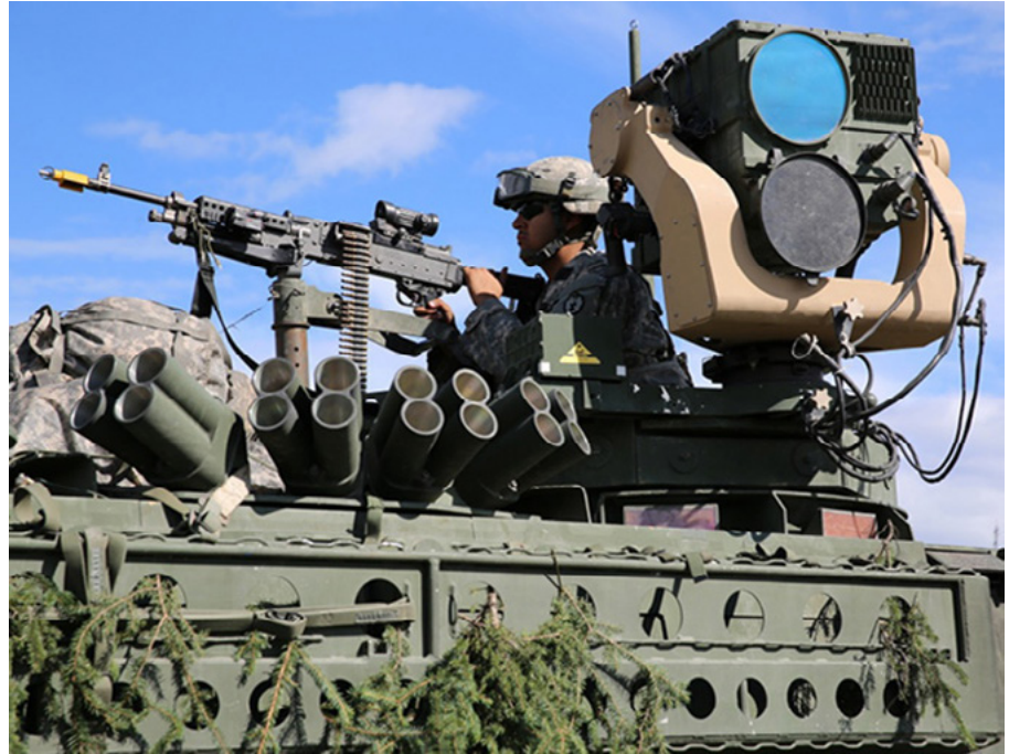
Figure 5. 196 th Infantry Brigade Stryker with APS. (U.S. Army photo by Rodney Jackson)
