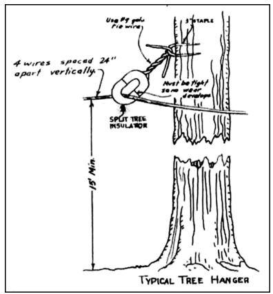
Figure 10. 1941 Diagram for Single-wire Telephone Line Construction
