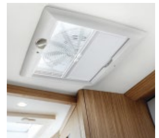
9403 Fresh air fan above kitchen
