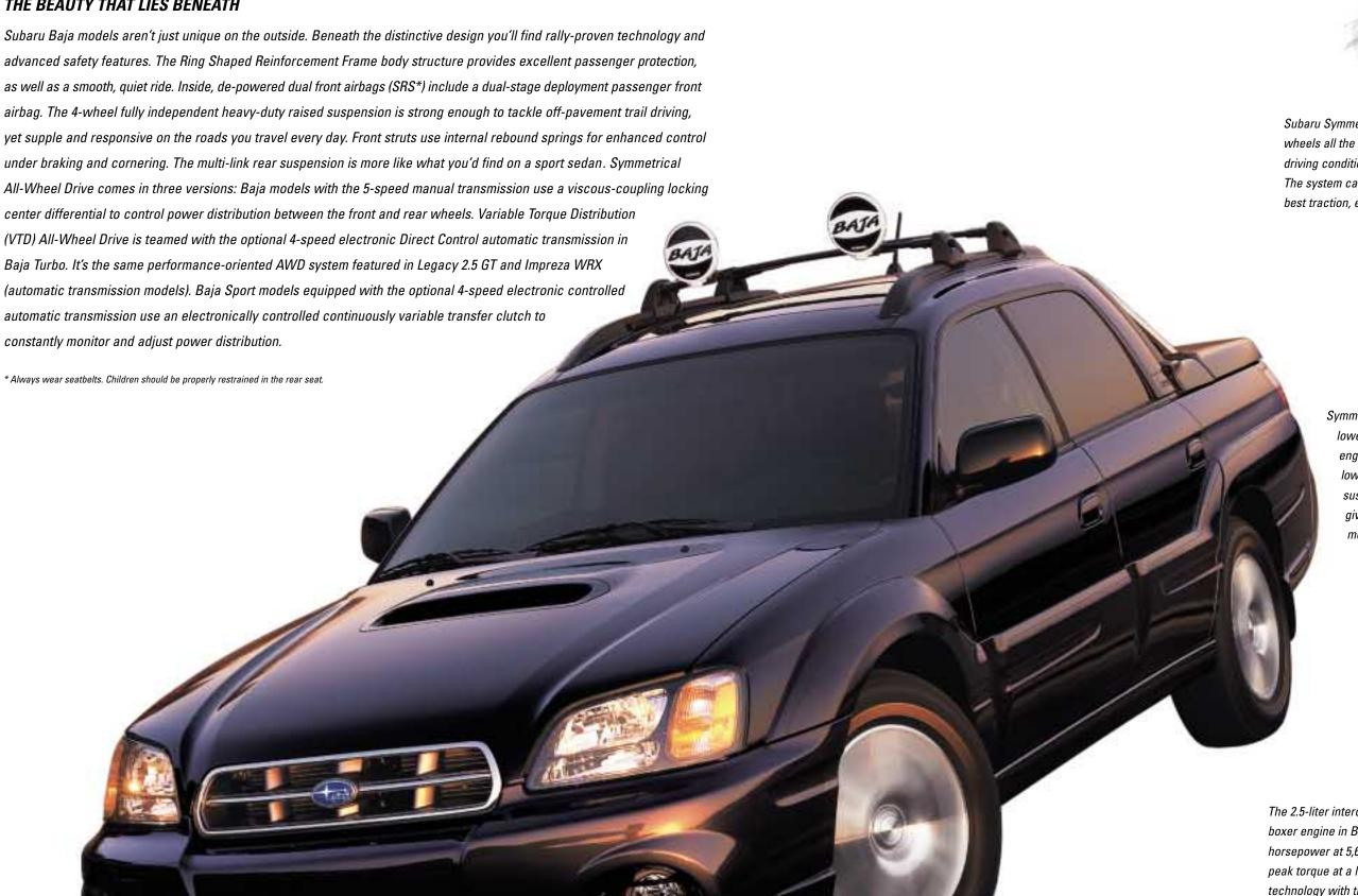
Subaru Symmetrical All-Wheel Drive powers all four wheels all the time, providing optimal traction for all driving conditions, from clear and dry to wet and slippery. The system can transfer power to the wheels with the best traction, enhancing handling and safety.
