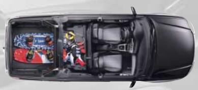
For maximum cargo space, you can drop the tailgate with the optional bed extender in place and lower the Switchback door for a cargo area over 90 inches long.
