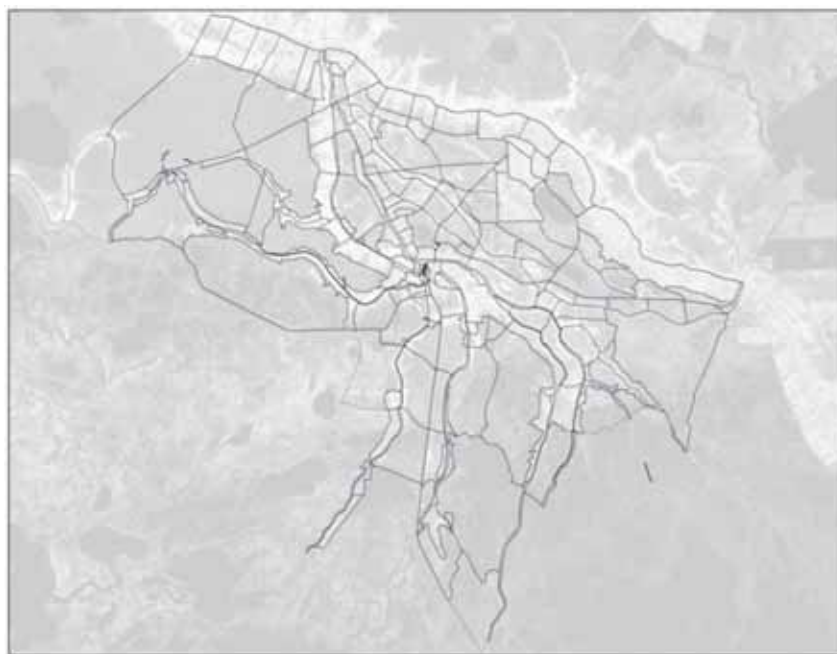
Figure 16 - Map of storage areas (HEC-FDA reaches) delineated for the interior hydrologic model
