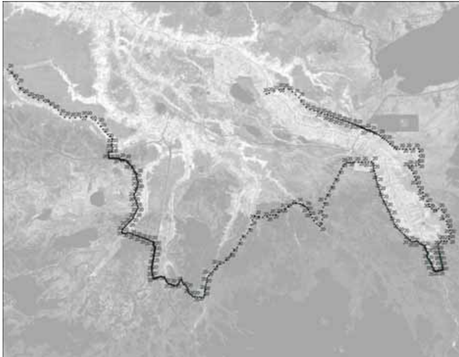
Figure 9 - With Project non-overlap levee alignment. Without project raised features are included in the with-project mesh. Elevations are in meters
