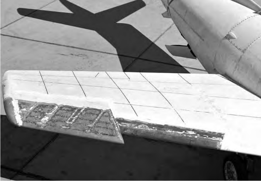
Leading-edge wing chord extensions tested on the third D-558-2 Skyrocket, one of many combinations of flaps, slats, fences, and extensions evaluated in the NACA's 6-year-long study of the Skyrocket's pitch-up behavior. NASA.
