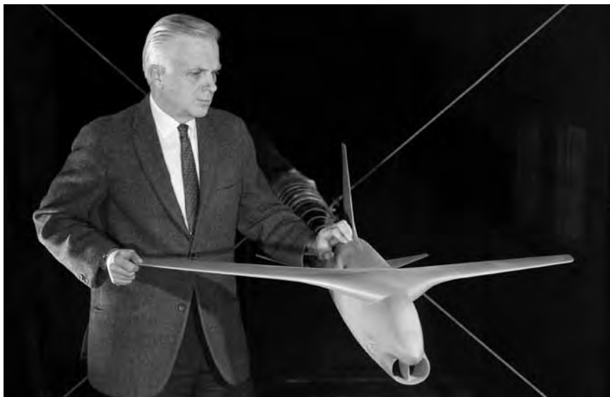
Whitcomb inspecting a supercritical wing model in the 8-Foot TPT. NASA.
