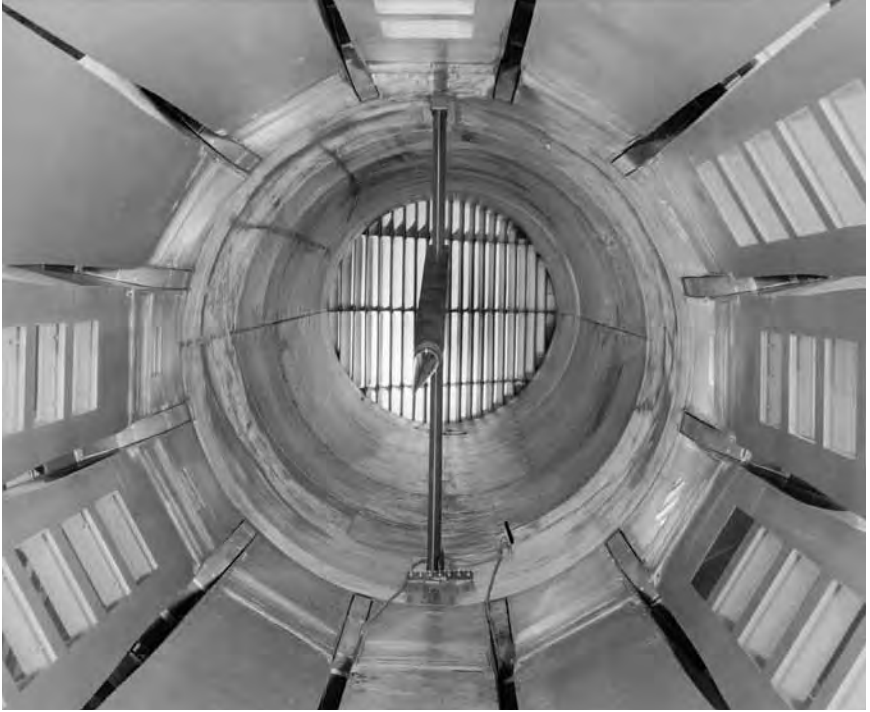
The slotted-throat test section of the 8-foot High-Speed Tunnel. NASA.
