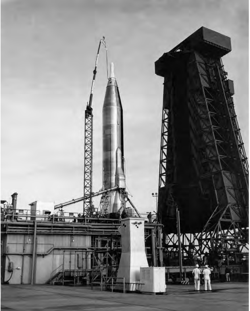
An Atlas ICBM with a low-drag ablatively cooled nose cone. USAF.
