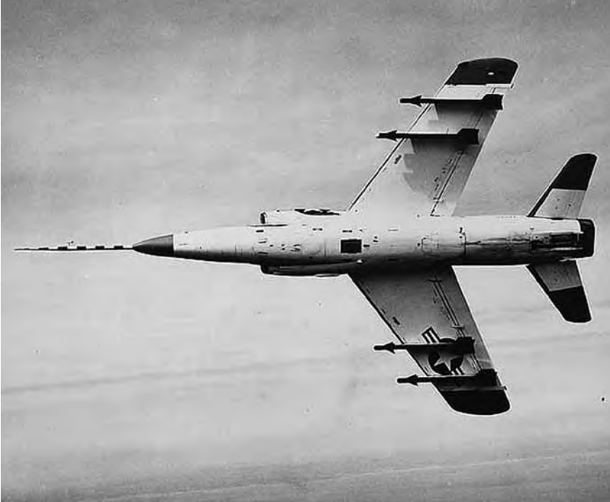
The area rule profile of the Grumman Tiger. National Air and Space Museum.
