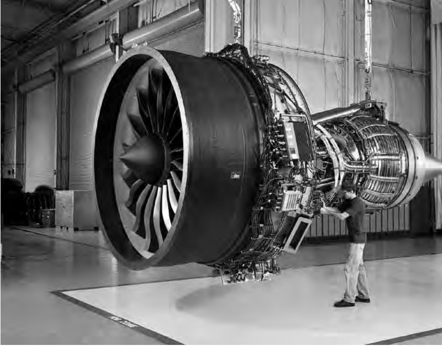
A General Electric GEnx engine with a composite damage-tolerant fan casing is checked out before eventual installation on the new Boeing 787. General Electric.
