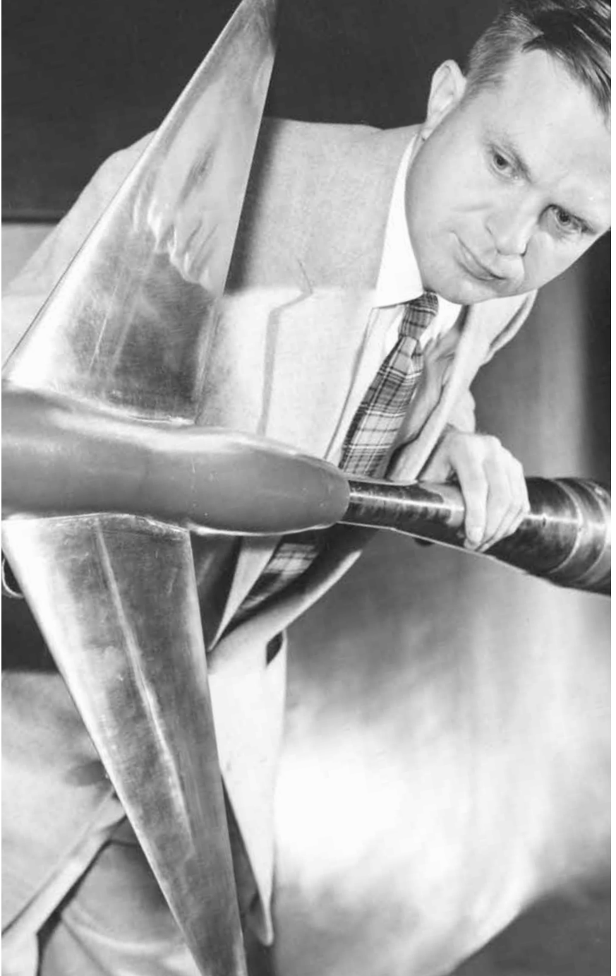
Whitcomb evaluates the shape of one of his area rule models in the 8-foot High Speed Tunnel. NASA.
