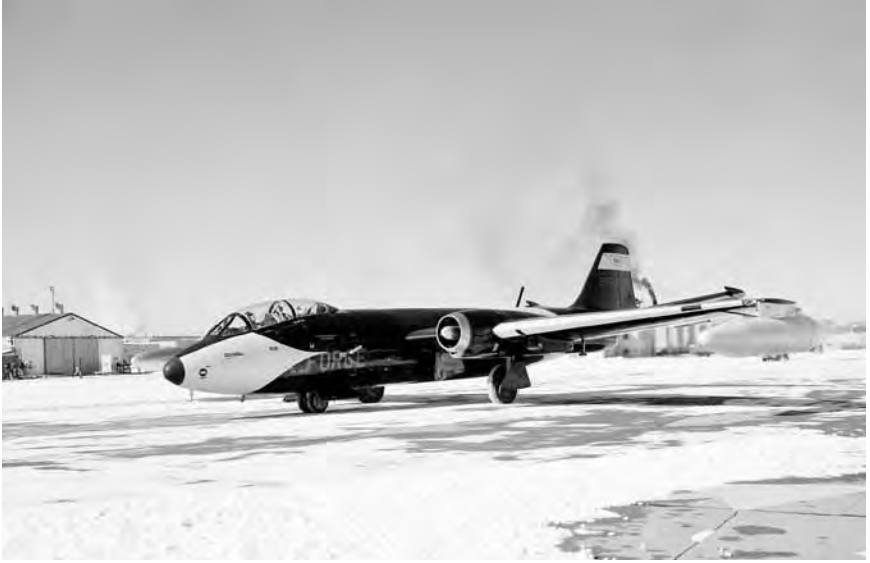
The Martin B-57B light bomber that Lewis modified to test hydrogen propulsion, shown on the snowy ramp of Lewis Laboratory (now Glenn Research Center) in 1958. NASA.
