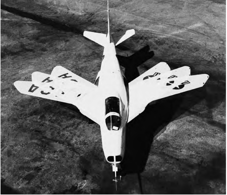
A time-lapse photograph of the Bell X-5, showing the range of its wing sweep. Note how the wing roots translated fore and aft to accommodate changes in center of lift with varying sweep angles. NASA.
