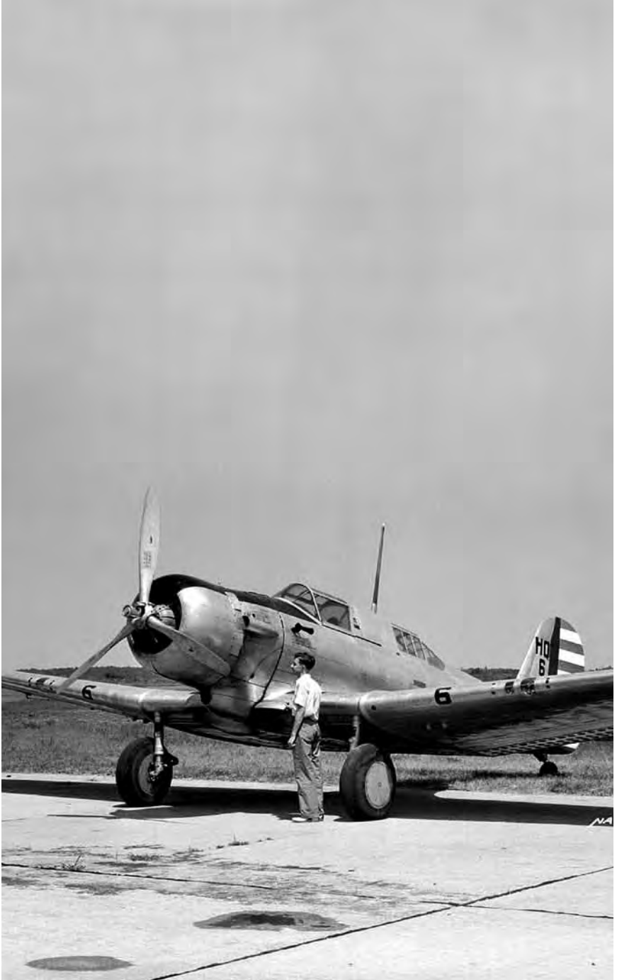
An NACA cowling on a Northrop A-17A at the Agency's Langley Laboratory in 1939. The NACA cowling was its signal contribution to integrating propulsive and aerodynamic design. NASA.
