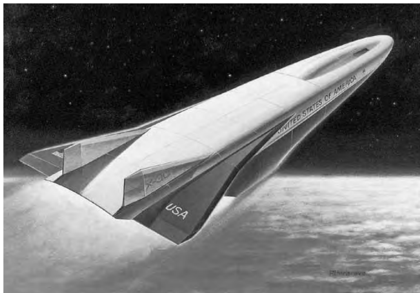
The National Aero-Space Plane concept in final form, showing its modified lifting body design approach. NASA.
