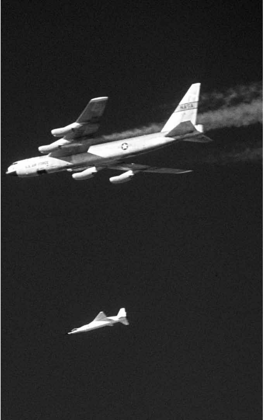
The X-43A Hyper-X test vehicle drops away from its Boeing NB-52B mother ship in November 2004, beginning its flight to Mach 9.7. NASA.
