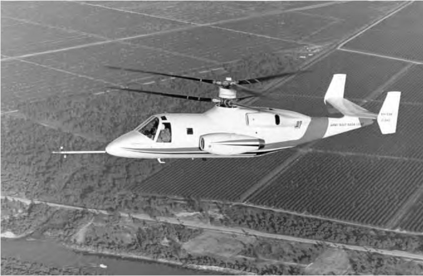
The Sikorsky XH-59A Advancing Blade Concept helicopter was a joint test program between the Army, Navy, NASA, and Air Force. NASA
