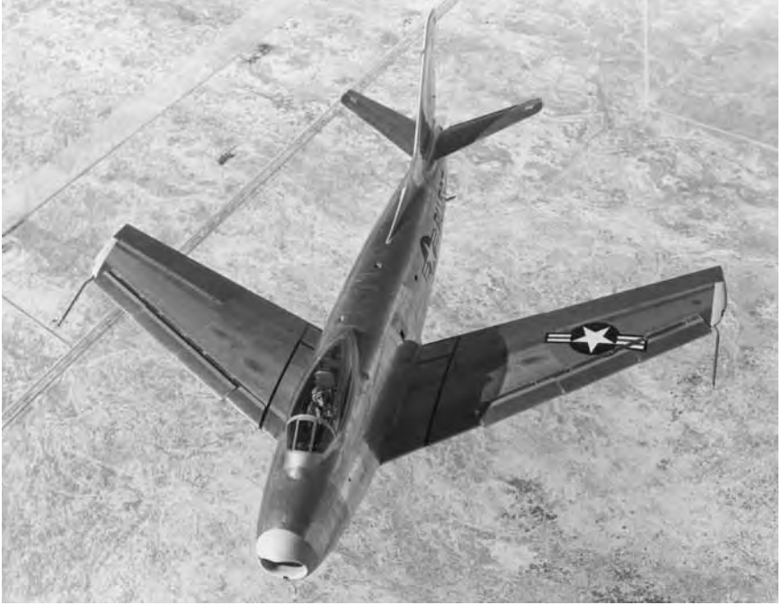
The North American XP-86, prototype of the F-86 Sabre family, represented an amalgam of German and American swept wing and streamlined aerodynamics. USAF.
