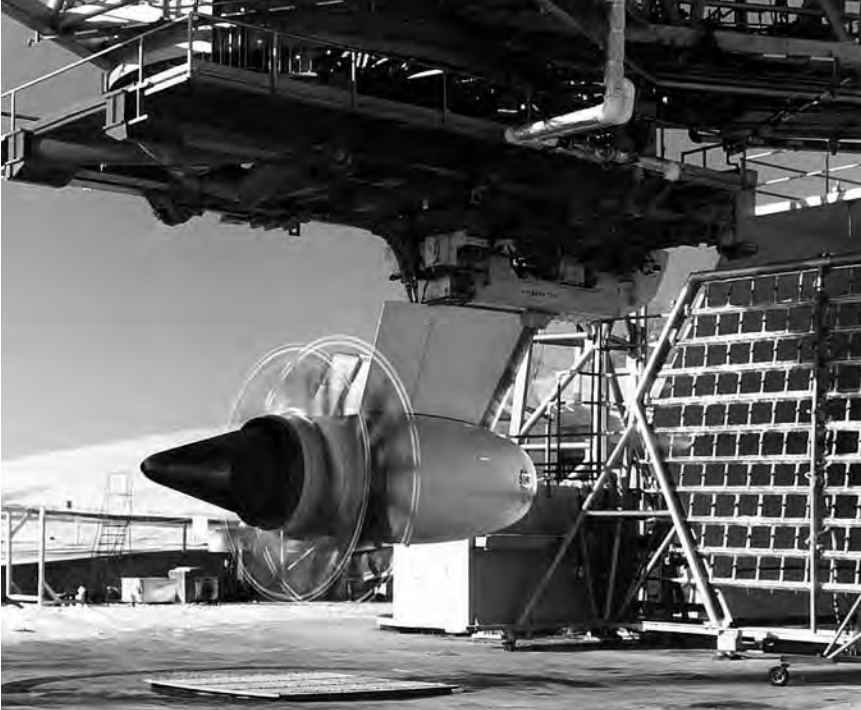
A General Electric design for an Unducted Fan engine is tested during the early 1980s. General Electric.
