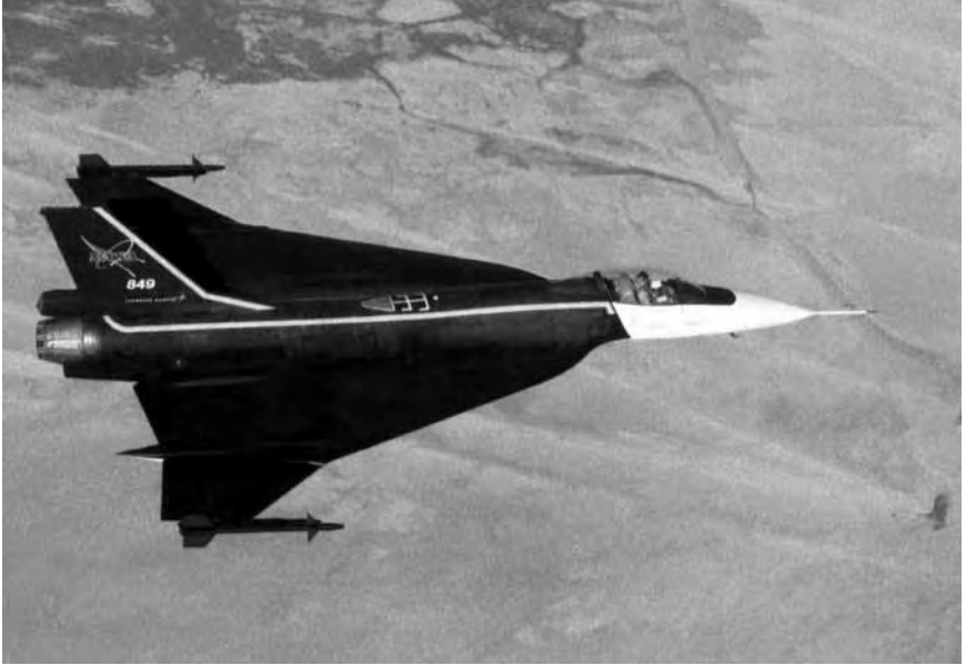
The NASA F-16XL cranked-arrow research aircraft aloft over the Dryden Flight Research Center on December 16, 1997. NASA.
