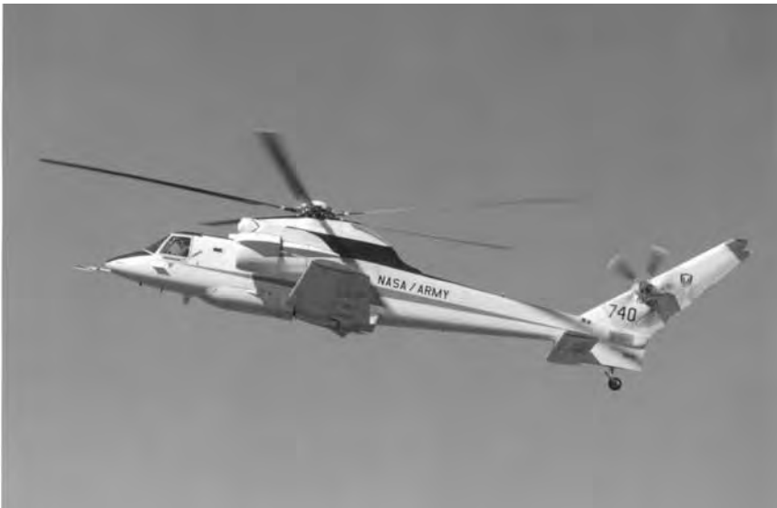
The NASA–Army Sikorsky S-72 Rotor Systems Research Aircraft in flight at NASA's Ames Research Center. NASA.
