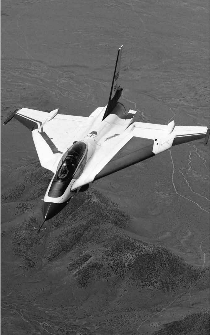
The F-16XL-2 was one of two test aircraft that NASA Dryden used in the 1990s to test the application of laminar flow at supersonic speeds. NASA.
