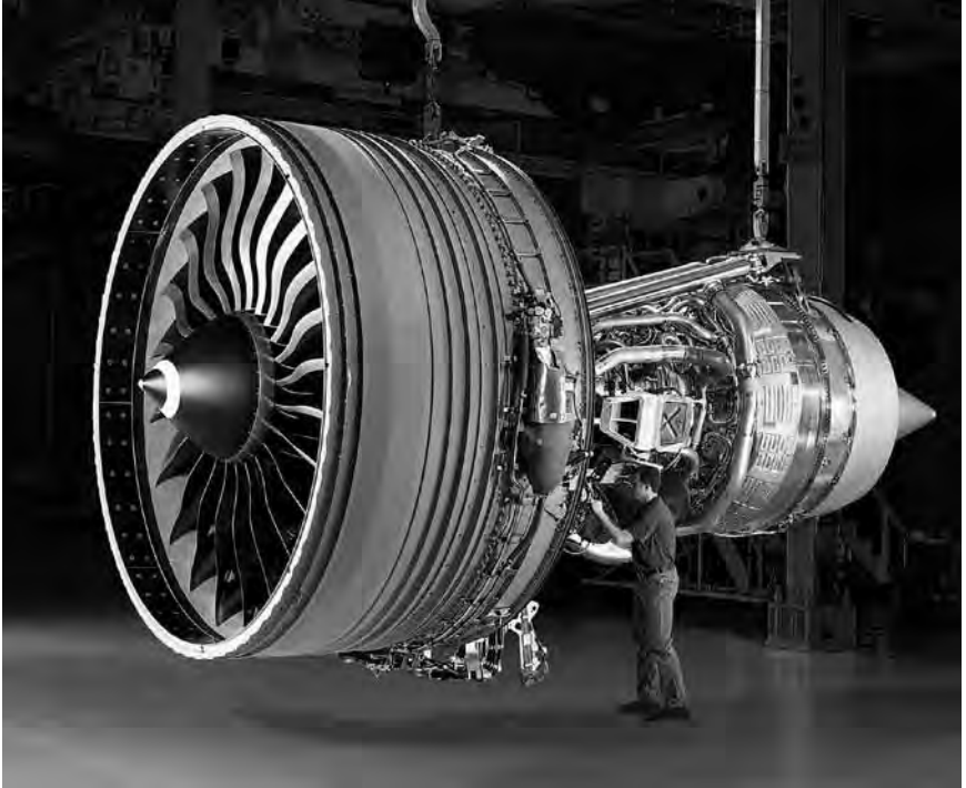
The giant General Electric GE90 jet engine that powers the Boeing 777 benefited from the Energy Efficient Engine project. General Electric.
