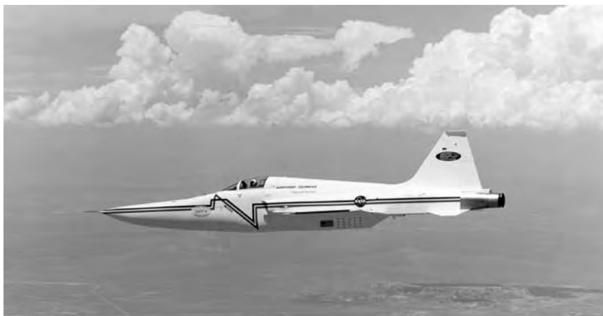
Close-up view of the SSBD F-5E, showing its enlarged "pelican" nose and lower fuselage designed to shape the shock waves from the front of the airframe. NASA.
