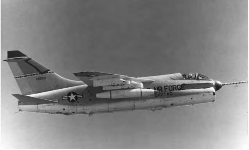
The Ling-Temco-Vought A-7D DIGITAC testbed was the first U.S. Air Force airplane with a digital flight control system. USAF.
