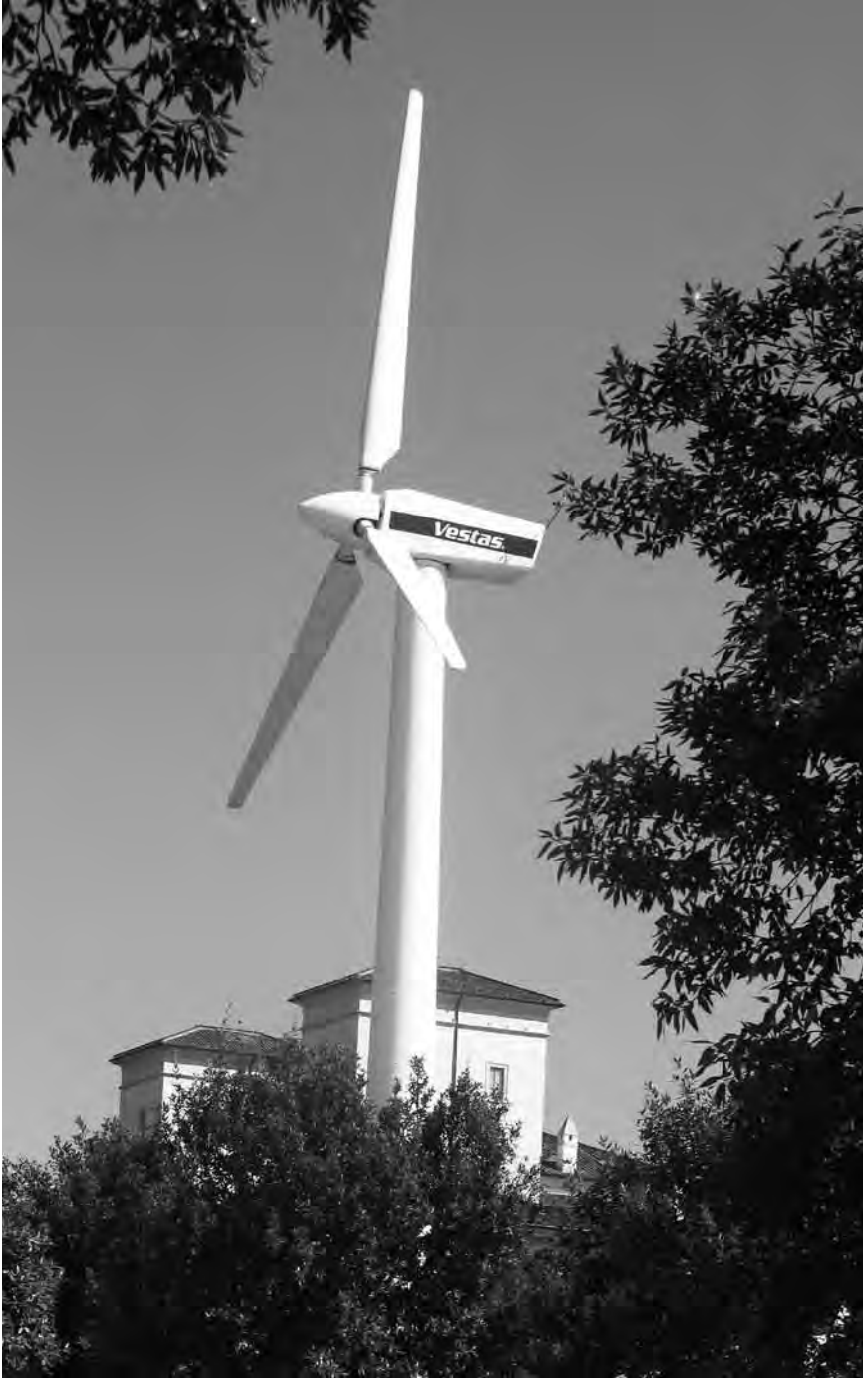
A full-pitch, fiberglass Vestas wind turbine in Rome in 2009. The Danish company remains the largest in the wind turbine industry. R.P. Hallion.
