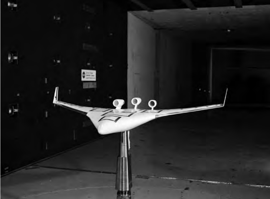
A 3-percent scale model of the Boeing Blended Wing Body 450 passenger subsonic transport in the Langley 14 x 22 Subsonic Tunnel. NASA.
