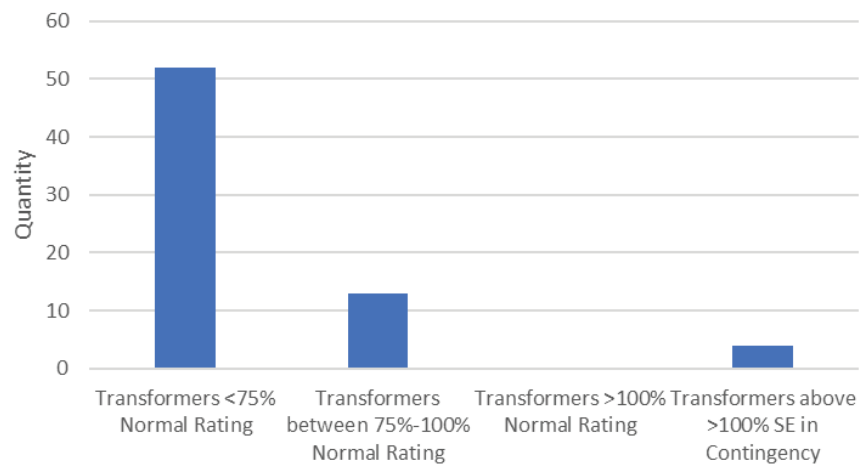
Exhibit 4.100: South Shore sub-region 2023 Forecasted Transformer Loading Profile
