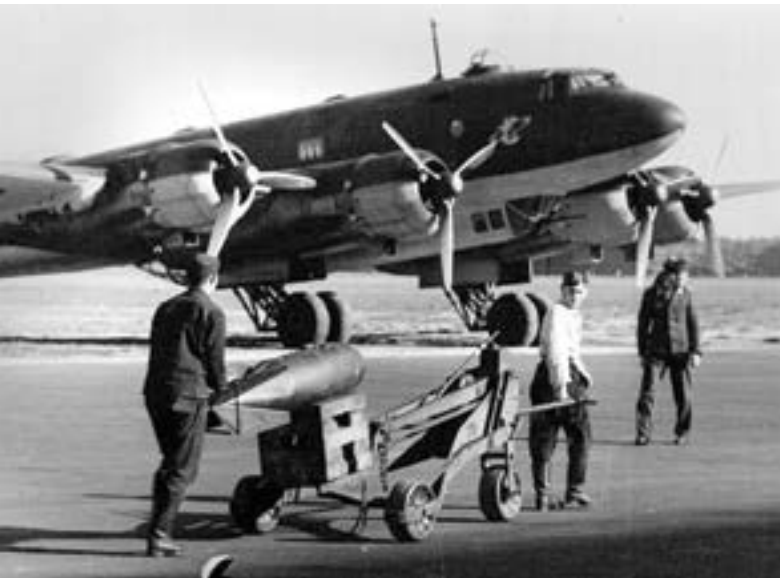
An SC250 fragmentation bomb load being prepared for an Fw 200 Condor of KG 40.
