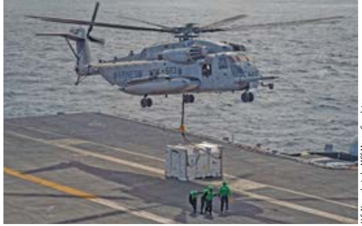
A Marine Corps CH-53E Super Stallion, with Marine Heavy Helicopter Squadron (HMH) 466, transports a mock F135 engine power module.
