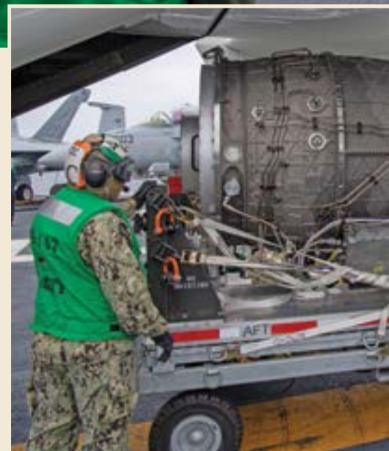
Sailors assigned to the “Argonauts” of Strike Fighter Squadron (VFA) 147 load an F-35C Lightning II power module onto a CMV-22B Osprey assigned to the “Titans” of Fleet Logistics Multi-Mission Squadron (VRM) 30 on the flight deck of aircraft carrier USS Carl Vinson (CVN 70).
