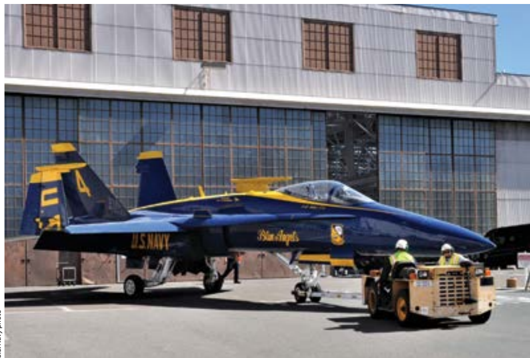
A former Blue Angels Legacy F/A-18C Hornet is towed to the Fleet Readiness Center Southwest test line where its hydraulic fuel will be drained as part of the demilitarization process in preparation for its conversion to a pedestaled display in the courtyard of Commander, Naval Air Forces.
