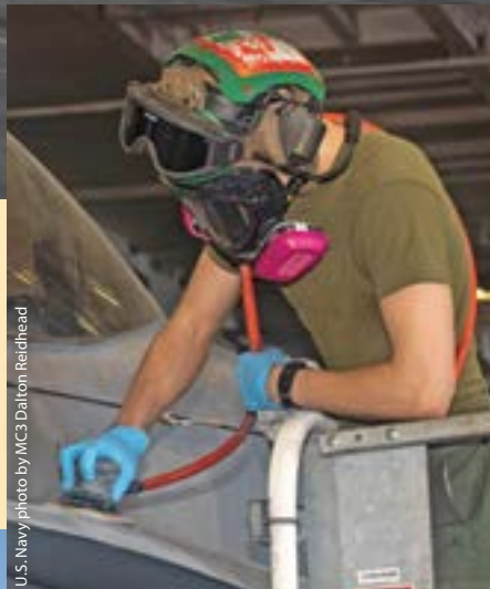
Lance Cpl. Warren Martineaulii, assigned to VMFA-323, sands nonskid off of an F/A-18C Hornet in the hangar bay aboard Nimitz.
