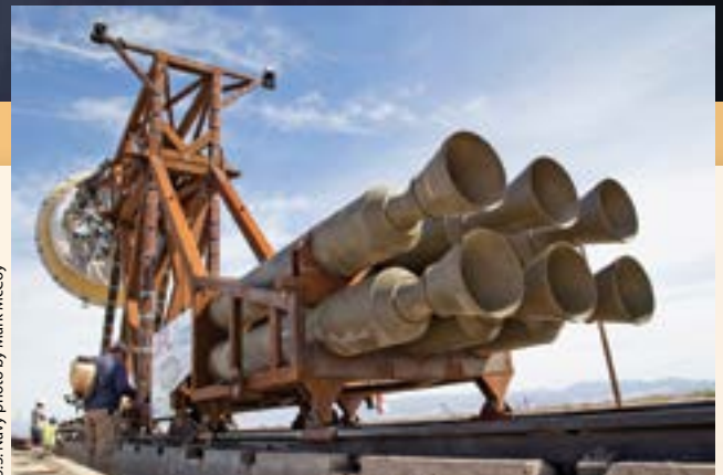
The SIAD design verification tests required a sled powered by six Nike rocket motors, seen here in April 2014.
