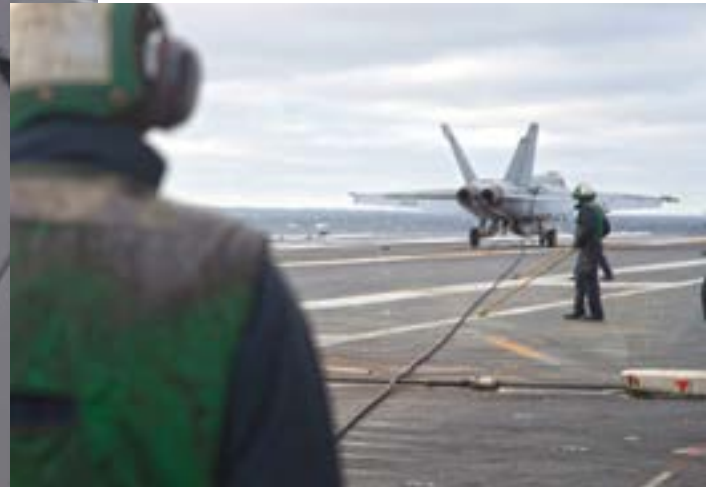
AVFA-106 F/A-18F lands on Ford's flight deck using the Precision Landing Mode.
