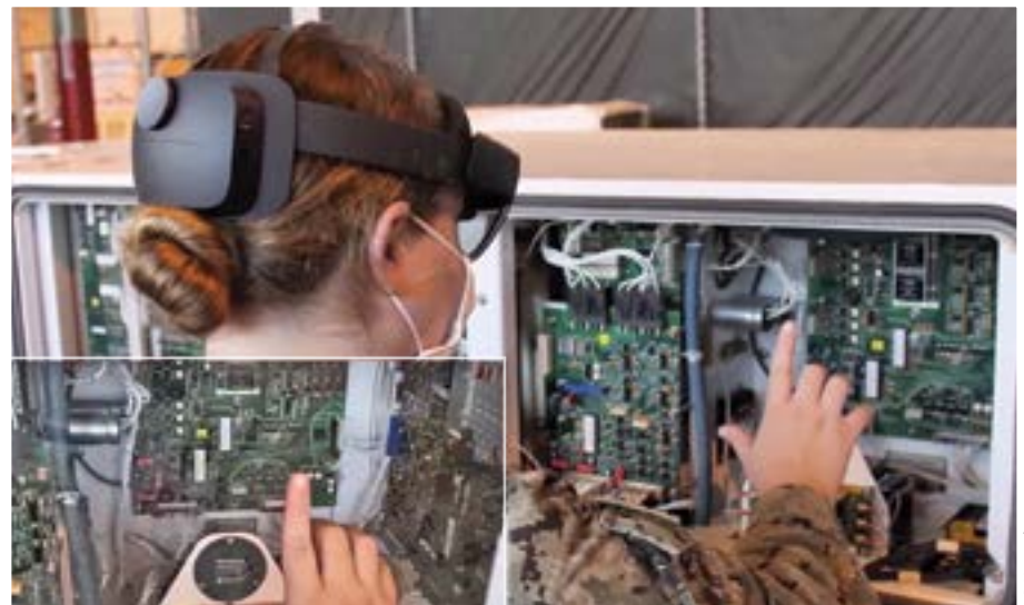
Petty Officer Hailey Wilmoth is using ARRMSS to communicate with a remote expert and capture a photo during Static Frequency Converter troubleshooting at Naval Air Station Patuxent River to send to the expert.
