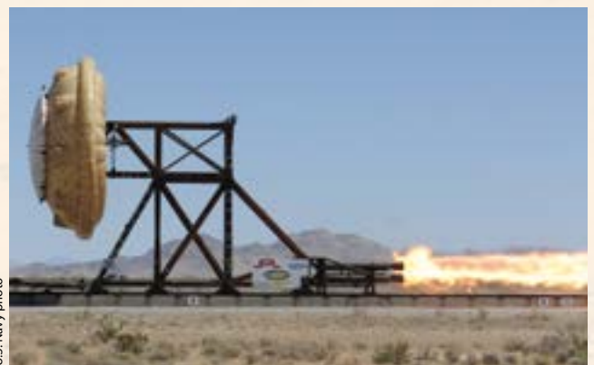
The shuttlecock-shaped SIAD rockets down NAWCWD’s Supersonic Naval Ordnance Track during a 2015 test.
