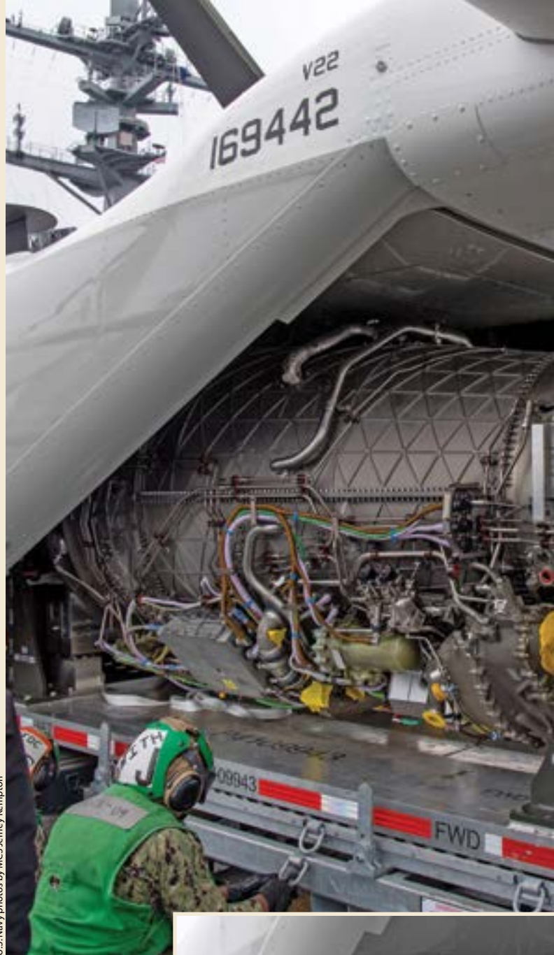
Sailors finish loading an F-35C power module into the CMV-22B.
