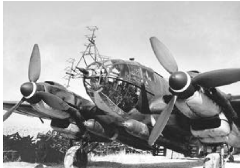
A torpedo-carrying Heinkel He 111H-18 with FuG 200 'Hohentwiel' ship-search radar.
