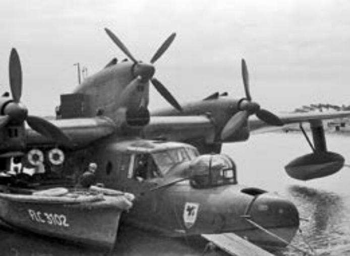
A Blohm und Voss Bv 138 is prepared with depth charges for an anti-submarine mission over the Black Sea. The tender at left was locally commandeered for Luftwaffe service.
