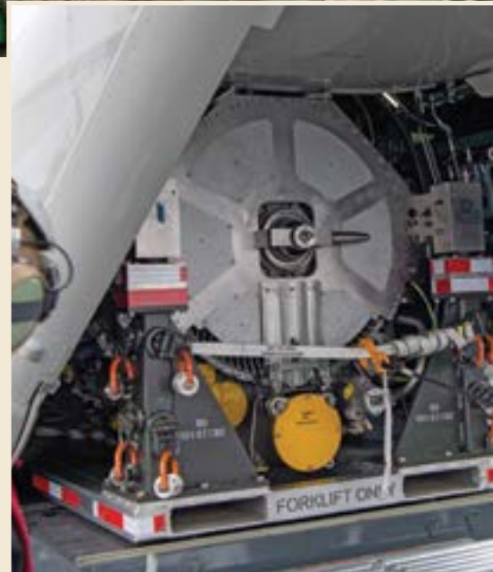
Sailors finish loading an F-35C power module into the CMV-22B.
