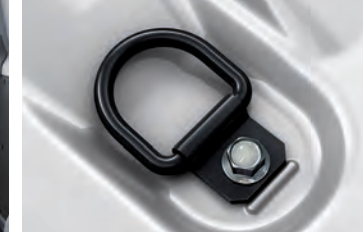
Six floor-mounted 2 and six wall-mounted D-ring tie-downs!
