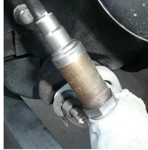
Ox Sensors right and left for Air/fuel ratio gauge.
