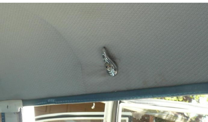
Installed right and left coat hooks above the rear doors.
