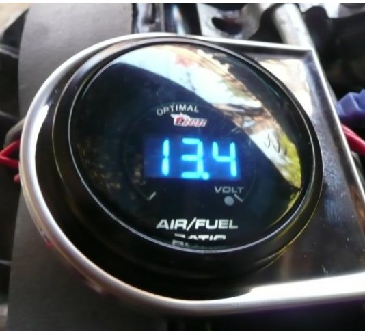
Air/Fuel ratio gauge with r/l selector switch.
