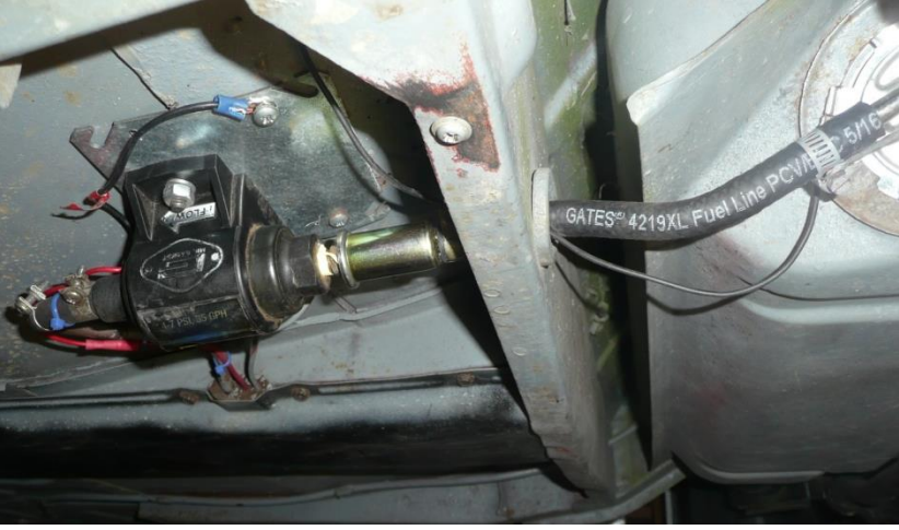
Relocated and rewired the electric fuel pump. This is required for the 140 engine. The fuel pump came with the wagon.
