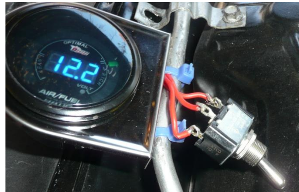
Air/Fuel ratio gauge with r/l selector switch.
