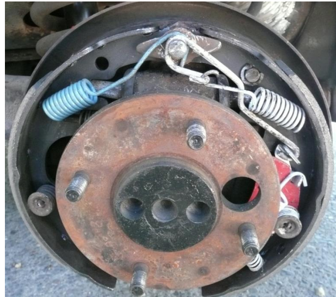
Left rear with self adjusters and new brake shoes
