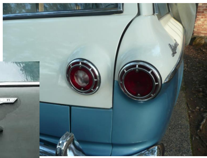
Added a 140 insignia to the tailgate in prep for new engine. This location is consistent with the cross flags of the 102 HP insignia location. Installed 1962 Backup light lenses.
