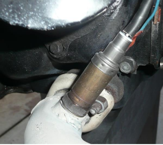
Ox Sensors right and left for Air/fuel ratio gauge.
