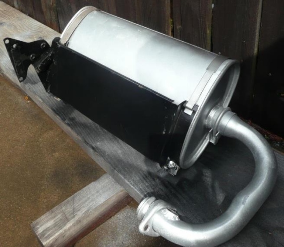
Factory 140 mufflers with heat shield
