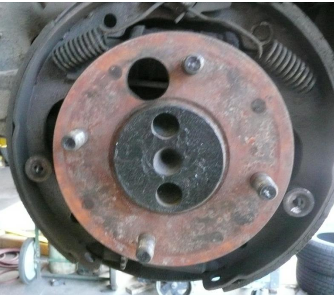
Left rear brake assembly no self adjusters
