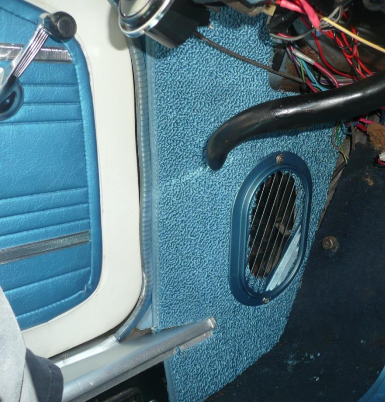
Installed Carpet on kick panels and painted vent grills blue.
