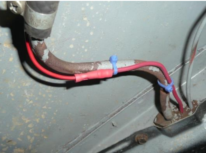
Relocated and rewired the electric fuel pump. This is required for the 140 engine. The fuel pump came with the wagon.
