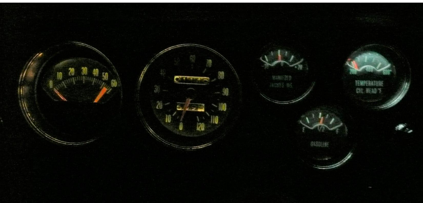
Installed "Super Bright LED lamps" in Spyder instrument panel Zeroed the Tack pointer
