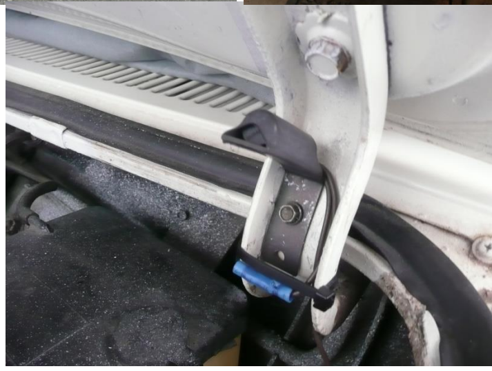
Trunk light with mercury switch
