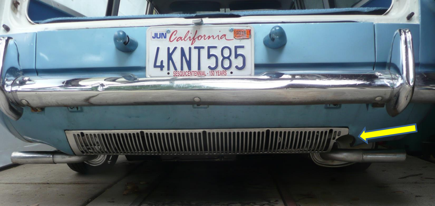
Final Tailpipe location after crossover pipe is installed.
