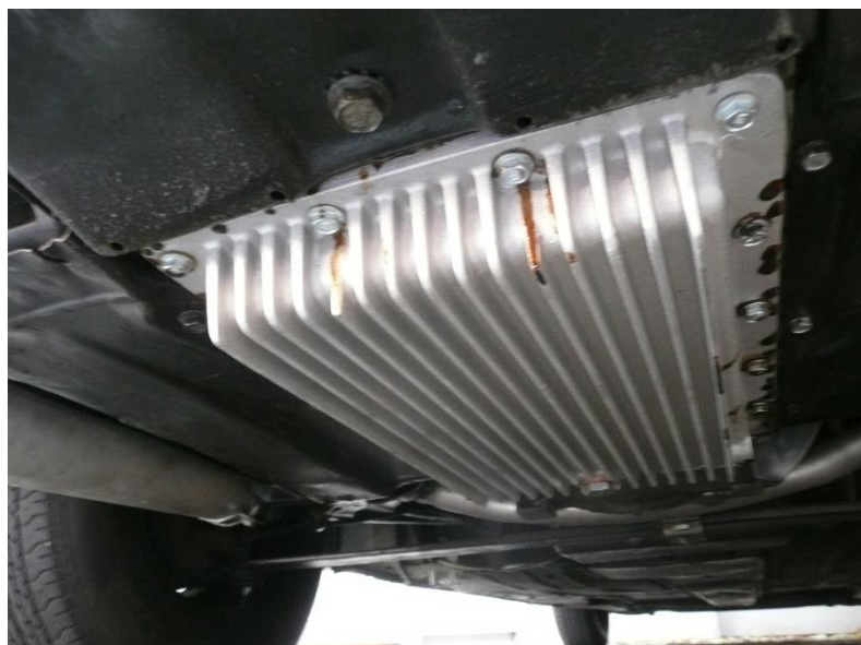
Aluminum Oil Pan 1 qt additional oil
