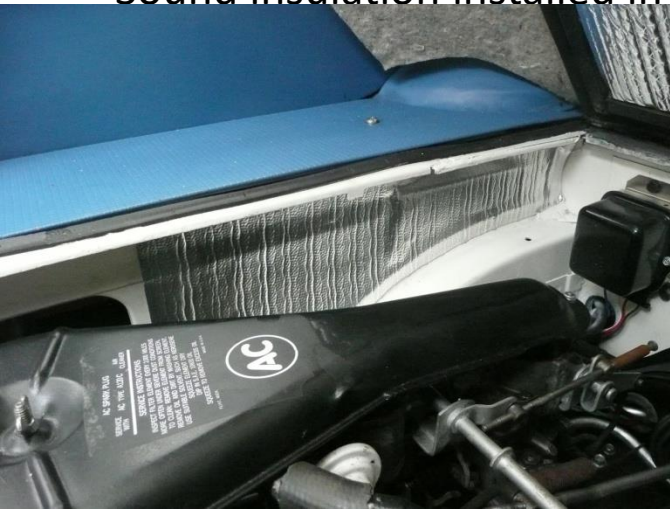
Sound insulation installed in engine compartment
