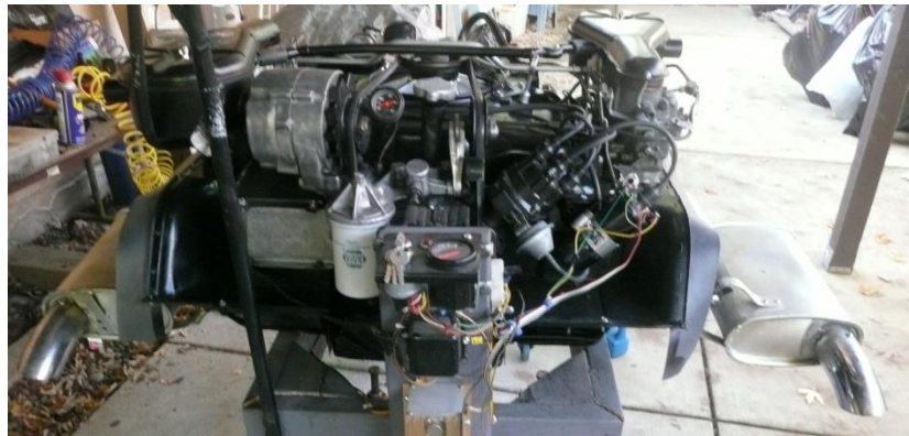
Dual exhaust with crossover pipe.
