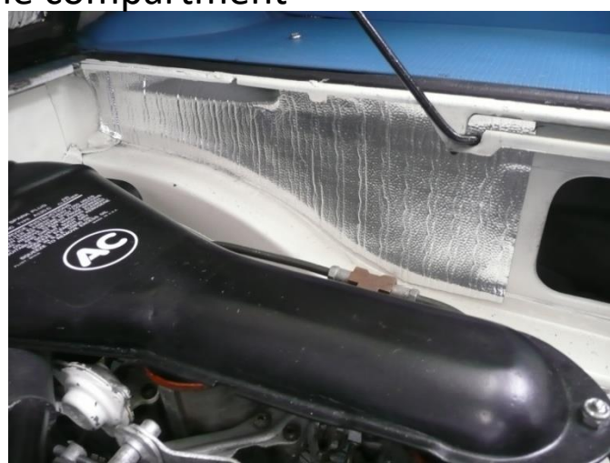
Sound insulation installed in engine compartment
