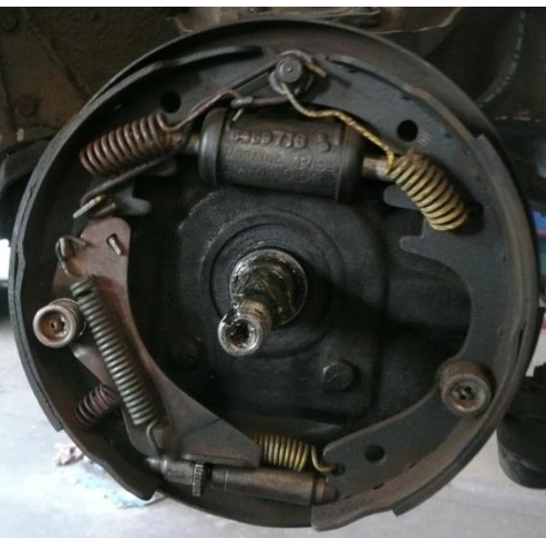
Left and Right brake assemblies with 64 backing plates and self adjusting brakes now on all four wheels.
