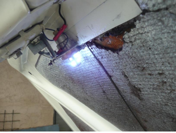
Trunk light with mercury switch
