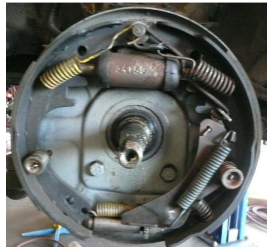
Left and Right brake assemblies with 64 backing plates and self adjusting brakes now on all four wheels.
