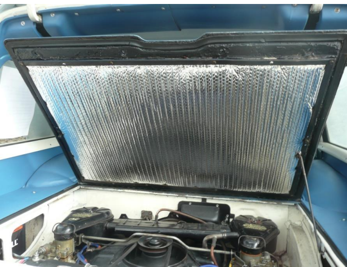
Engine hatch insulation
