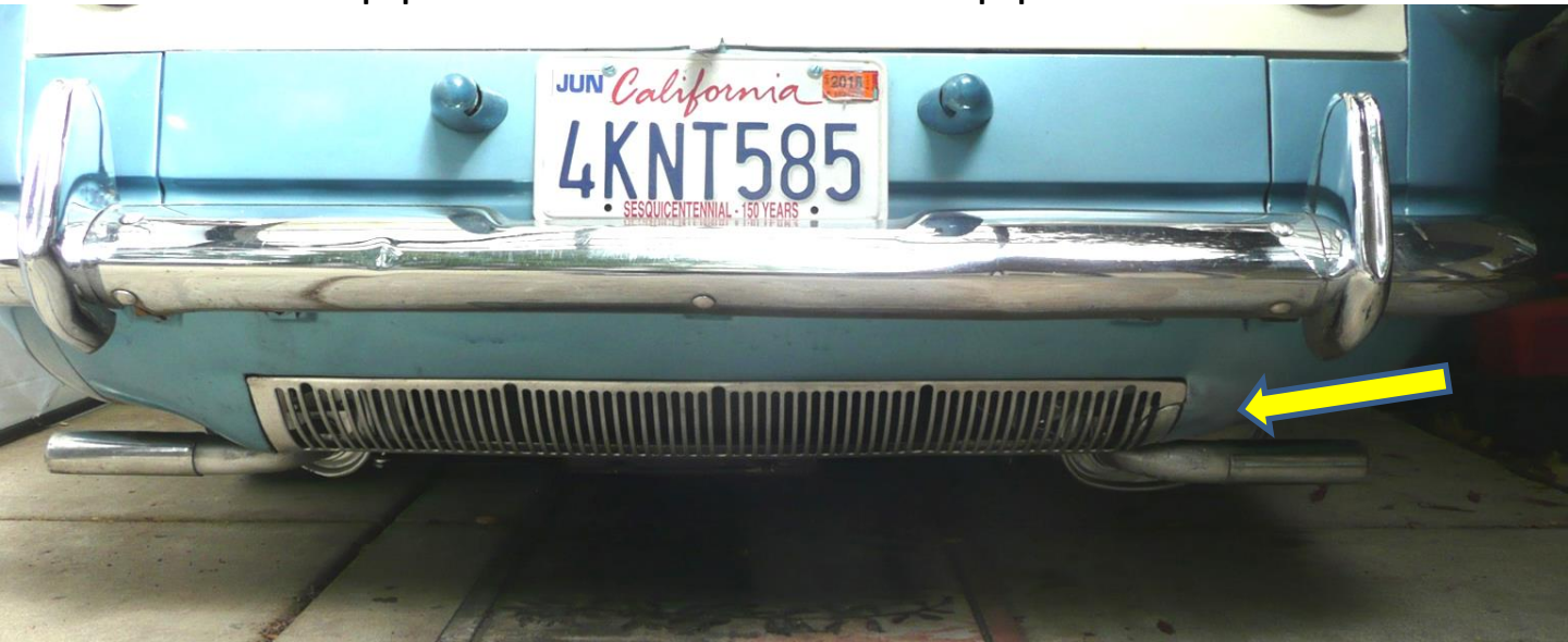
Final Tailpipe location after crossover pipe is installed.
