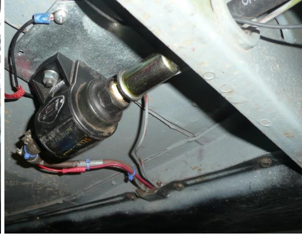
Relocated and rewired the electric fuel pump. This is required for the 140 engine. The fuel pump came with the wagon.
