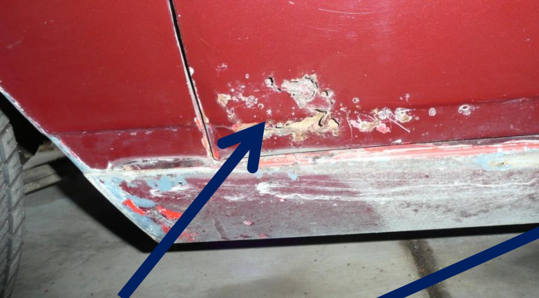
Left front Door Rust Repair
