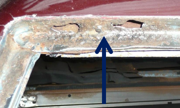
Front Windshield Rust Repair Top right
