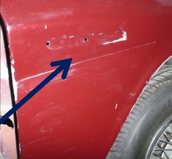
Right front fender need dent Repair
