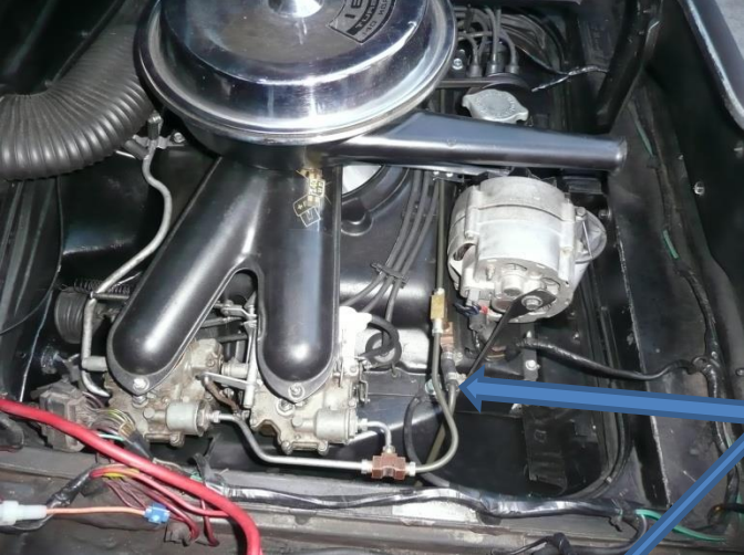
Engine compartment cleaned painted and new bolts were installed to hold down the shrouds
