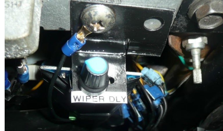
Windshield wiper delay 3 to 30 seconds, mounted to the right of the Hazard switch
