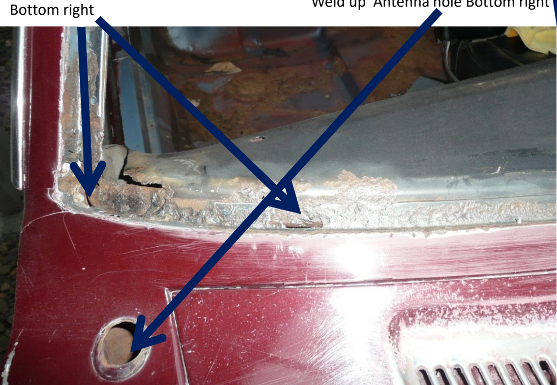
Weld up Antenna hole Bottom right
