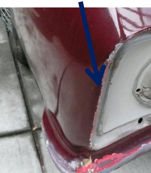
Left rear fender Dent Repair
