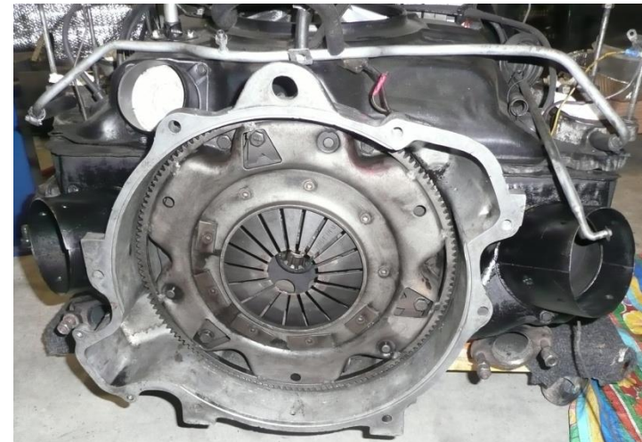
Engine removal and clutch and bell housing removal. Replaced bell housing seal. Cleaned and painted shrouds and tunnel covers.
