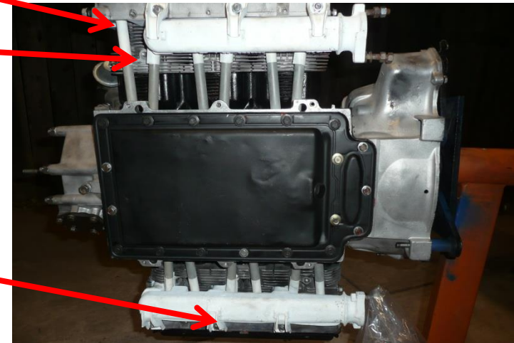
Exhaust Manifold heat shields self fabricated
