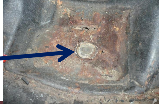
Trunk Bottom To be cut out and a new bottom (supplied) to be welded in.
