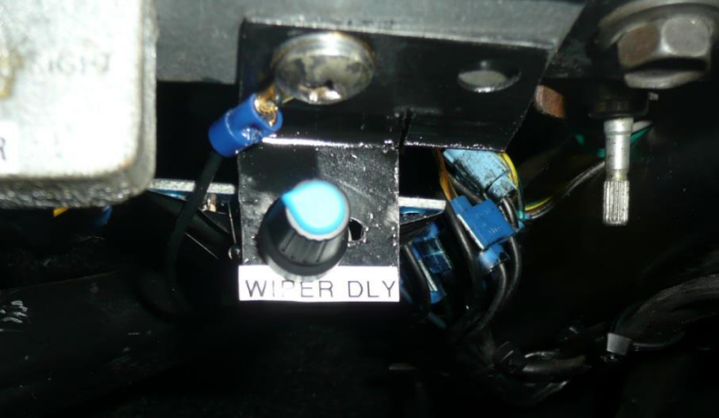
Windshield wiper delay 3 to 30 seconds, mounted to the right of the Hazard switch
