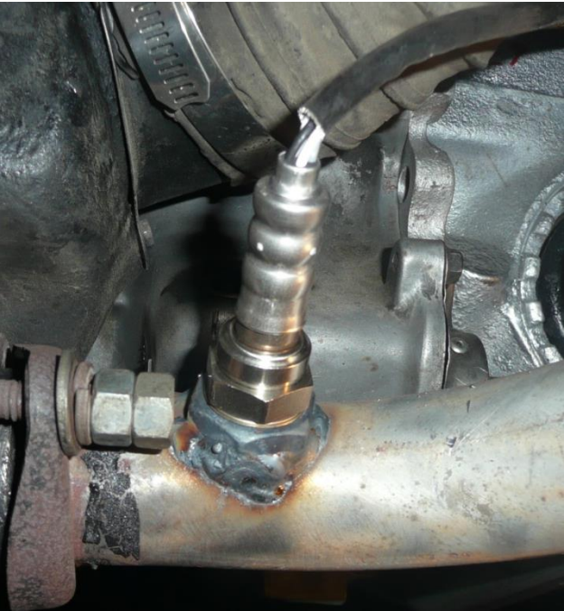
O2 Sensor at head of right exhaust pipe
