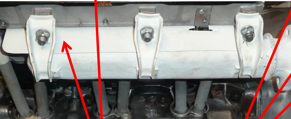
Exhaust Manifold heat shields, self fabricated
