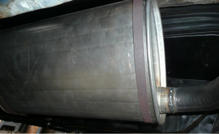
Drivers side muffler after installation.
