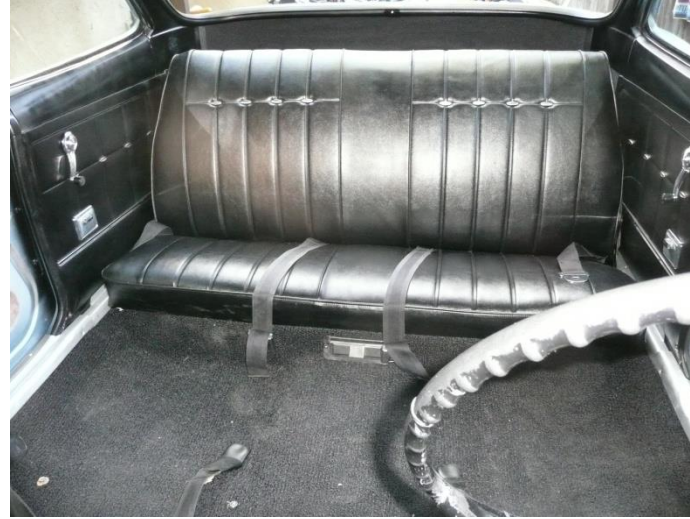
Progress 12: installed rear package shelf, rear seat and front and rear carpet and all seat belts.
