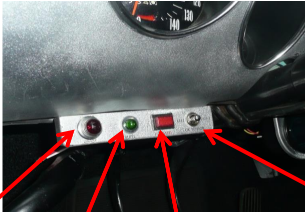
Emergency Brake Cruise Emergency Flashers Side select for fuel ratio Gauge
