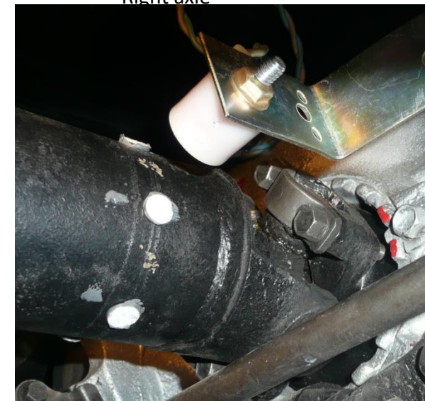
Road Speed pickup coil Right axle
