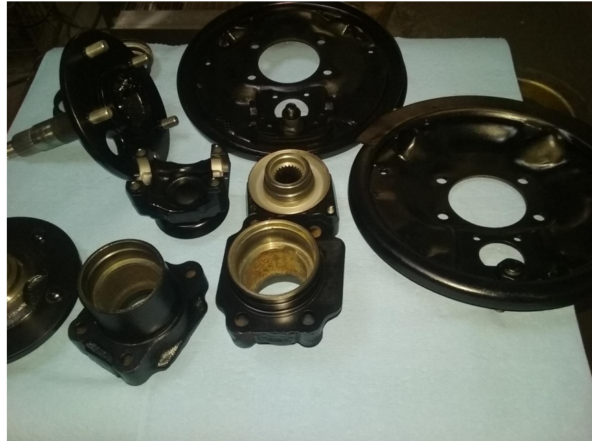
Rear hubs prepped and painted and ready for assembly.
