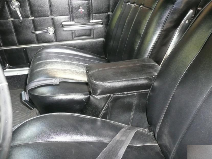
One of a kind center console. Made from material salvaged from the old seats and some scrap carpet material.
