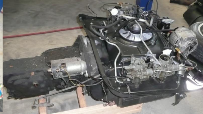
Engine removal and clutch and bell housing removal. Replaced bell housing seal. Cleaned and painted shrouds and tunnel covers.
