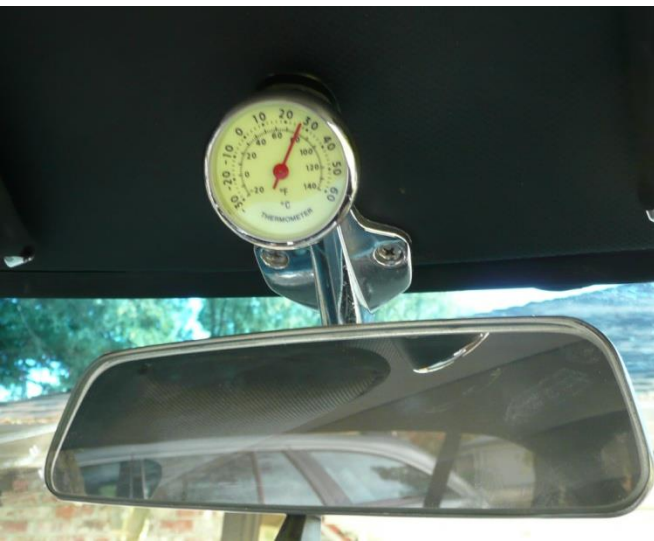
Mounted a thermometer on the end of the mirror mount.
