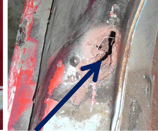
Left front Door Sill Rust Repair
