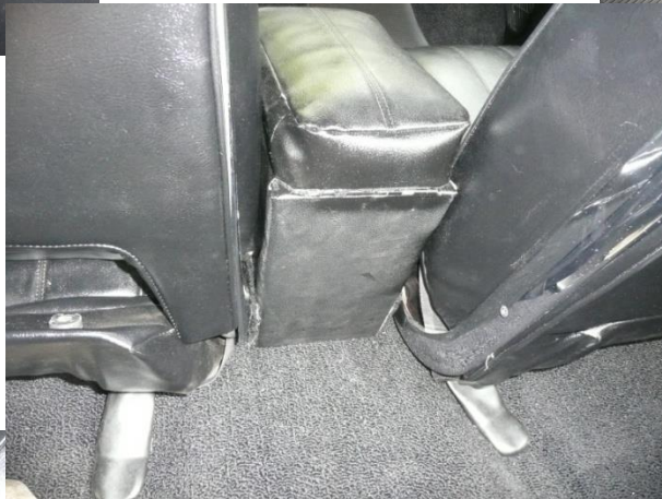
One of a kind center console. Made from material salvaged from the old seats and some scrap carpet material.
