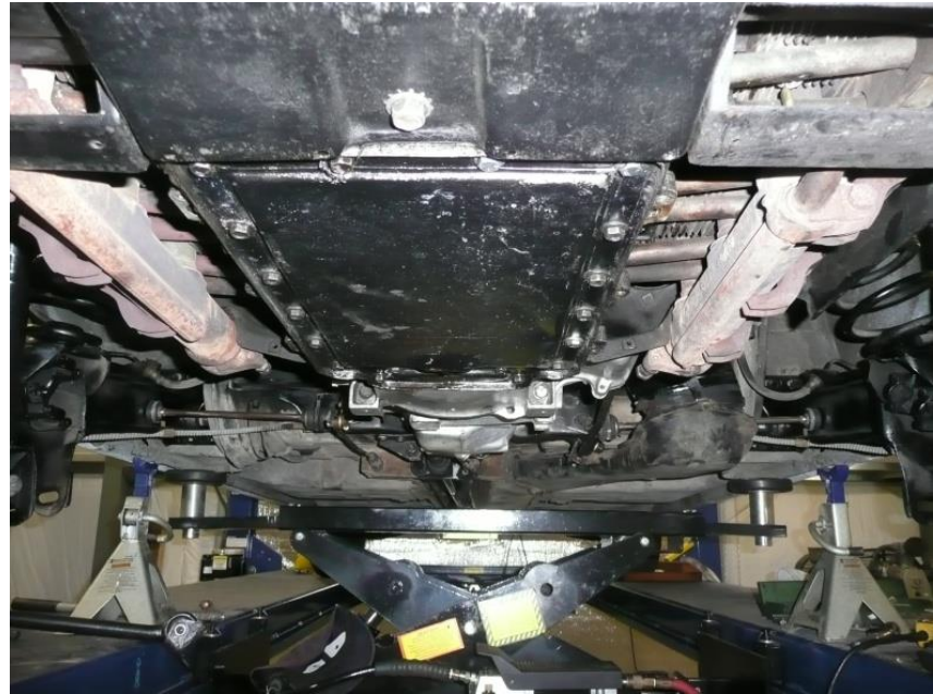
Original engine installation with 3.27 transaxle .
