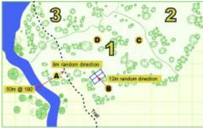
Figure 16. Initial steps of plot location.
