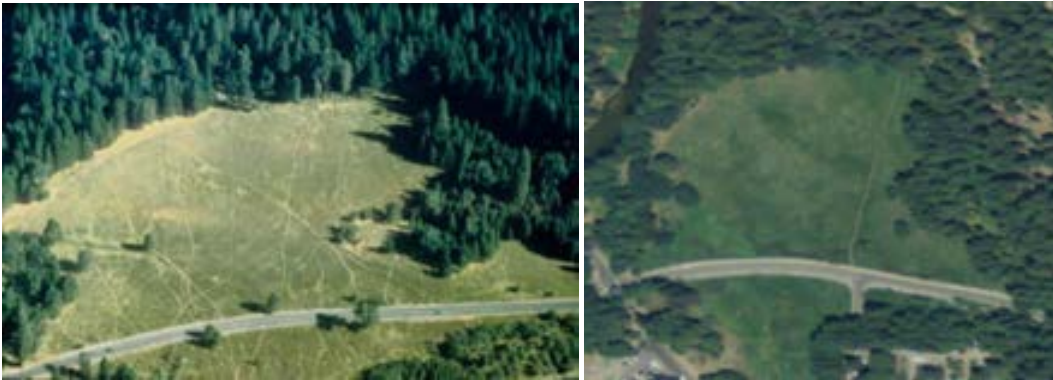
Figure 1: The park has successfully removed networks of informal trailing in meadows. In this example before (left) and after (right) restoration of Stoneman Meadow, high visitor use was mitigated by adding fencing to direct people to a new boardwalk, which allowed access to the meadow without the associated impacts.
