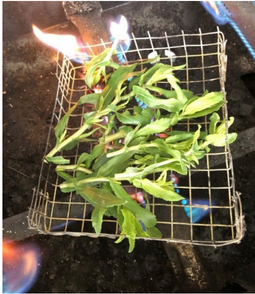
Figure 9. Curlycup gumweed had the longest time to ignition (TI) for each month except September. Photo shows material collected in June. Photo by Derek Tilley.
