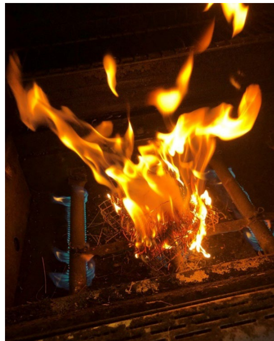
Figure 11. A 12 g sample of cheatgrass harvested in mid-September ignites quickly and burns explosively. Photo by Derek Tilley.
