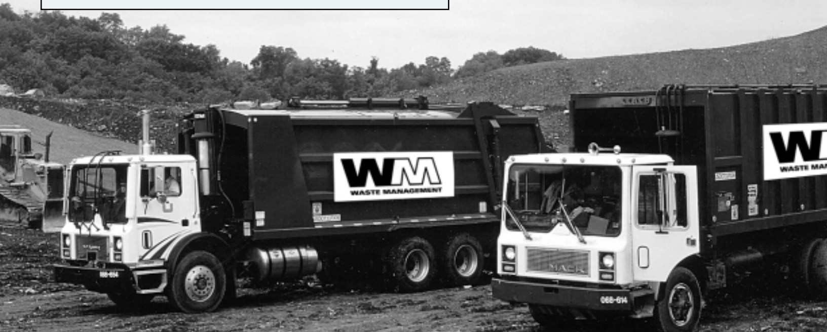
Waste Management uses Mack MR refuse haulers with the E7G 325-hp LNG engine (left) and the E7 300-hp diesel engine (right).
