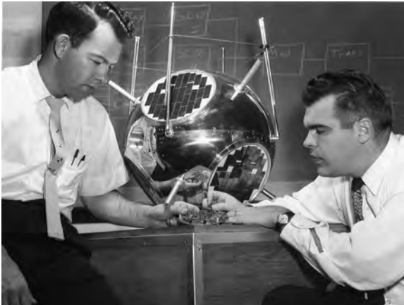
STB Bosses. Marty Votaw (left) and Ed Dix, who succeeded Votaw in 1963 to become the second head of NRL's Satellite Techniques Branch, work on SOLRAD 3. The same spherical shell carried an unclassified payload for studying solar X-rays and a classified one, GRAB 2, for spying on Soviet electronic signals emanating primarily from radar systems. (NRL photo 60383.jpg)
