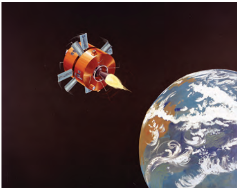
Solrad Hi. Artist's rendition of the two-payload SOLRAD 11 mission at a point when the perigee kick motor is firing to bring the payloads to a higher orbit. Also known as SOLRAD Hi, the payloads were finessed into positions in high orbits on opposite sides of the planet where they measured solar radiation. (Source: Solrad XI STS PKM Firing (77311(2).jpg) )
