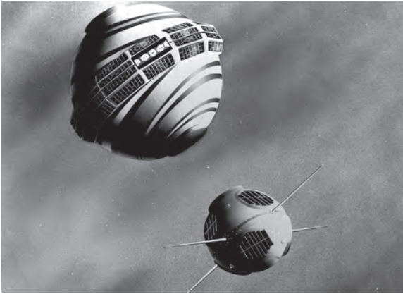
Double First. An artist's drawing depicts the Applied Physics Laboratory's Transit 2A satellite and the Naval Research Laboratory's solar radiation measurement satellite shortly after their planned separation. On June 22, 1960, the two satellites were launched in a piggyback style and then the smaller NRL SOLRAD satellite was released from the Transit satellite by spring force. When this image was publicly released, the GRAB payload inside SOLRAD's shell was highly classified. (NRL photo 60414.jpg)
