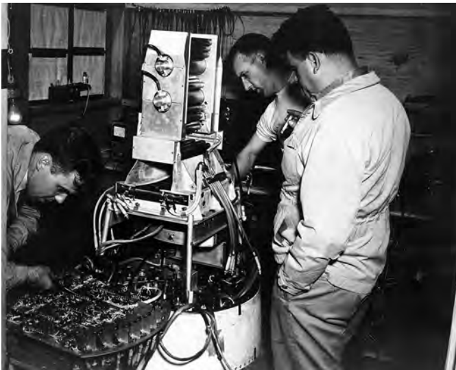
High-Profile Launch. Major media reporters were on hand to watch the launch of Viking 4 from the deck of USS Norton Sound in 1950. NRL engineers are shown adjusting electronic components for timing solar radiation measurements in the scientific “warhead.” (NRL photo P-238)
