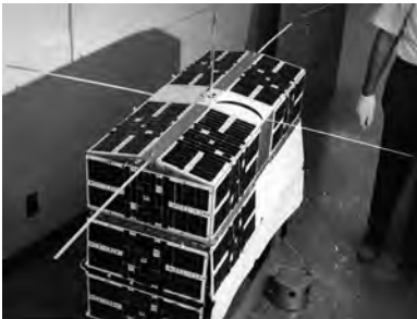
Timation 2. Though not very pretty, the Timation 2 satellite was part of the important process of testing the performance of highly accurate quartz clocks for a space-based navigation system that would become known as GPS. Timation 2 was launched into orbit on September 30, 1969. (NRL photo D-250.jpg)
