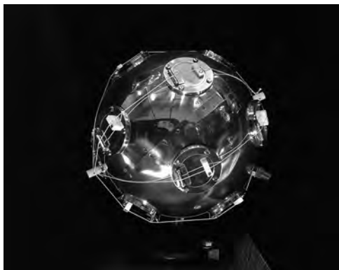
Space Reference. Launched on March 9, 1965, Dodecapole 1 served as a reference target for calibrating the Navy's Space Surveillance System (NAVSPASUR). Once in orbit, a mechanism involving twelve “trap doors” allowed metallic tapes to shoot out and form into 25-foot-long rods about 1/2 inch in diameter, resulting in a space target that was 50 feet across. (NRL photo 77112(14).jpg)
