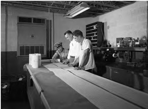
The Lazarus Viking. In a hangar at the White Sands Missile Range in New Mexico, NRL engineers conduct an instrument check on Viking 10. On the first launch attempt on June 20, 1953, the engine exploded, but the rocket was subsequently rebuilt and successfully launched on May 7, 1954. It reached an altitude of 136 miles (217 kilometers). Shown also is the scroll of telemeter data from the flight. (NRL photos 53-061582(22) and 54-061582(17))
