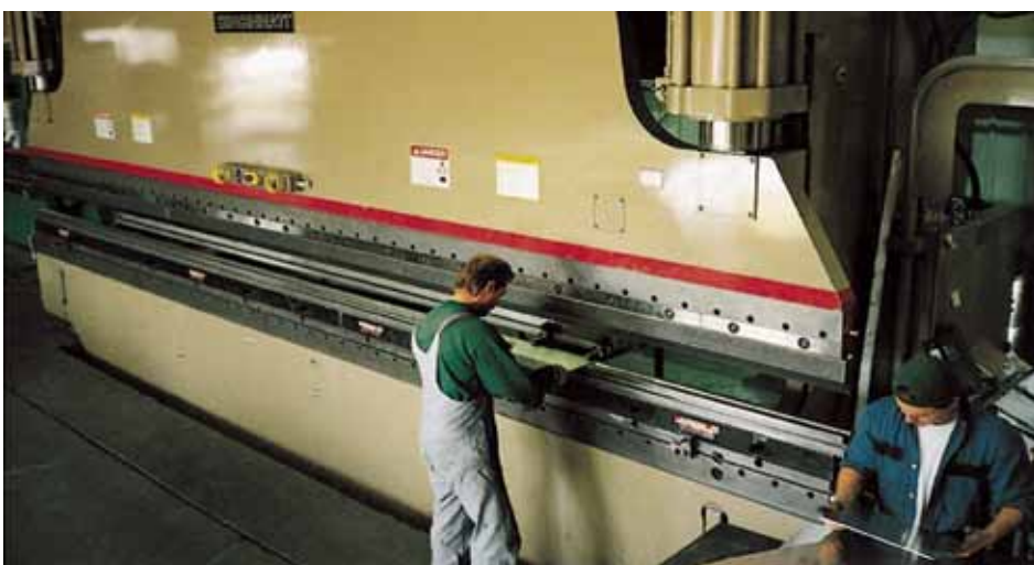
The press brake at Kingfisher is hard at work in Vernon, BC.
