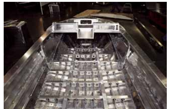
Kingfisher heavy gauge aluminum hulls are built with a hefty grid and stringers, like on this 1775 Extreme Series Model.
