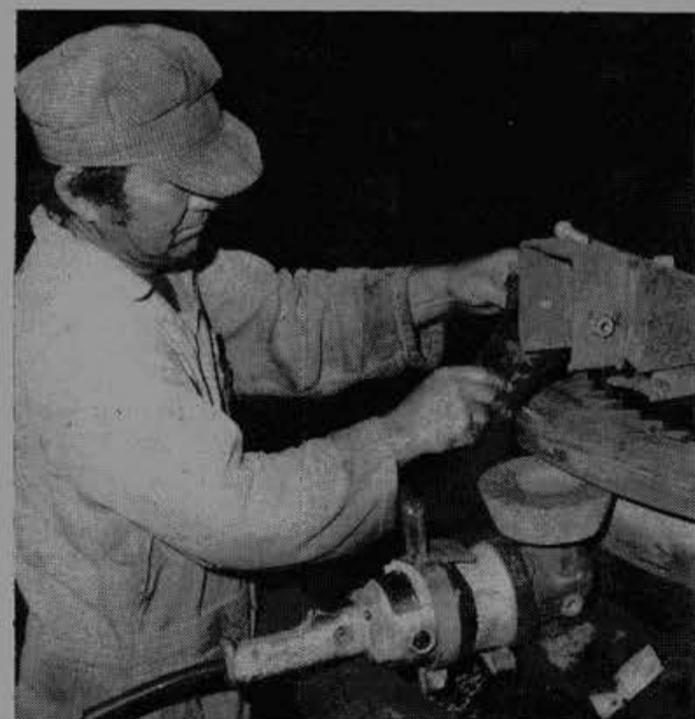
Takaesu smooths out surface after welding (above) and welds warped areas (left).
