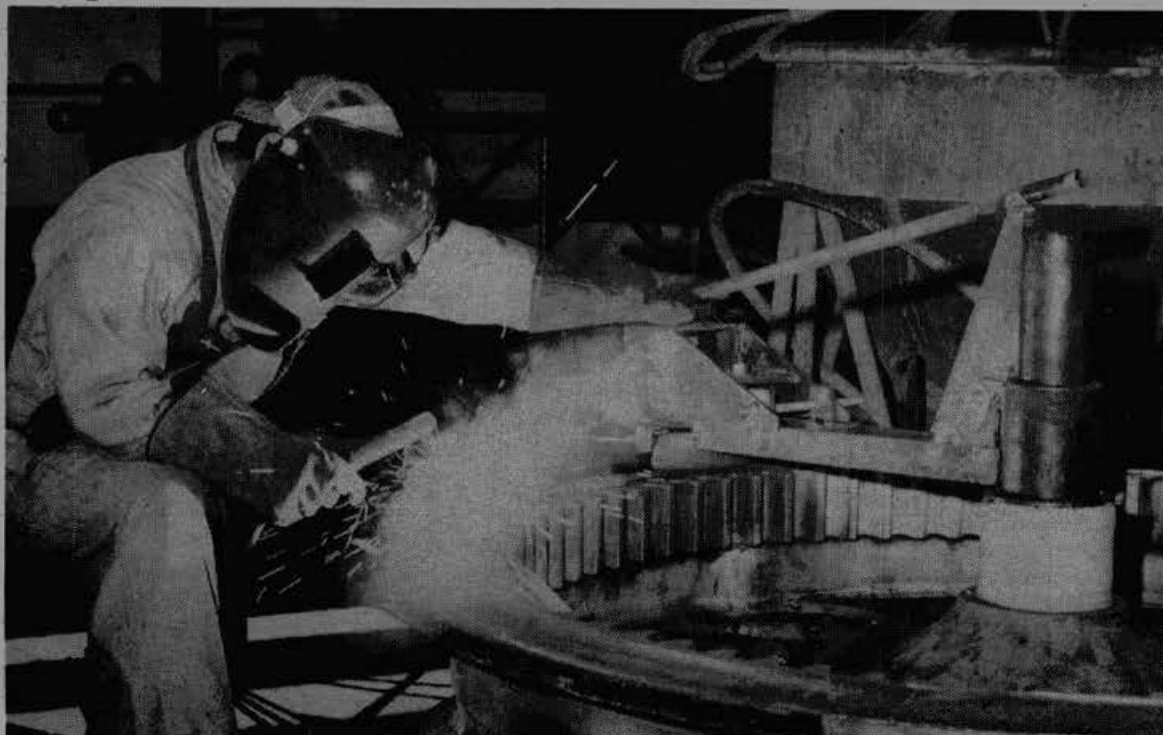
Takaesu smooths out surface after welding (above) and welds warped areas (left).
