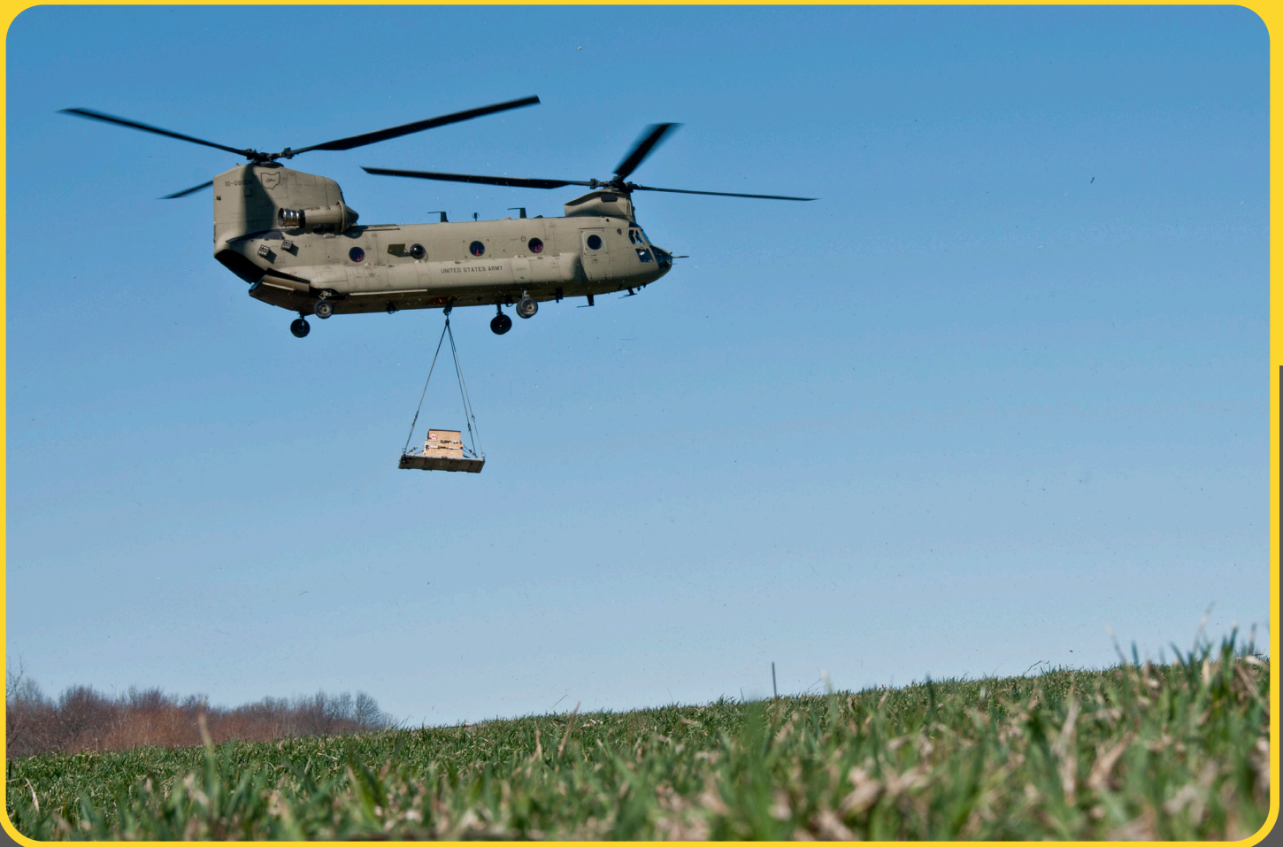
A CH-47 Chinook from the Ohio Army National Guard's Company B, 3rd Battalion, 238th Aviation Regiment, located in North Canton, Ohio, performed a sling load of a heavy drop pallet in a muddy drop zone at the 179th Airlift Wing, Mansfield, Ohio, March 18, 2016.
