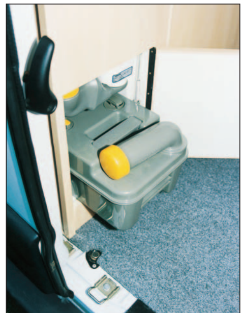
Removal of the cassette was accomplished through an access door in the aisle wall of the shower room.
