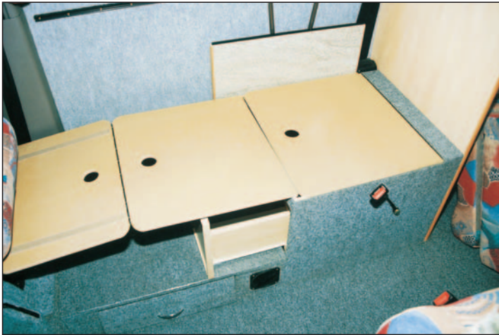
Bed making required neither effort nor agility. Just open the underseat drawer, hinge over the baseboard, and open it out to meet the front seat. Then fold flat the backrest board.
