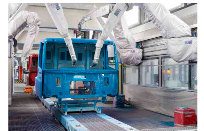
Robots paint cabs in the new state-of-the-art Cab Paint Facility at the DAF premises in Westerlo, Belgium.
