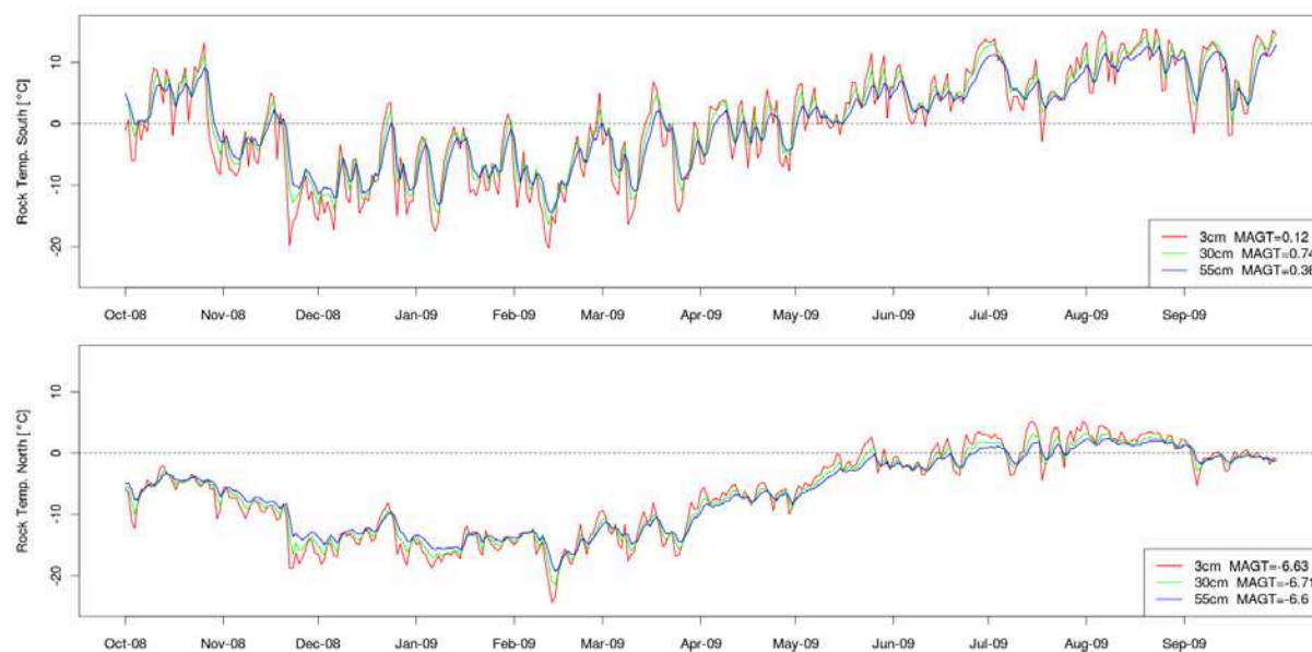
Fig. 5 – Mean daily rock temperature on the south and north faces of the Piton Central for the hydrological year 2008-09 at three different depths below the surface.
