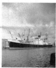
The "CAIRNDHU" was built in 1952 by Wm. Gray & Co. Ltd. of Hartlepool. Gross Tonnage 7503.27 Net Tonnage 4631.12 Shaft Horse Power 4650 Net Horse Power 831
