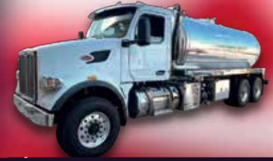
2024 PETERBILT 567 , CUMMINS ISX 450 HP, ALLISON AUTOMATIC TRANSMISSION, 4200 ALUMINUM TANK, NVE 4310 BLOWER 940 CFM, 36" TOOLBOX, CHROME PACKAGE. CALL FOR PRICE
