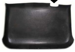
Headliner comes with wiper control location marked for cutout during installation
