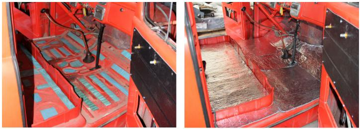
Typical Floor Panel Sound Damping and Thermal Barrier Insulation.
