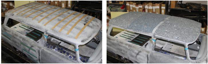
Typical Roof Panel Sound Damping and Thermal Barrier Insulation.
