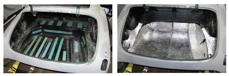
Typical Trunk Floor Sound Damping and Thermal Barrier Insulation.
