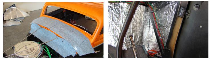
Typical Cowl Panel Sound Damping and Thermal Barrier Insulation.
