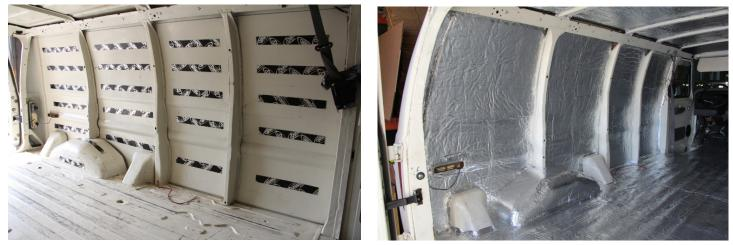
Typical Body Panel Sound Damping and Thermal Barrier Insulation.
