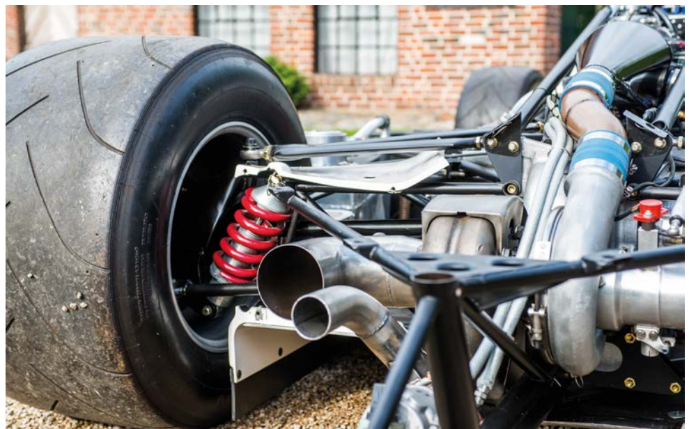
Rear bodywork of the car was so low that the upper suspension wishbones actually ran above it
