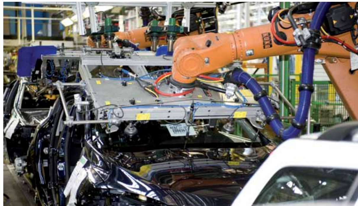
Fitting windscreens on Mégane 3 at the Palencia site.
