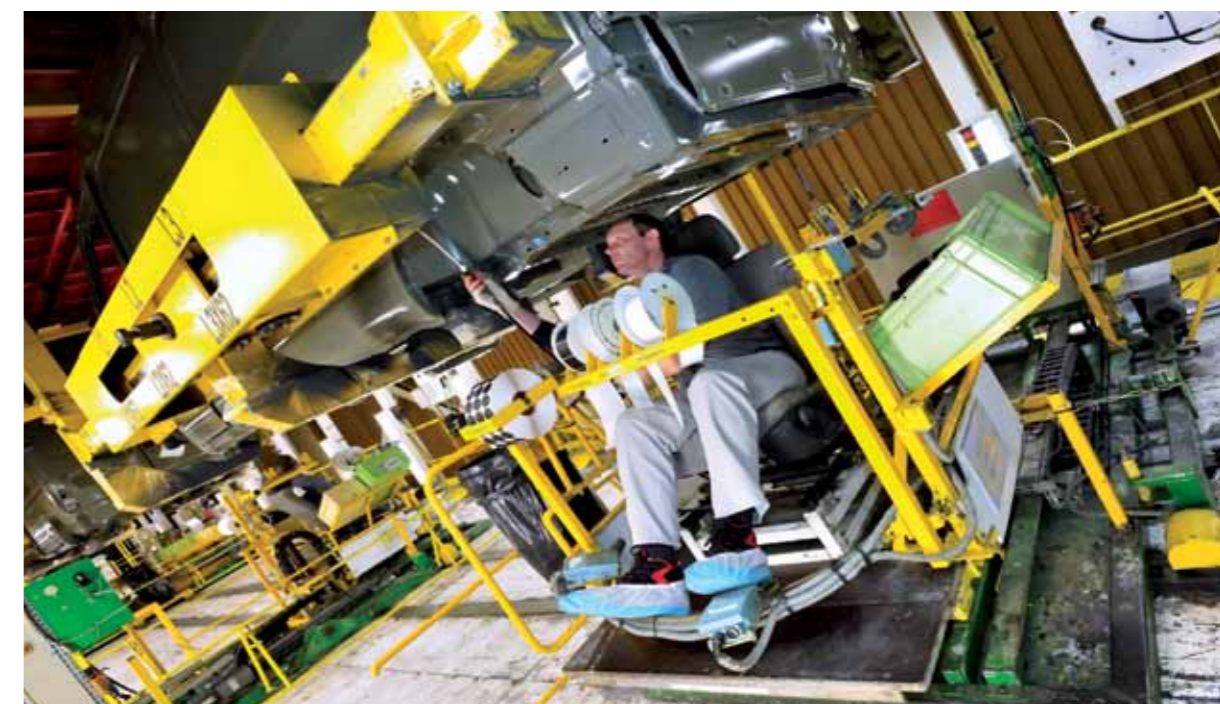
Sovab Batilly - Mastics workshop- underbody tool trolley for person of reduced mobility. Pedal or joystick control.
