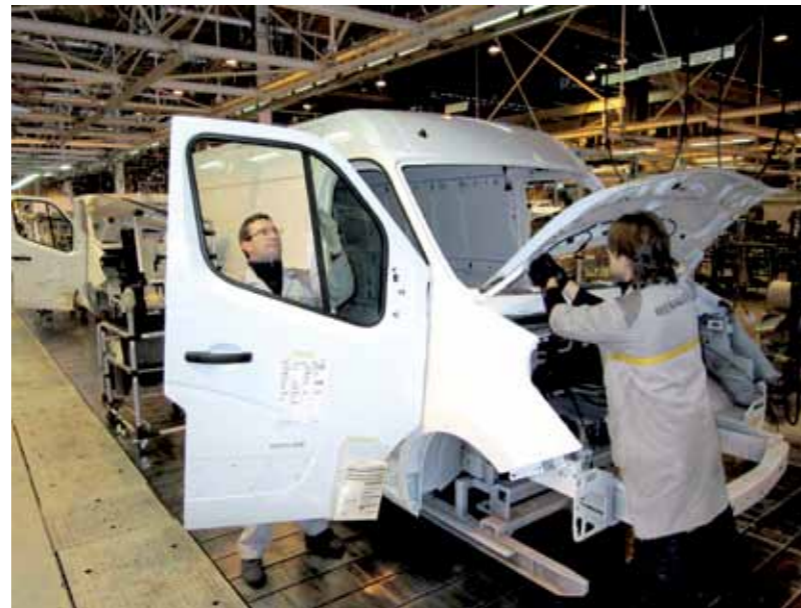
Batilly plant: Fitting trim parts on new Master.
