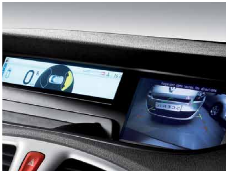
To make parking maneuvers easier and safer, the reversing camera projects a picture of the area behind the car onto the navigation screen.
