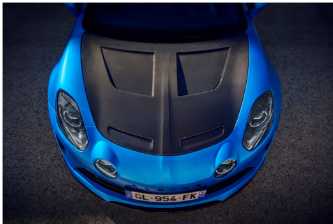
Entirely made of carbon fiber, the bonnet of the A110 R loses 2.9 kg. The two air ducts optimize the aerodynamics of the sports car.
