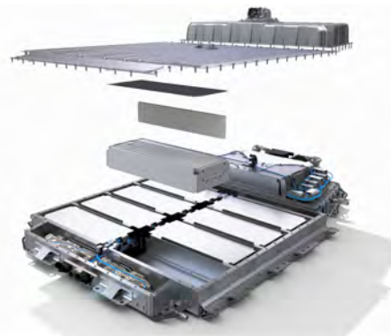
An ultra-thin battery of only 110 mm.
