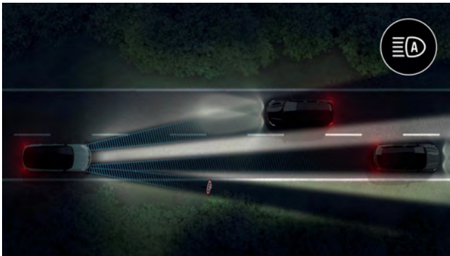
Matrix LED Vision technology adapts the distribution of light to ensure the comfort and safety of the driver and occupants of surrounding vehicles.
