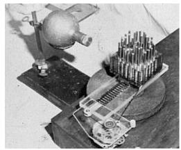
Figure 16.8. The prototype for the CT scanner
