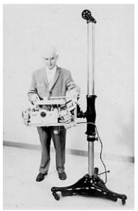
Figure 6.8. Benedict Cassen and the first radionuclide scanner
