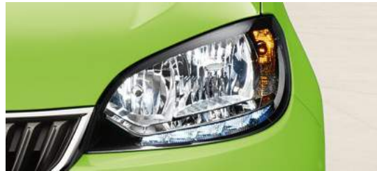
HALOGEN TWIN HEADLIGHTS WITH SEPARATE LED DAYTIME RUNNING LIGHTS
