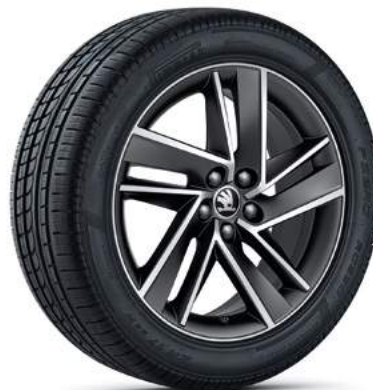
Blade 5JA 071 497G ZG6 light-alloy wheel 7.0J × 17" for 215/40 R17 tyres ET46 black matt brushed ŠKODA Genuine Accessories
