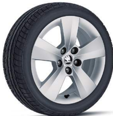
Matone 6V0 071 495A 8Z8 light-alloy wheel 6.0J × 15" for 185/60 R15 tyres ET38 silver metallic ŠKODA Genuine Accessories
