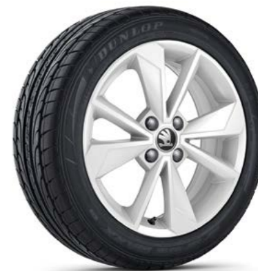
Scorpius 1ST 071 496K FM9 Light-alloy wheel 6,0J x 16" for 185/50 R16 tyres in white design
