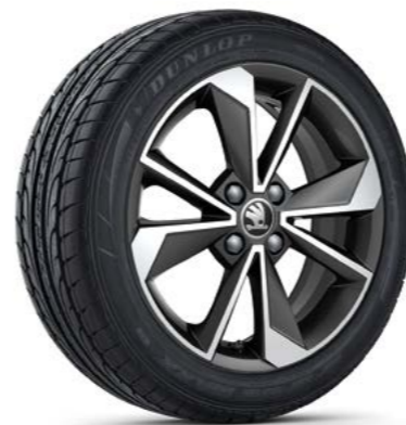
Scorpius 1ST 071 496J FL8 Light-alloy wheel 6,0J x 16" for 185/50 R16 tyres in black metallic design, brushed
