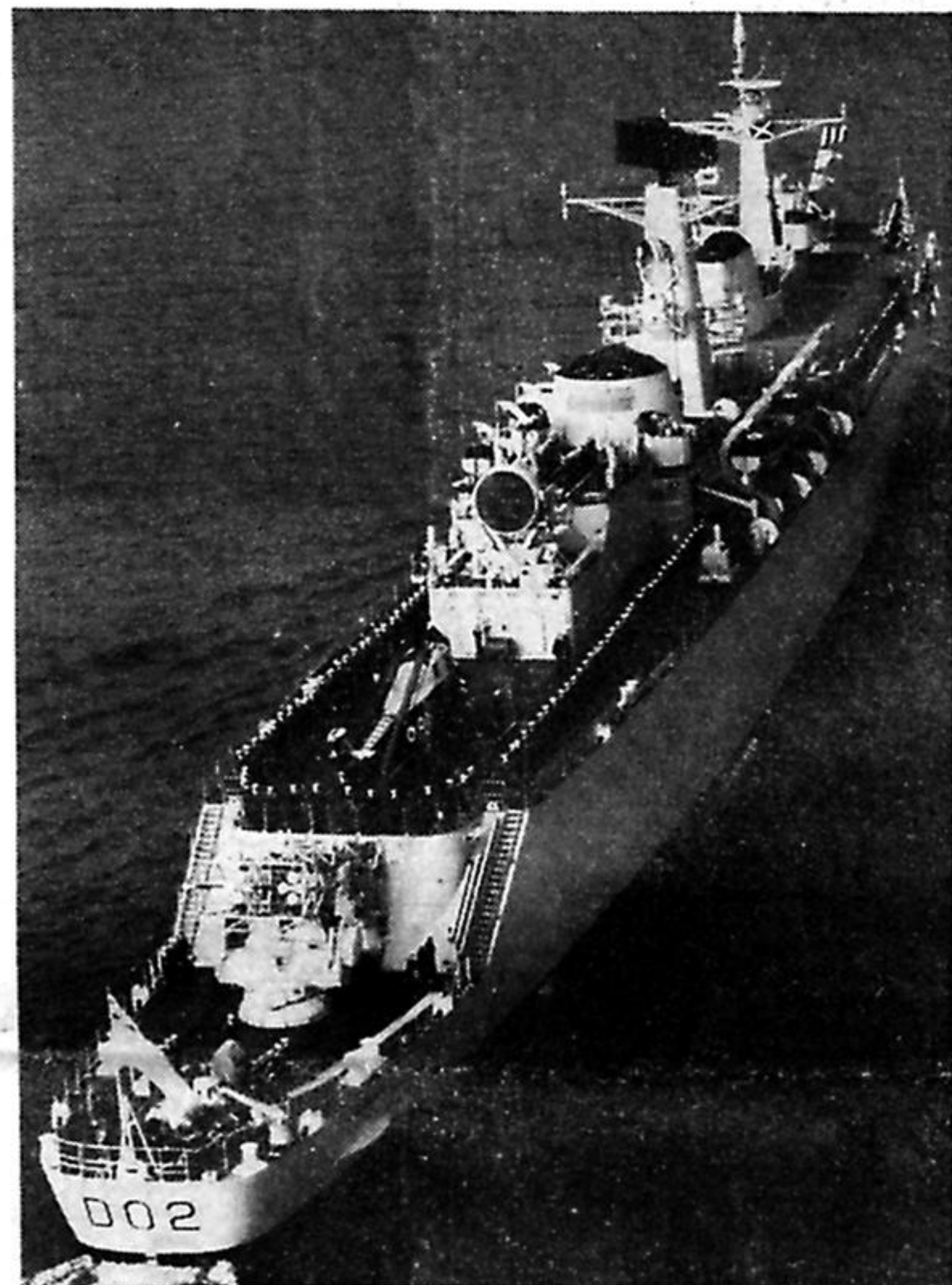
H.M.S. Devonshire, first of the six County Class guided-missile destroyers (6,200 tons, full load). Hampshire, Kent and London are expected to join the Fleet this year and good progress is being made with the other two, H.M.S. Fife and H.M.S. Glamorgan. These two ships will carry the Seaslug Mark II—later to be fitted to the other four. At the moment they are fitted with Seaslug Mark I medium-range ship-to-air guided missiles. Short-range anti-aircraft missiles (Seacat) are also part of the armament of these powerful ships.
