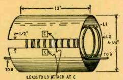
Fig. 5—The output coil is sheet copper.
