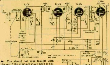
the set if the diagram given here is followed. All condensers are rated at 200 volts, and the resistors may be 1/2-watt size unless otherwise specified. Multiband operation is possible by connecting a band-change switch at points S on the diagram. Standard coil assemblies can be used on broadcast and short-wave bands. These should be standard coils
