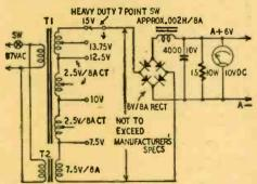
Fig. 3-A power supply for low-voltage use.
