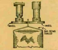
sticky. When the material is not thermoplastic, it is necessary to add a strip of film of thermoplastic substance between the sides of the bag. Again heat causes it to become sticky sealing the bag. The wheels and shafts should be of good heat-
