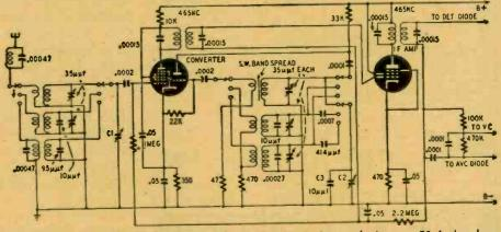
Fig. 4-The simple r.f. end of the Murphy A-104. Its tuning scale is over 50 inches long.
