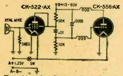
The wrist-watch radio transmitter schematic. staff to build radio transmitters actually down to the size of a lipstick case (minus batteries and microphone).
