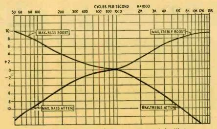
Fig. 1—Amplifier response under maximum tone control settings.
