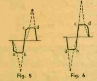
setting frequency changes from normal due to metal fatigue and loss of temper in the vibrating reed, are easily seen. Use only one complete cycle of the vibrator for comparison on the 'scope screen.
