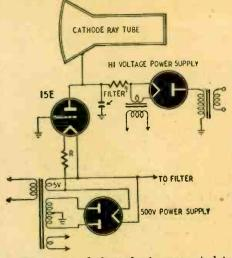
The plate of the tube is connected to the high-voltage power supply, but draws no current because the tube is cut off by the high bias voltage. As soon as the power is turned off, the bias voltage drops rapidly to below cutoff before the 15E filament has cooled off appreciably. The tube then conducts and quickly discharges the high-voltage condenser through the low-voltage bleeder.
