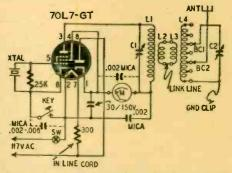
Schematic of the I-tube a.c.-d.c. transmitter. Two additional capacitors are suggested.
