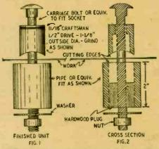
The die for the cutter is made of a piece of thick-wall pipe cut off square. It should fit snugly around cutter but not bind, if the hole is to be a clean one. Force a hardwood cylinder halfway into the pipe and drill it accurately through the center for a snug, sliding fit for the bolt.
