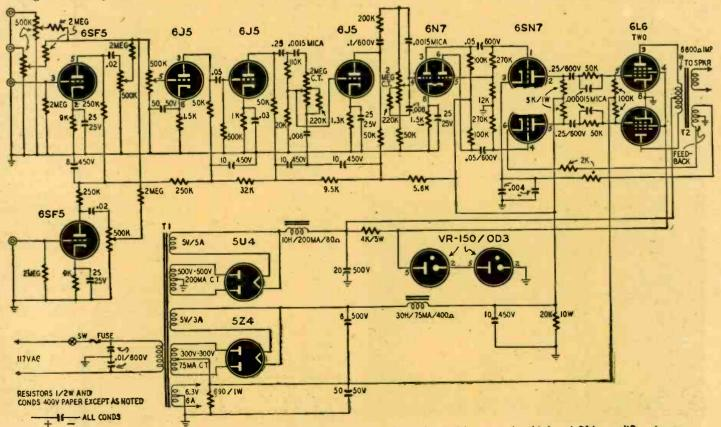
Fig. 2—The circuit of the amplifier. The bass and treble tone controls are located between the third and fifth amplifier stages. RADIO-CRAFT for APRIL, 1948
