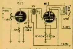
A power supply delivering about 200 ma is adequate for this amplifier.
