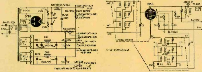
Fig. I-Line-operated power pack for BC-654-A or similar receivers. 36
