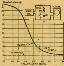
Fig. 2—Operation of the bass-boost circuit.
