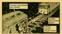
How the proposed radar system will operate.
