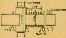
My original coil forms had 7 sections, but the coils will be flatter and neater if a larger number of sections are cut, at least 11 or 13. The forms must be cut with an odd number of sections.
