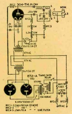
Fig. 4—A 1-kw r.f. induction heater.
