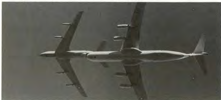
By far the primary cause of C-135 mishaps in 1983 was air refueling. Tankers are still experiencing abrupt pitch changes while the receiver is in the contact position.
